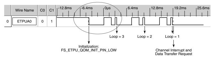
Figure 8. qom\_example1.c QOM0 (ETPUA0) Output
