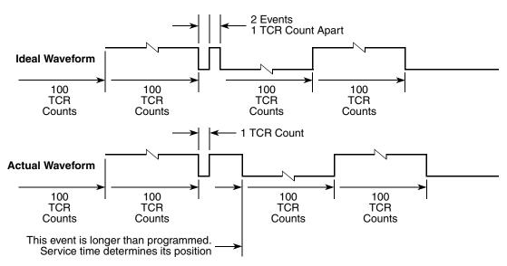
Figure 6. Real v. Ideal Waveforms
