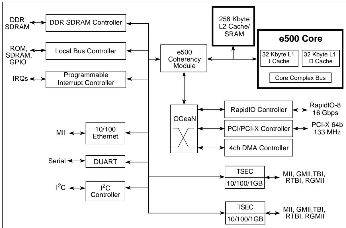
Figure 1. MPC8540 Functional Block Diagram
