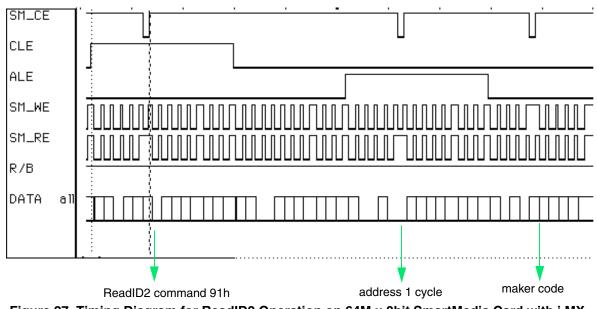
Figure 27. Timing Diagram for ReadID2 Operation on 64M x 8bit SmartMedia Card with i.MX
