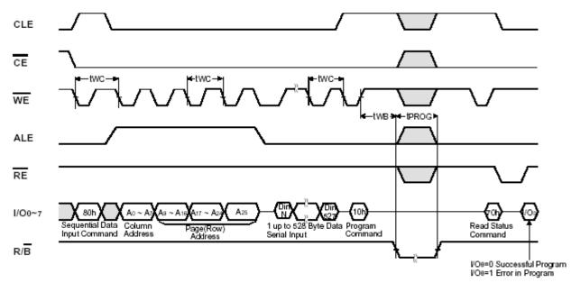
Figure 10. Timing Diagram of Page Write Operation
