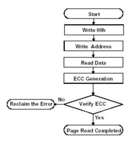
Figure 17. Flow Chart for Page Read Operation
