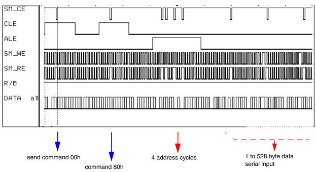
Figure 22. Timing Diagram for Page Program Operation on SmartMedia Card with i.MX
