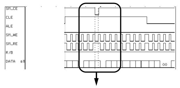
Figure 18. Timing Diagram During CLE Cycle
