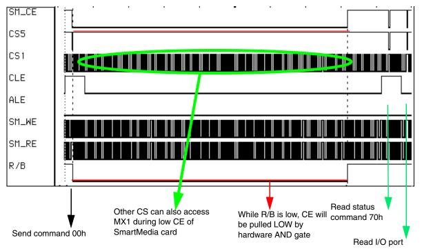
Figure 23. Page-Programming on SmartMedia Card with i.MX
