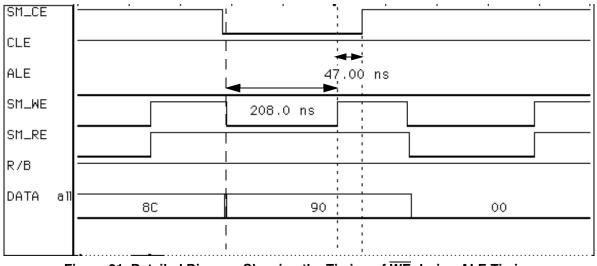
Figure 21. Detailed Diagram Showing the Timing of WE during ALE Timing
