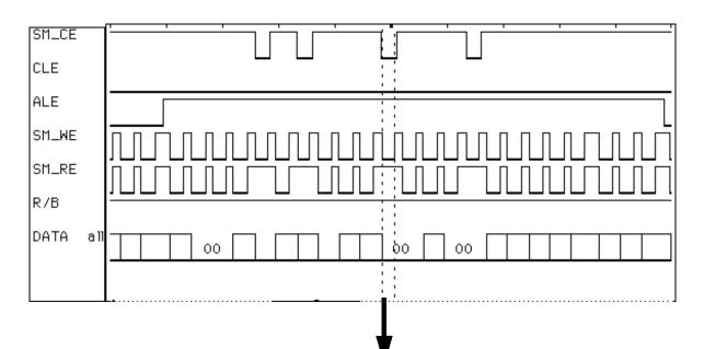
Figure 20. Timing Diagram of ALE Cycle
