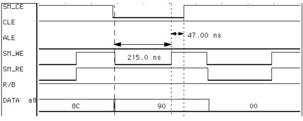
Figure 19. Detailed Timing Diagram of WE During CLE Cycle
