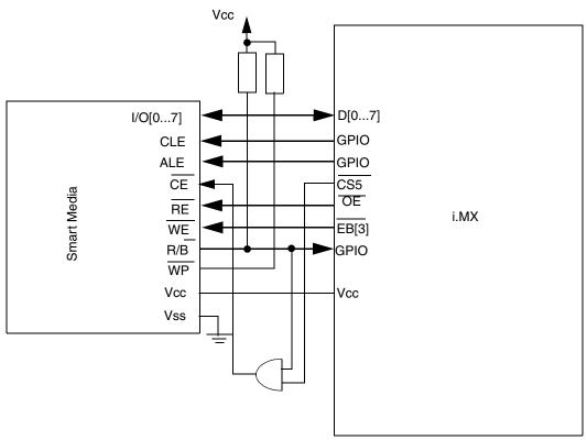
Figure 3. SmartMedia Card Interface with i.MX
