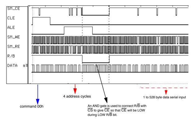
Figure 24. Timing Diagram for Read Operation in 64M x 8 bit SmartMedia Card
