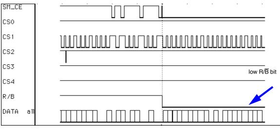
Figure 25. Access of Other Chip-Select (CS) of i.MX during Low R/B bit of SmartMedia Card
