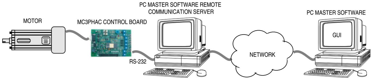
**Figure 4. Connecting Motorola Microcontrollers to the Internet**
