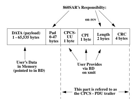
Pad - pad may be needed if the PDU is not a multiple of 48 bytes.
