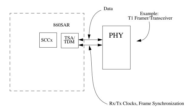
The MPC860SAR supports aggregate Tx/Rx rates of 60 Mb/s for the UTOPIA interface and 20 Mb/s for the serial interface.
