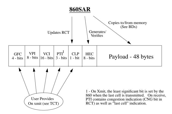
\*A switch routes cells using VPI/VCI via a lookup table. An entire VP can be switched.
