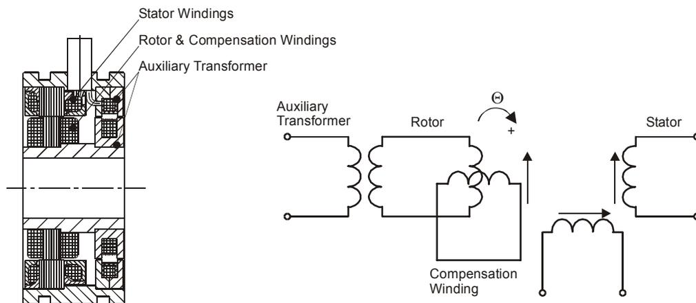
**Figure 3-1. Block Scheme of the Hollow Shaft Resolver**
