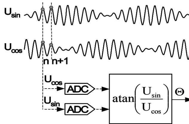
**Figure 3-5. Angle Extraction Using the Inverse Tangent Method**
