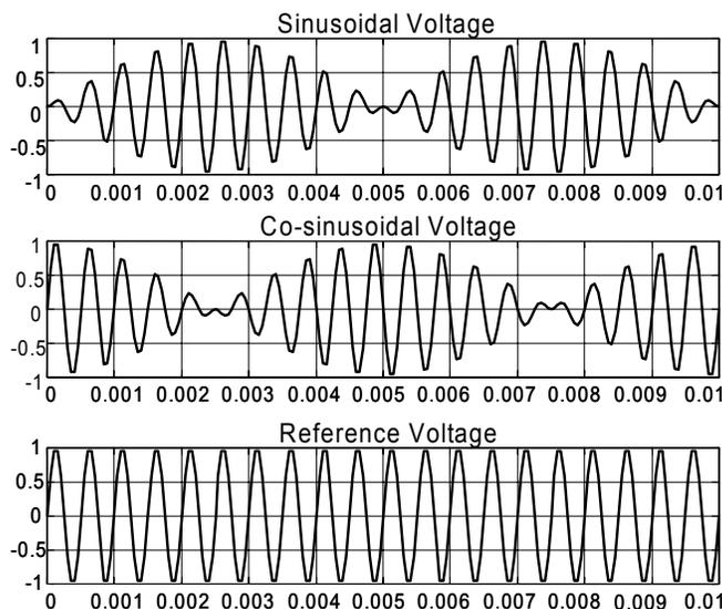
**Figure 3-4. Excitation and Output Signal of the Resolver**
