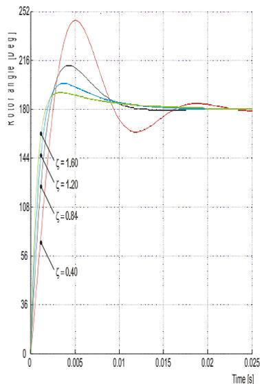
**Figure 3-9. Dynamic Responses of the Rotor Angle Estimations -**
