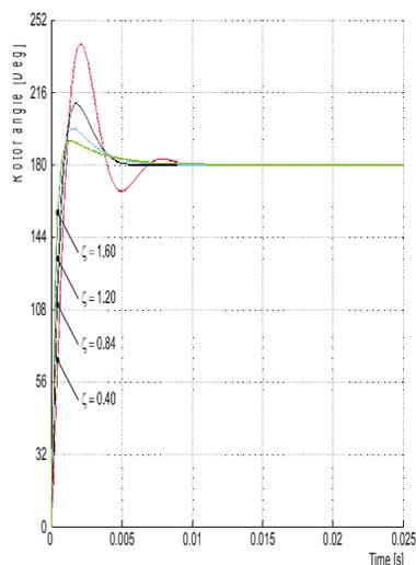
**Figure 3-10. Dynamic Responses of the Rotor Angle Estimations -**
