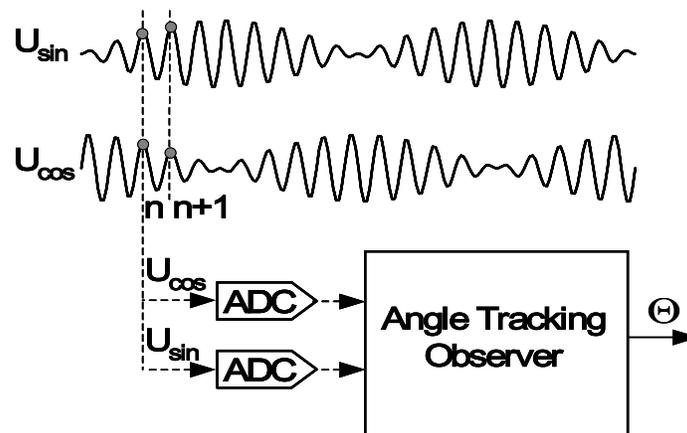
**Figure 3-6. Angle Extraction Using the Angle Tracking Observer**
