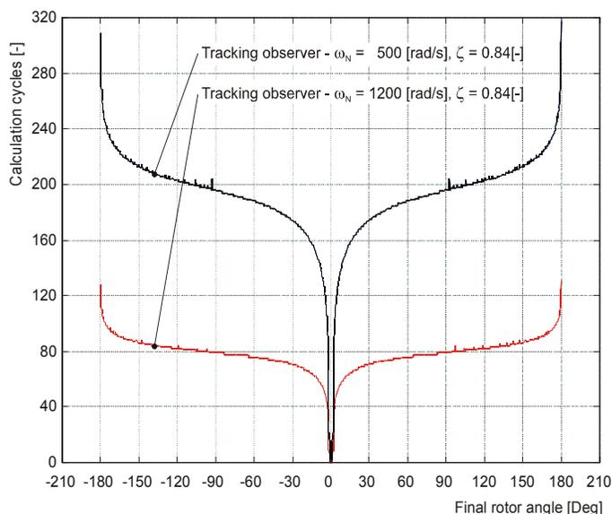
**Figure 5-3. Settling Time of the Angle Tracking Observer**
