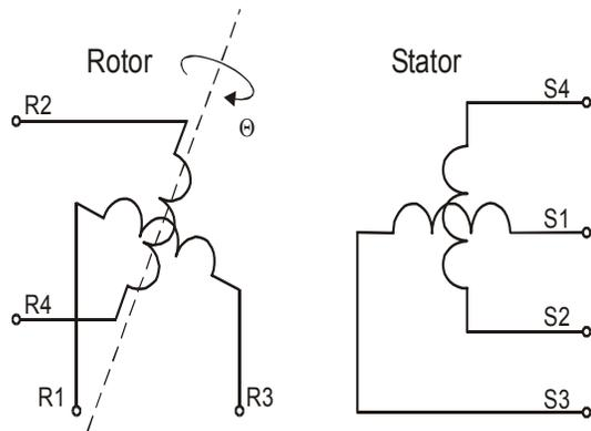
**Figure 3-2. Block Scheme of the Resolver**
