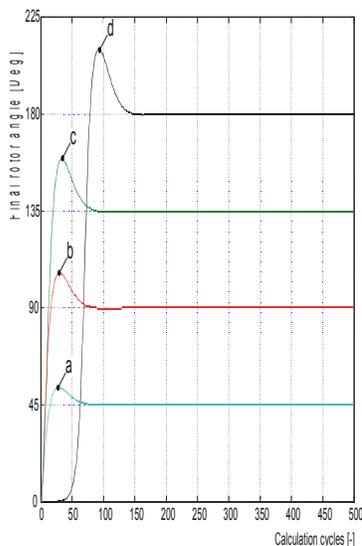
**Figure 5-2. Responses of the Estimated Angle of the Angle Tracking Observer -**
