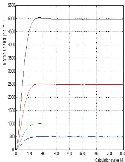
**Figure 5-5. Transient Response of Rotor Speed Estimations -**
