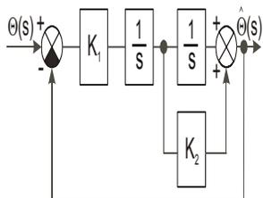
**Figure 3-8. Simplified Block Scheme of the Angle Tracking Observer**
