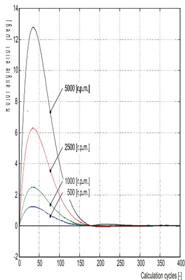
**Figure 5-6. Transient Response of Rotor Angle Estimation Error -**
