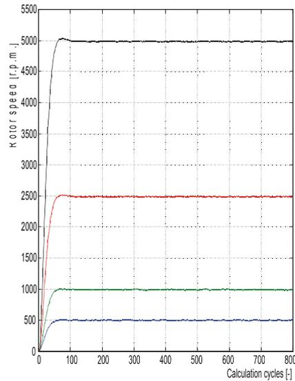
**Figure 5-7. Transient Response of Rotor Speed Estimations -**
