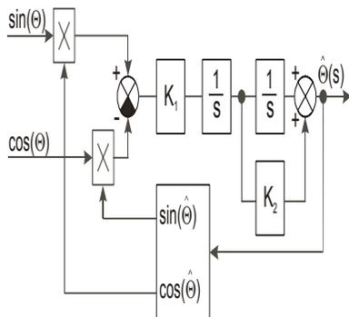
**Figure 3-7. Block Scheme of the Angle Tracking Observer**
