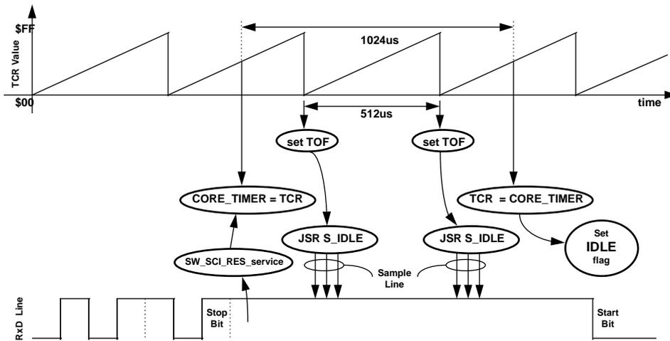
Figure 6-3. Relationship Between Data Line, Core Timer and S\_IDLE Routines
