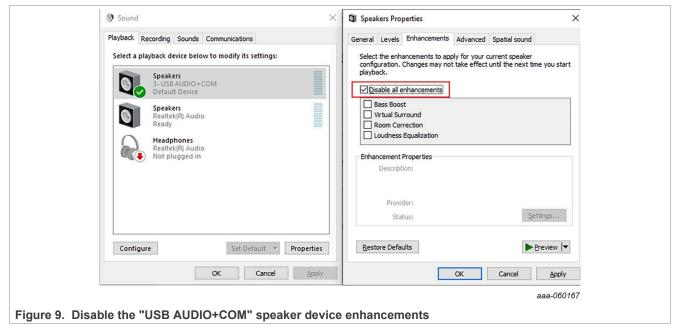
Then the user can open a COM window, launch the recording APP, and start recording the up-streaming filtered audio. To select the filter, up-streaming and recording, type "a"/"A" and "0"~"7" in the COM window. For more details, see <a href="Section 7.2">Section 7.2</a>. To analyze and evaluate the filter and the filtered signal quality, watch the recorded signal, both in time and frequency domains.
