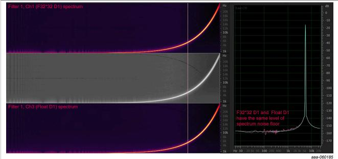
Figure 21. 3000 Hz LPF - F32\*32 D1 and float D1 has the same level of noise
