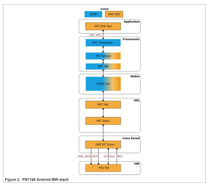
Figure 2 shows the architecture of the PN7160 Android NFC stack.
