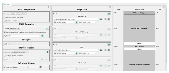
Include the application binary and specify the Boot Target and Type, the Export BLOB Image to create a bootable flash image containing both the start-up self-test and user application.
