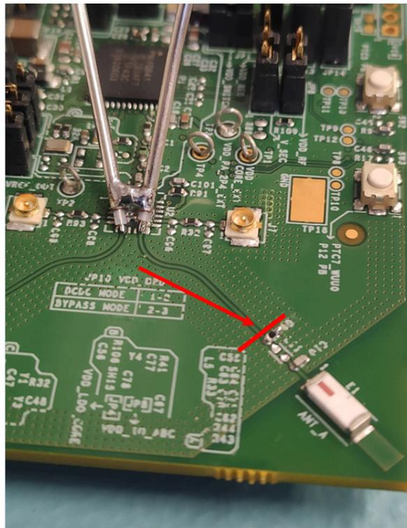
Figure 2. VNA calibration plane moved to the antenna PI filter
