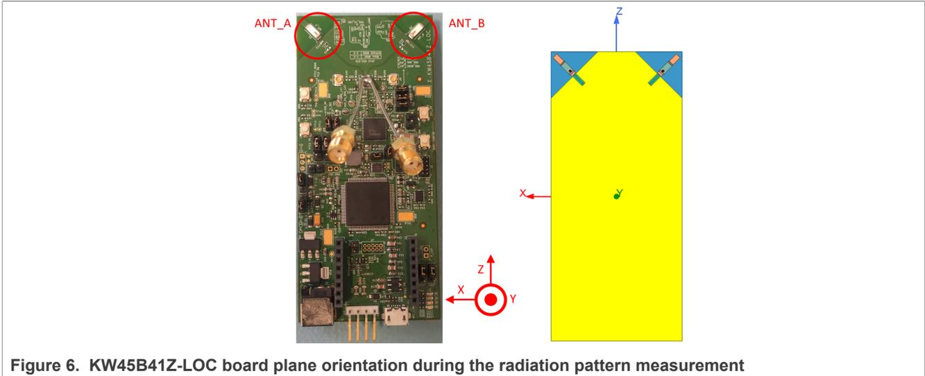
Figure 6. KW45B41Z-LOC board plane orientation during the radiation pattern measurement
