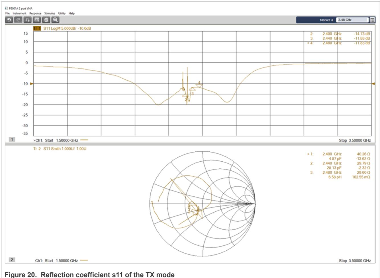
Figure 20. Reflection coefficient s11 of the TX mode
