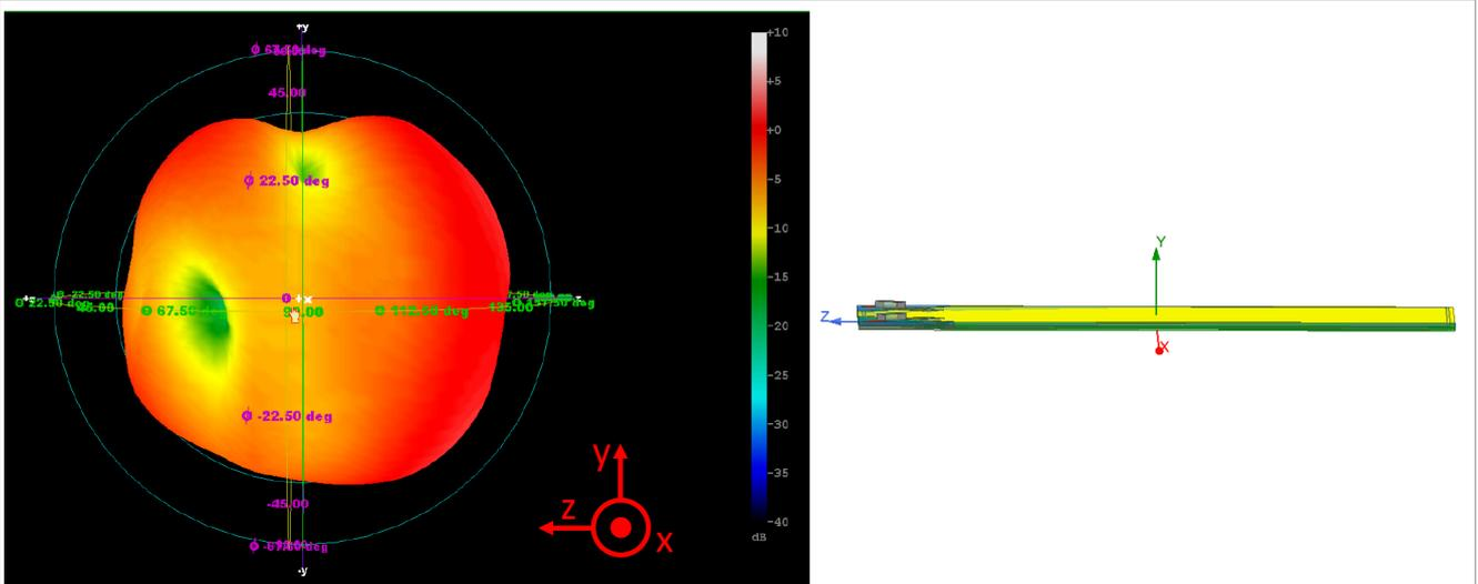
Figure 7. ANT\_A 3D radiation pattern
