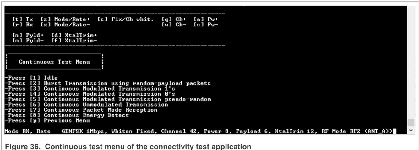
Figure 36. Continuous test menu of the connectivity test application
