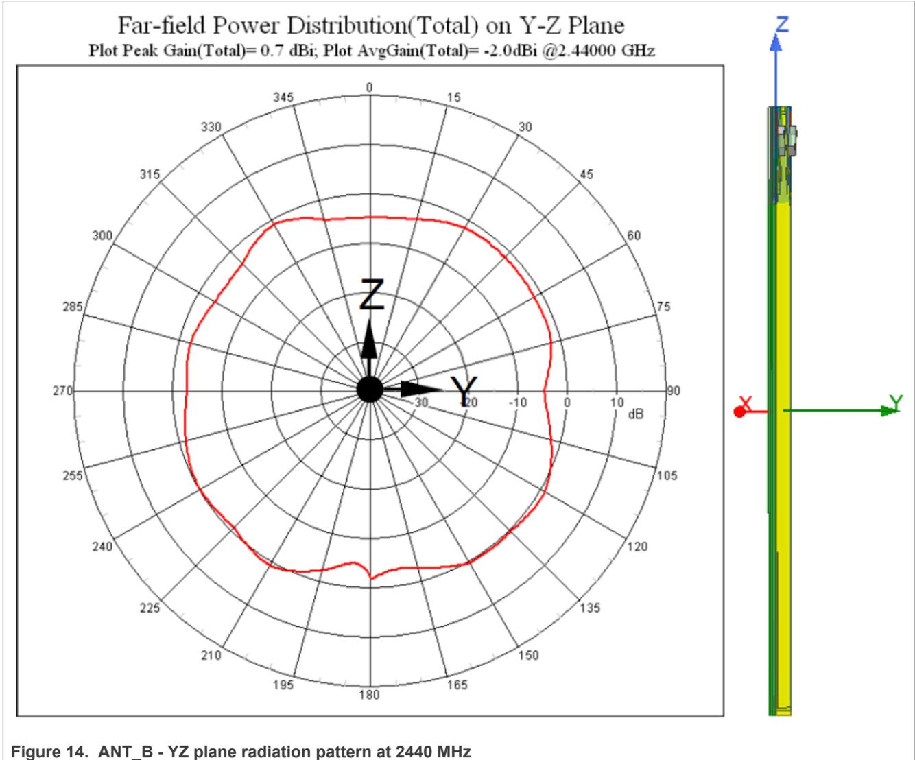
Figure 14. ANT\_B - YZ plane radiation pattern at 2440 MHz
