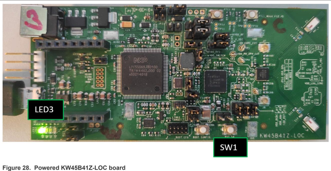
Figure 28. Powered KW45B41Z-LOC board
