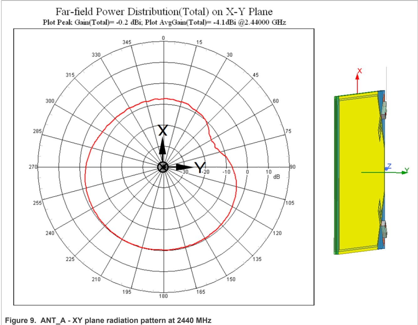
Figure 9. ANT\_A - XY plane radiation pattern at 2440 MHz
