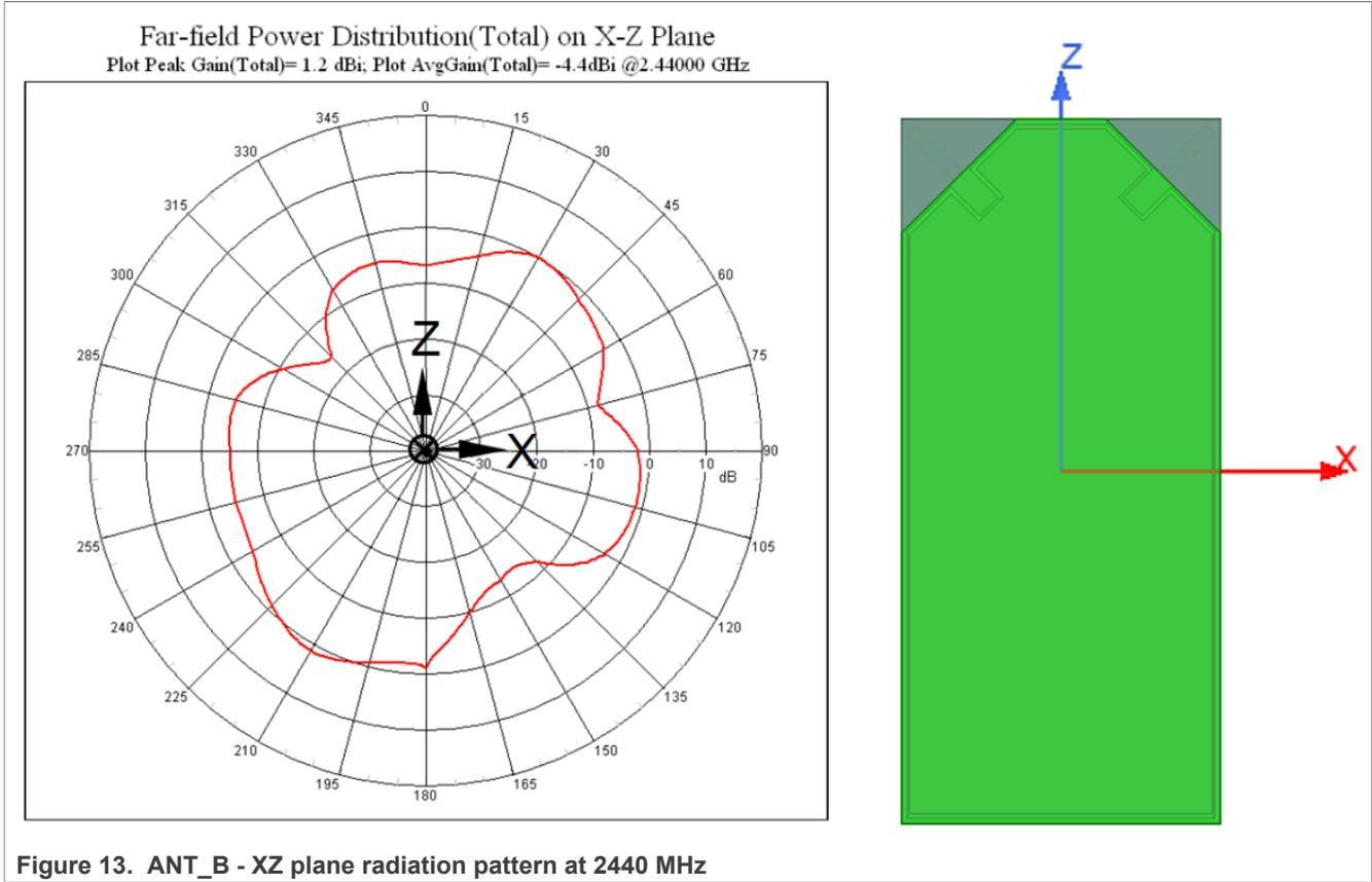
Figure 13. ANT\_B - XZ plane radiation pattern at 2440 MHz
