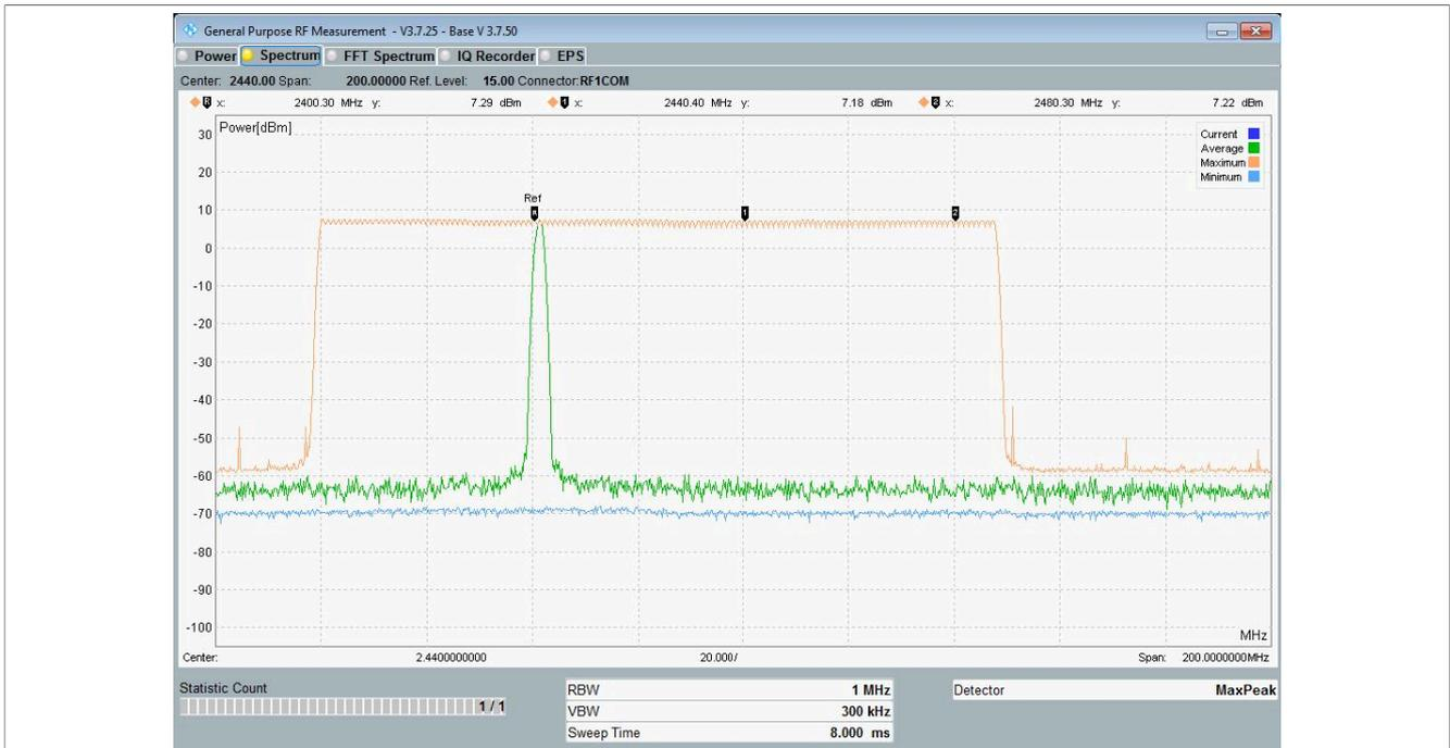
Figure 25. Frequency spectrum captured during maximum TX output level measurement
