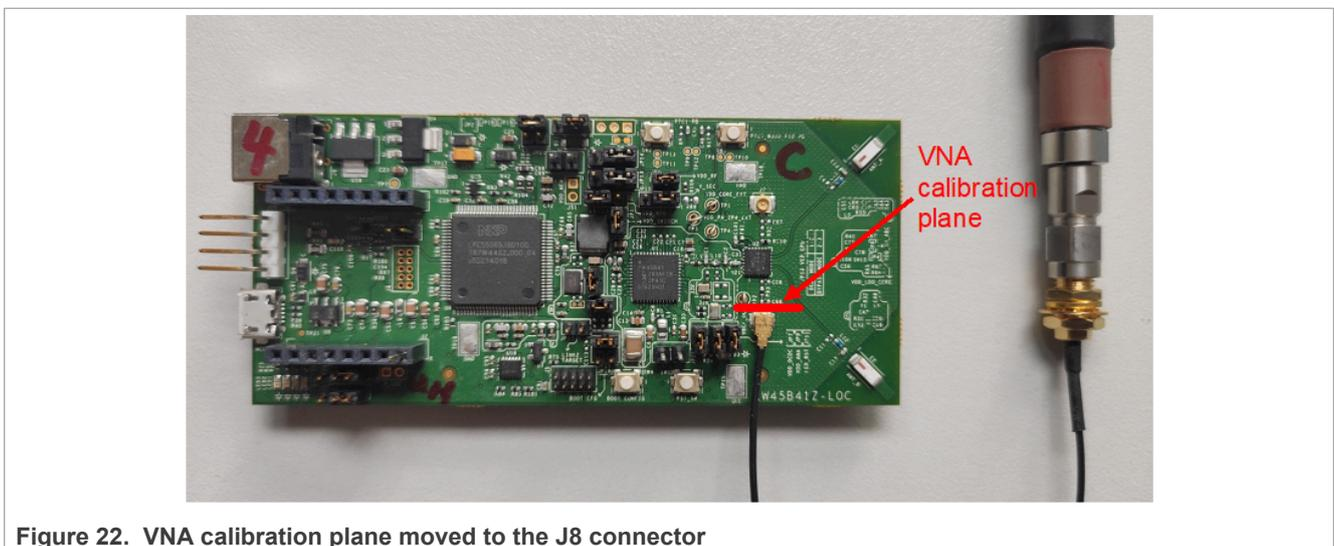
Figure 22. VNA calibration plane moved to the J8 connector
