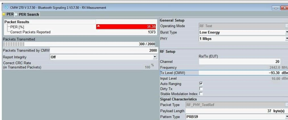
Figure 27. Sensitivity measurement of KW45B41Z-LOC board for BLE data rate of 1 Mbit/s on channel 20
