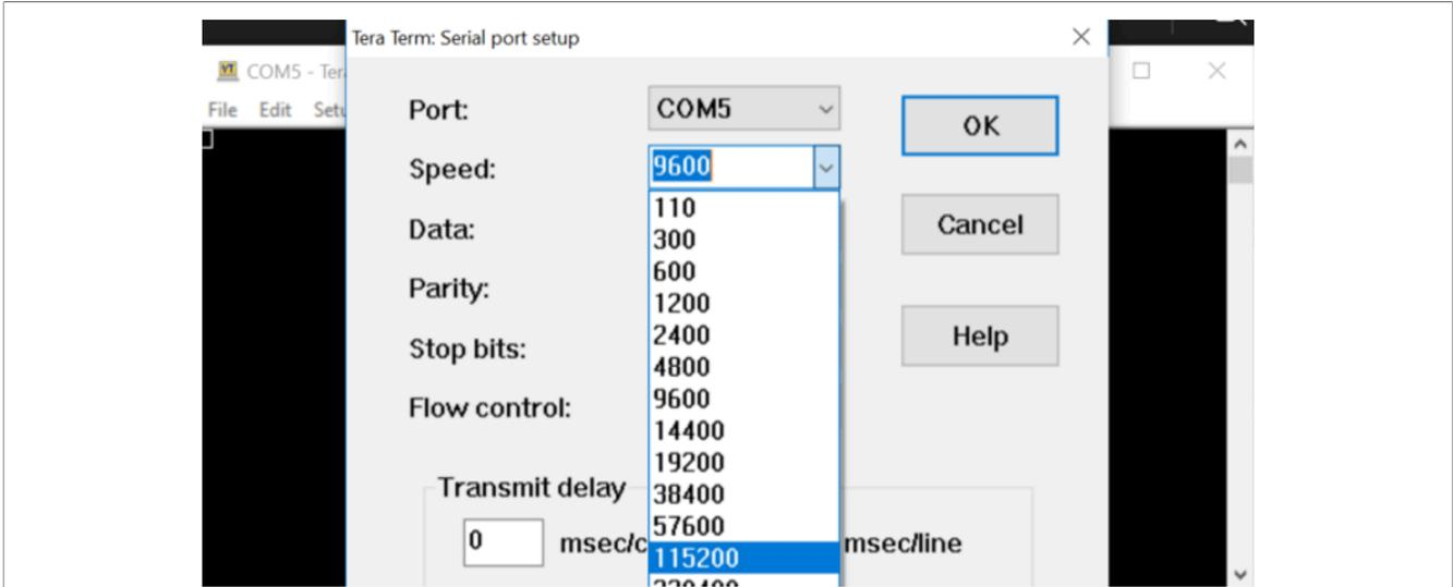
Figure 32. Teraterm Serial COM port settings
