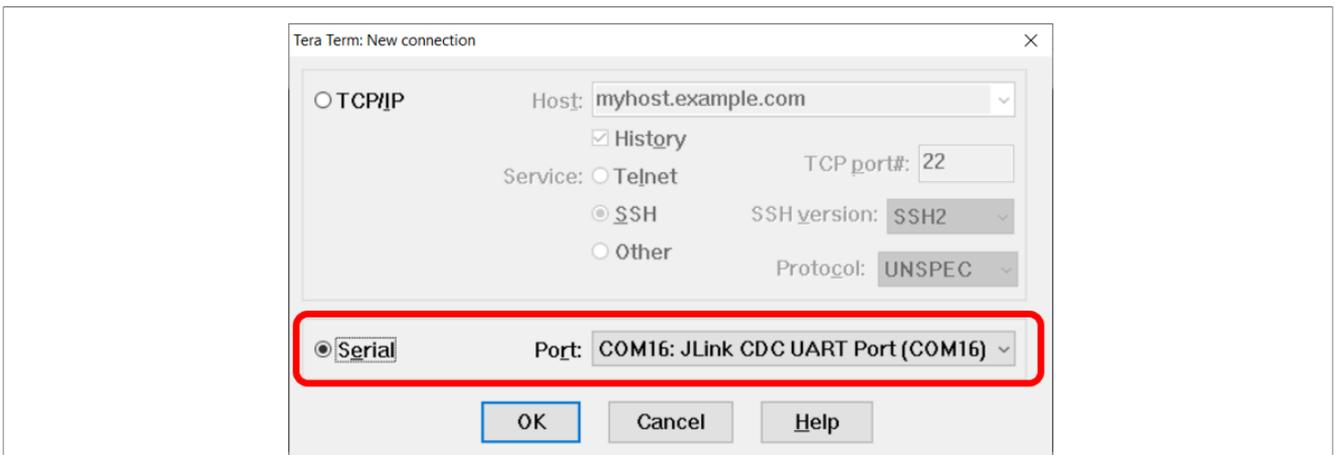
Figure 31. Teraterm Serial port setup selection
