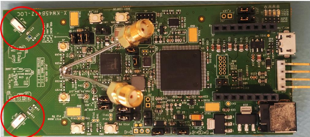
Figure 1. KW45B41Z-LOC board with semirigid cables soldered for antenna reflection coefficient measurement
