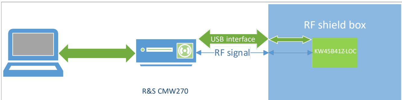
Figure 26. RF sensitivity measurement – block diagram
