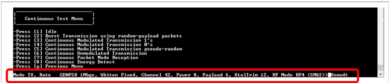
Figure 38. Continuous unmodulated transmission
