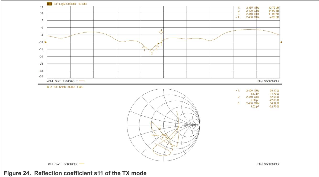
Figure 24. Reflection coefficient s11 of the TX mode
