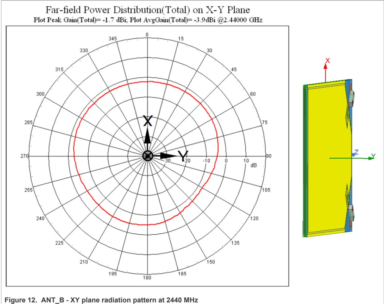
Table 8. ANT\_B - XY plane radiation pattern at 2440 MHz
