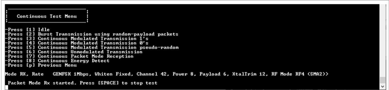
Figure 37. Continuous packet receive mode
