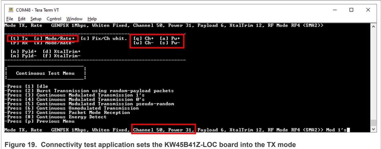
Figure 19. Connectivity test application sets the KW45B41Z-LOC board into the TX mode
