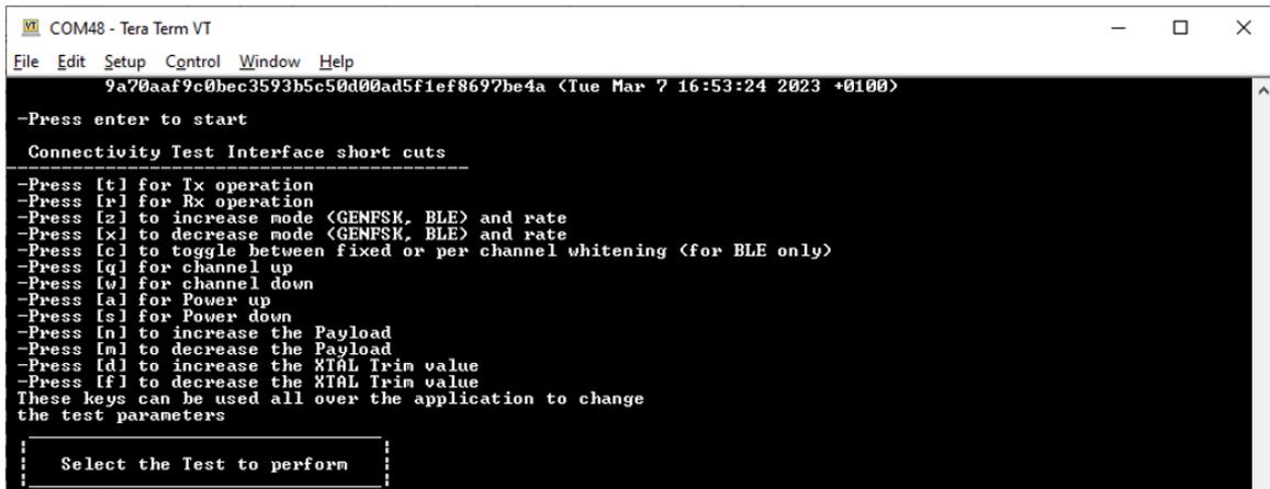
Figure 39. Connectivity test interface shortcuts menu
