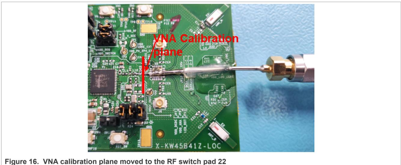
Figure 16. VNA calibration plane moved to the RF switch pad 22
