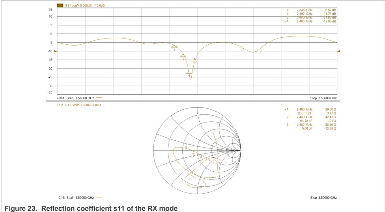
Figure 23. Reflection coefficient s11 of the RX mode
