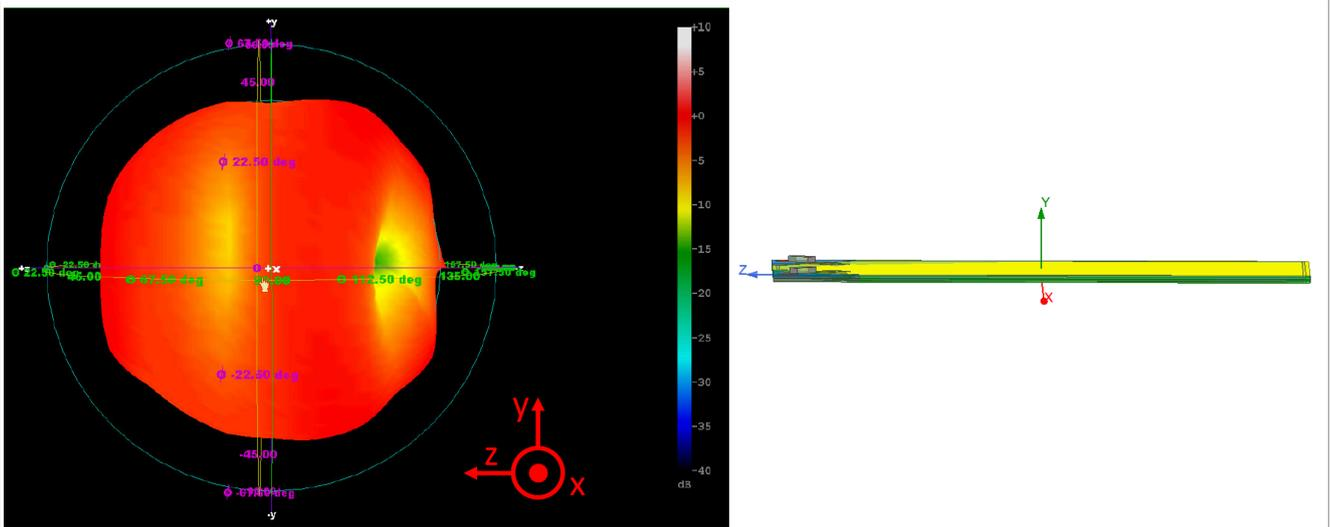
Figure 8. The ANT\_B 3D radiation pattern
