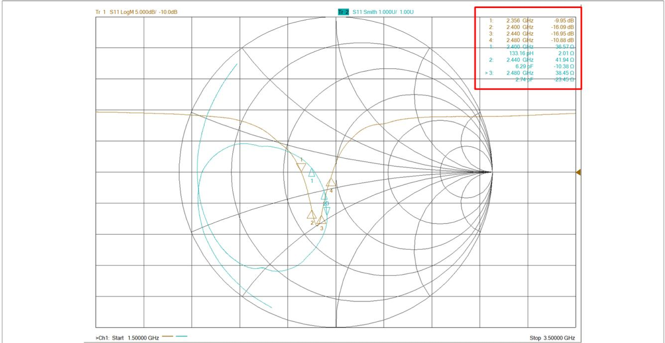
Figure 4. Reflection coefficient s11 – ANT\_A
