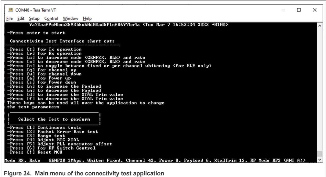
Figure 34. Main menu of the connectivity test application
