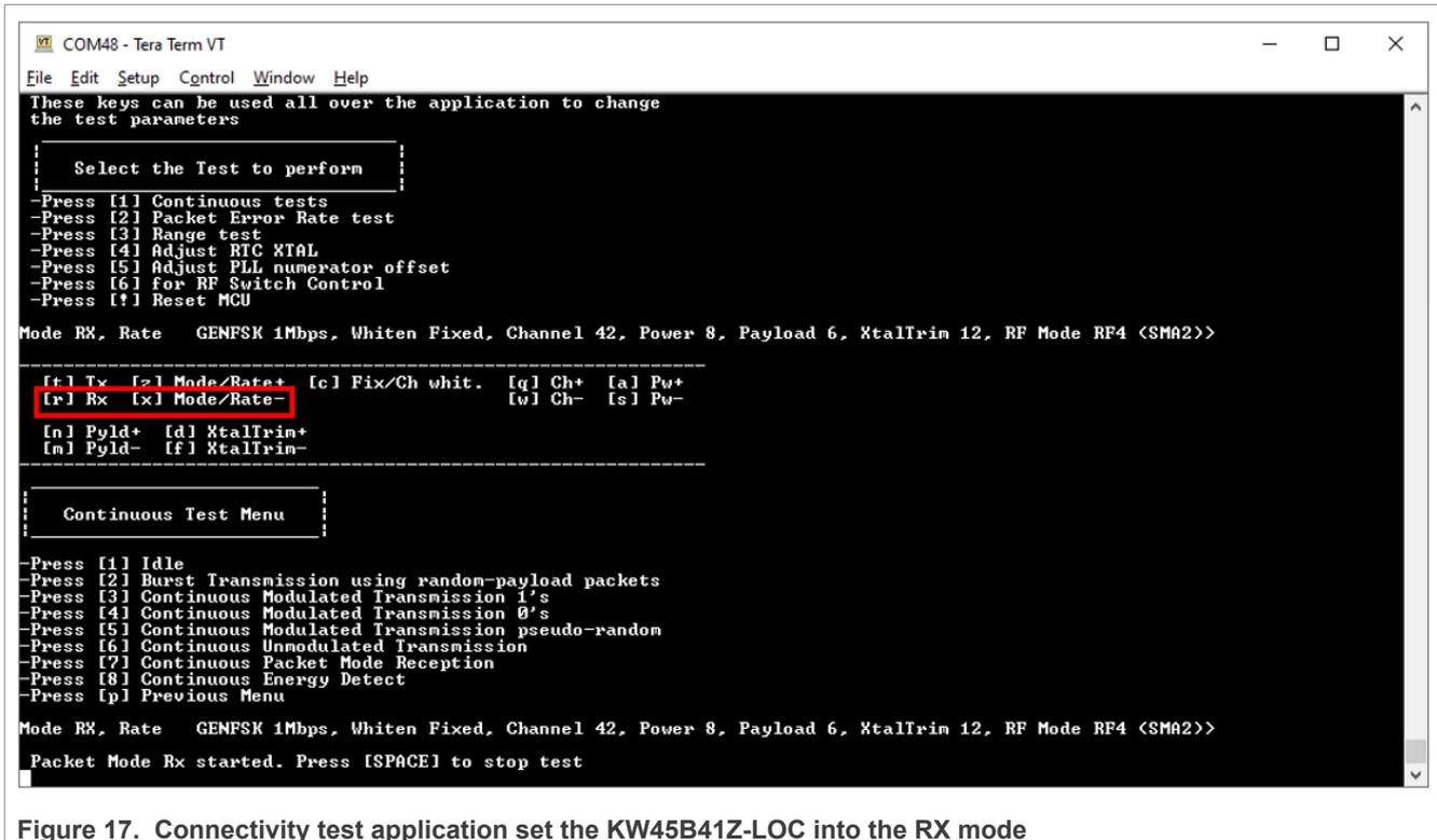
Figure 17. Connectivity test application set the KW45B41Z-LOC into the RX mode
