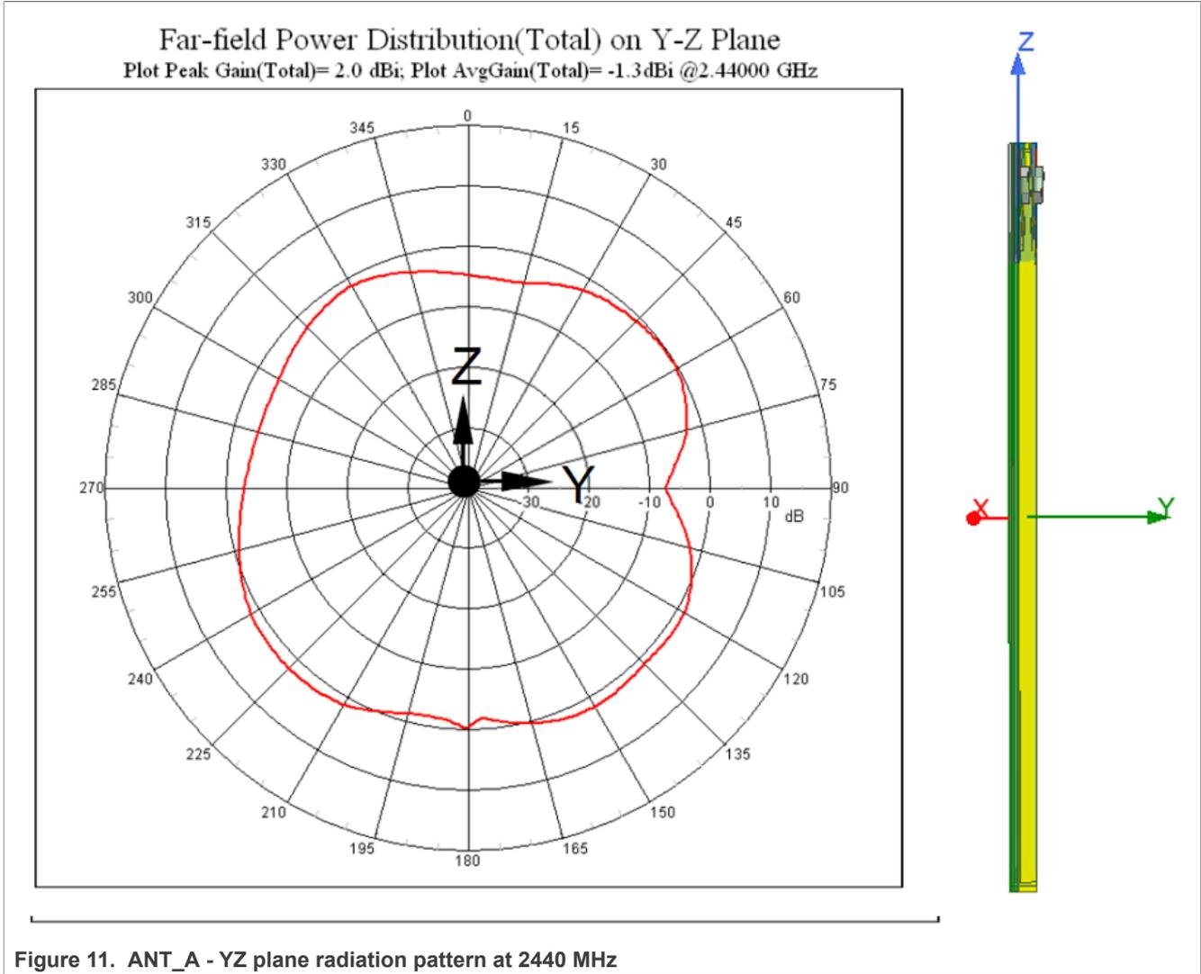
Figure 11. ANT\_A - YZ plane radiation pattern at 2440 MHz
