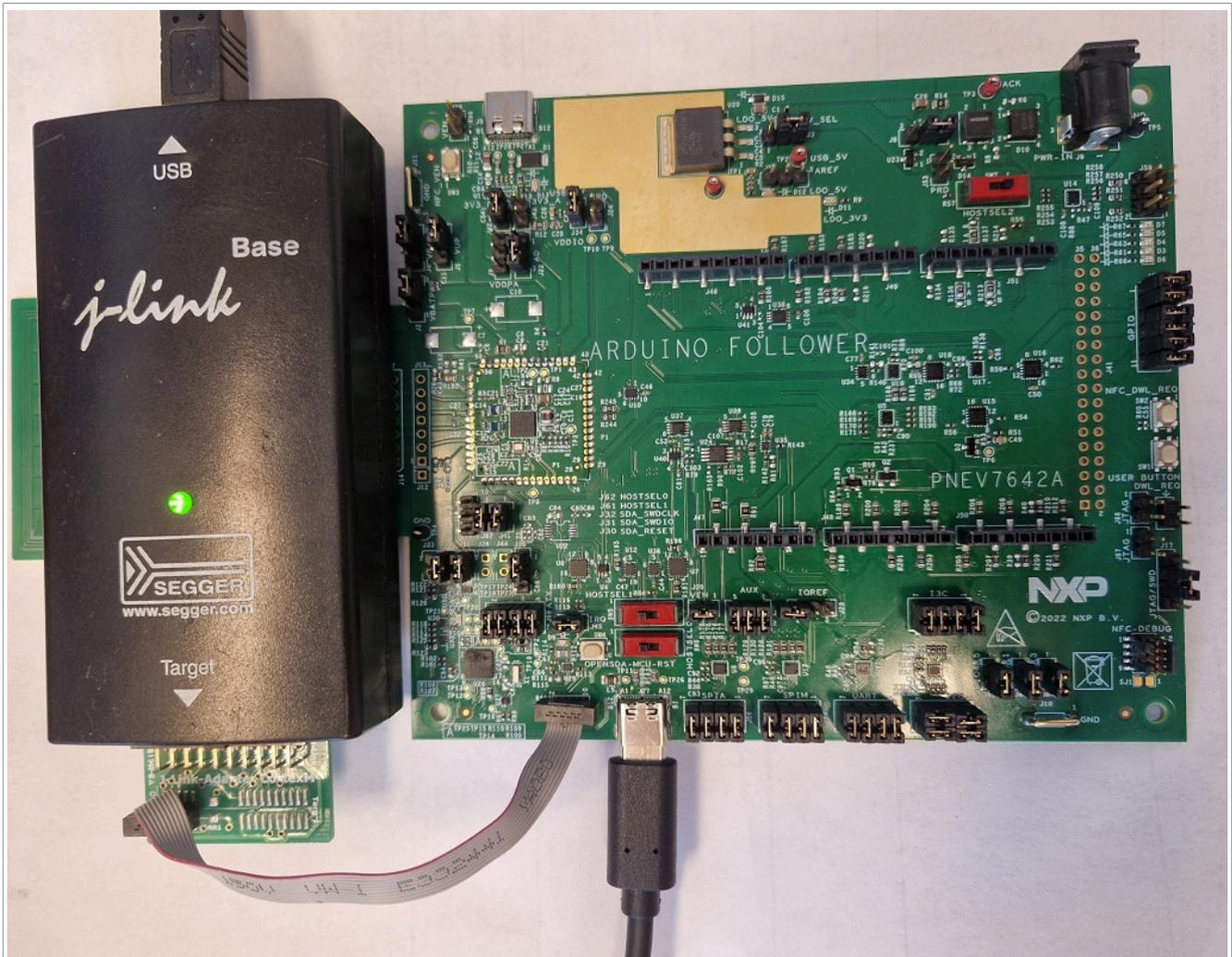
Figure 4. OpenSDA programming connection
