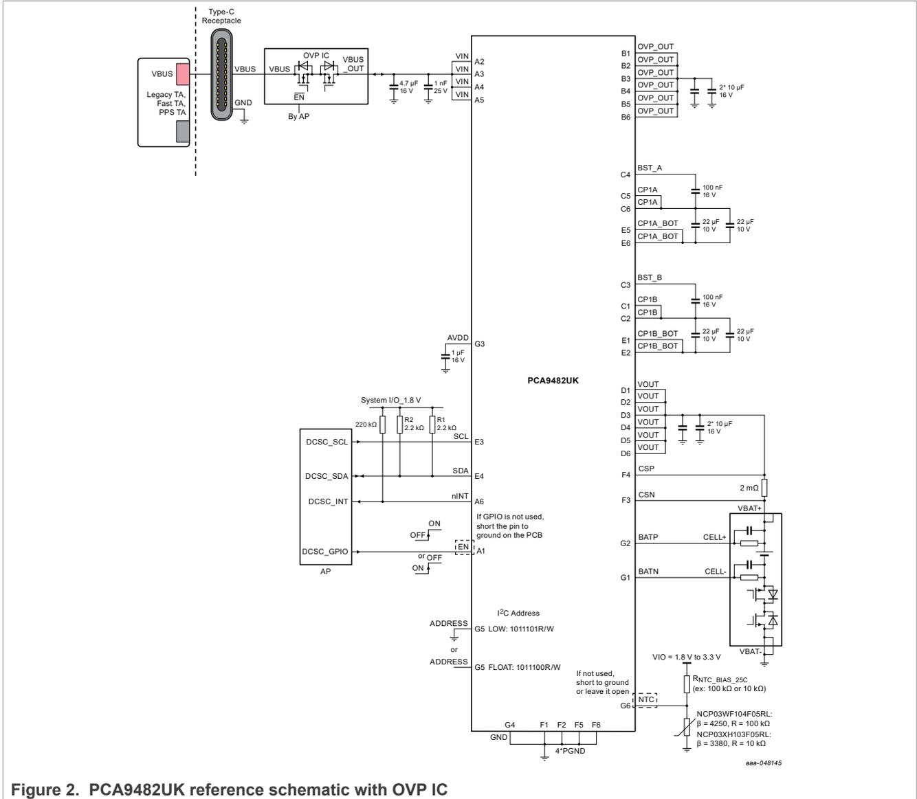
Figure 2. PCA9482UK reference schematic with OVP IC
