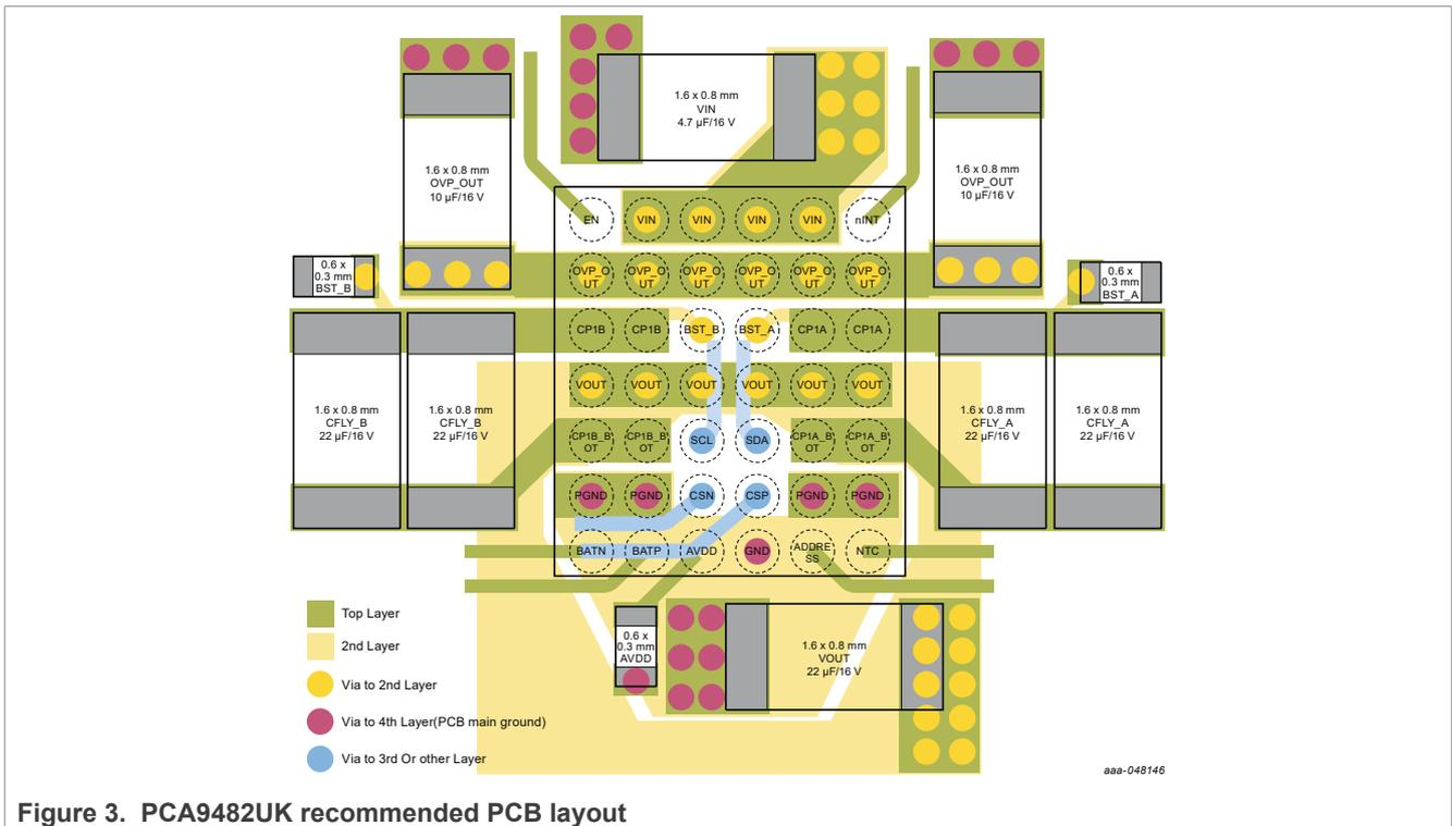
Figure 3. PCA9482UK recommended PCB layout
