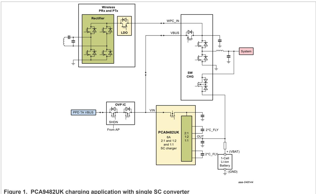
Figure 1. PCA9482UK charging application with single SC converter
