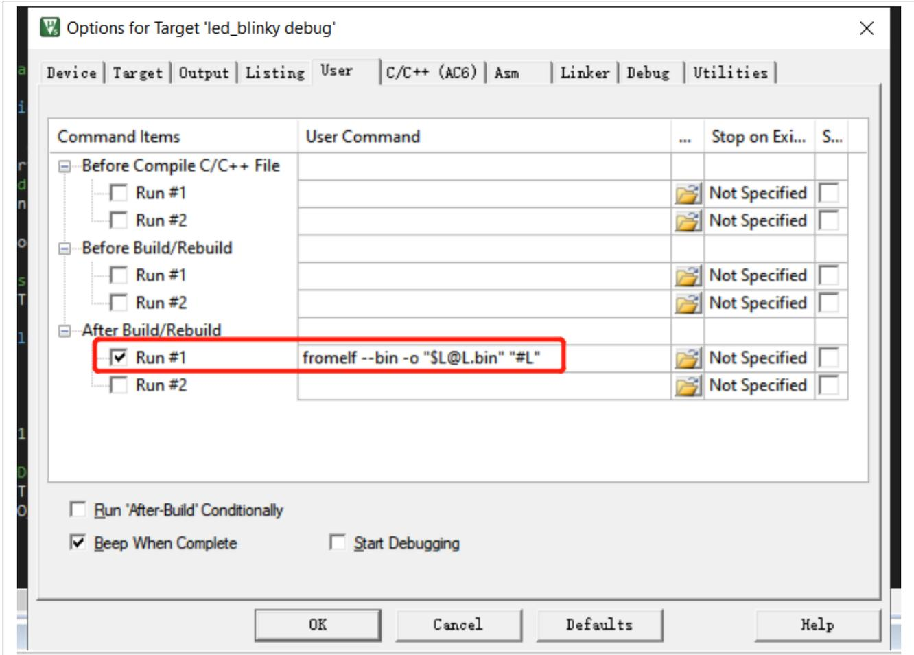
Figure 14. Adding post build command to generate .bin file
