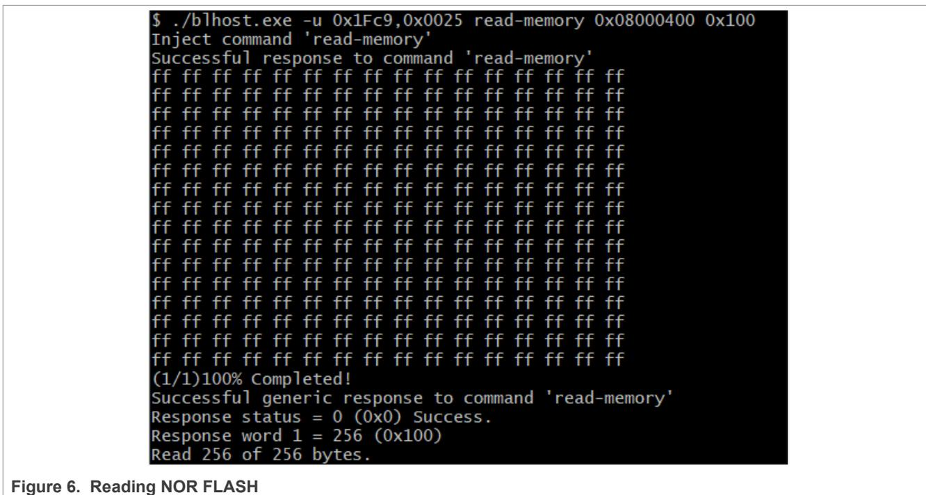
Figure 6. Reading NOR FLASH
