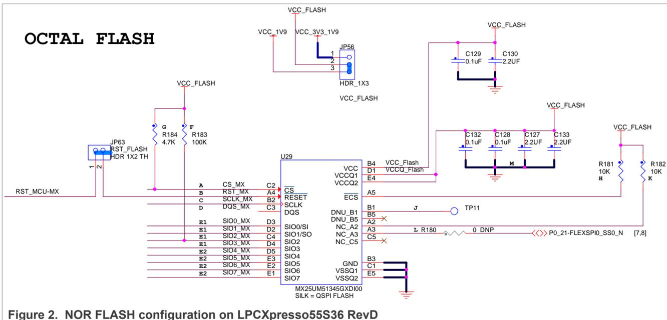
Figure 2. NOR FLASH configuration on LPCXpresso55S36 RevD
