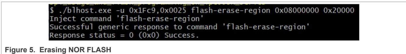
Figure 5. Erasing NOR FLASH
