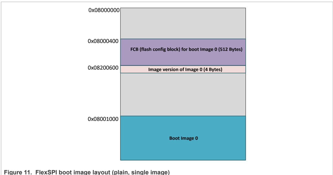
Figure 11. FlexSPI boot image layout (plain, single image)
