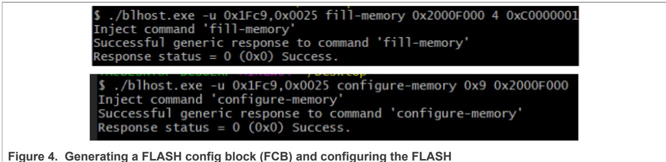
Figure 4. Generating a FLASH config block (FCB) and configuring the FLASH
