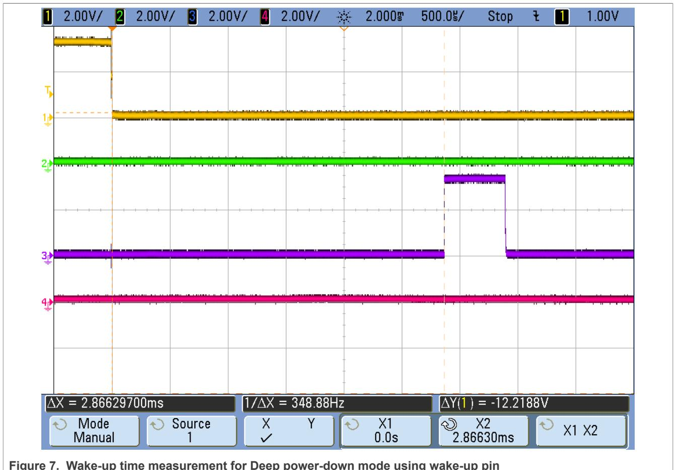
Figure 7. Wake-up time measurement for Deep power-down mode using wake-up pin
