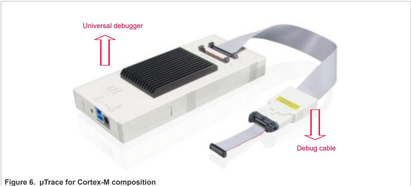
Figure 6.  $\mu$ Trace for Cortex-M composition
