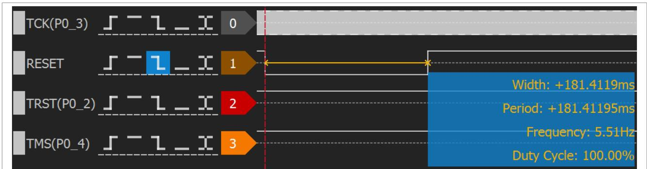
Figure 9. Duration of RESET negative pulse
