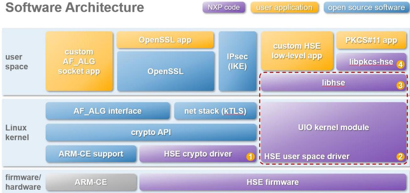
Figure 1. Linux crypto architecture
