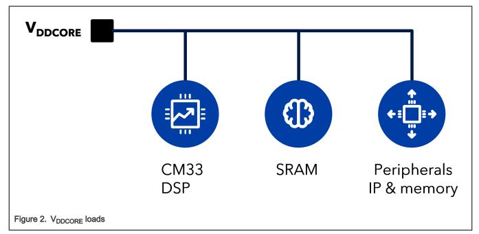
$V_{DDCORE}$  has adjustable voltage from 0.6 V to 1.15 V. The minimum  $V_{DDCORE}$  voltage level in the active mode is determined by the core frequency before the CPU clock divider, as shown in Table 1.  $V_{DDCORE}$  voltages below 0.7 V are for retention mode only.
