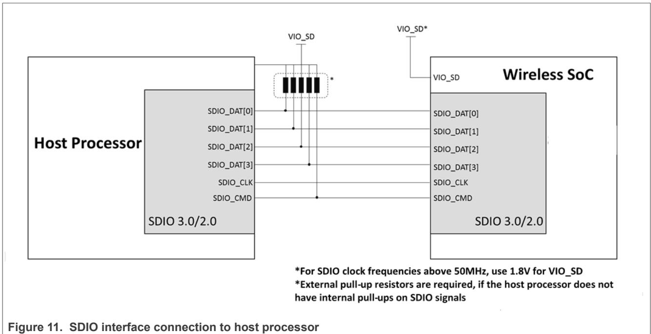
Figure 11. SDIO interface connection to host processor
