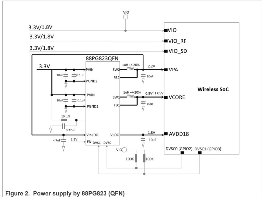
Figure 2. Power supply by 88PG823 (QFN)
