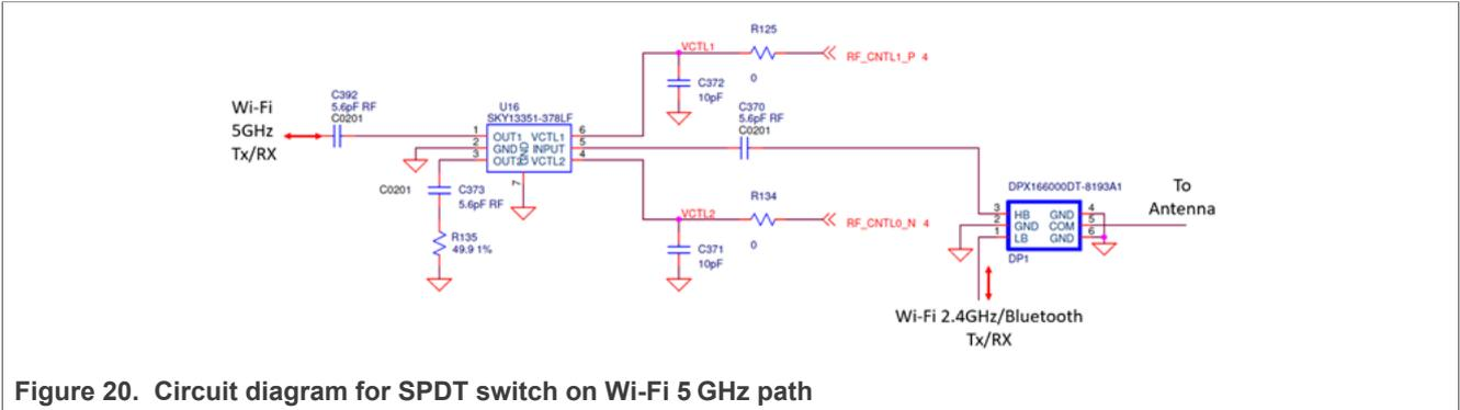
Figure 20. Circuit diagram for SPDT switch on Wi-Fi 5 GHz path
