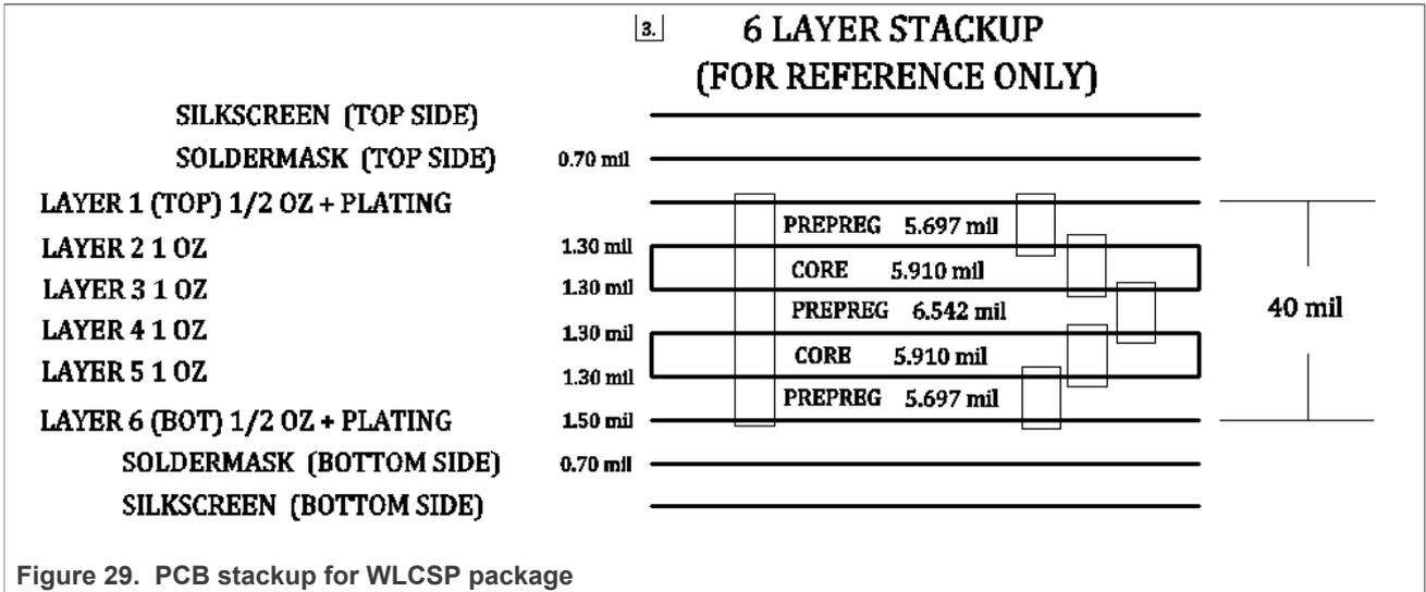
Figure 29. PCB stackup for WLCSP package
