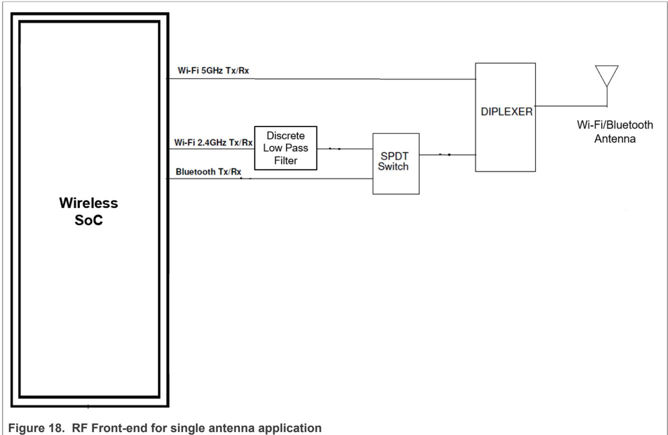
Figure 18. RF Front-end for single antenna application
