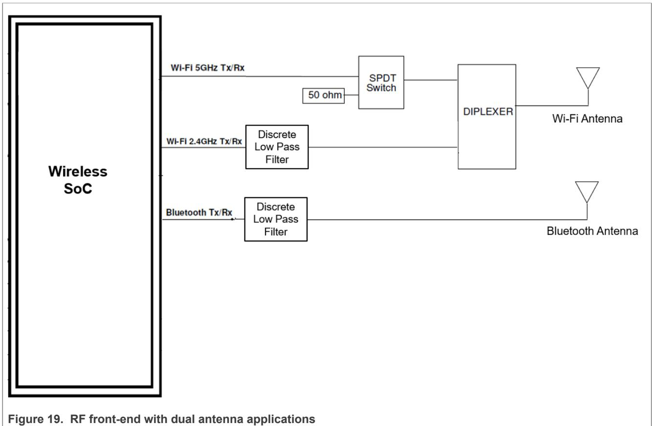
Figure 19. RF front-end with dual antenna applications
