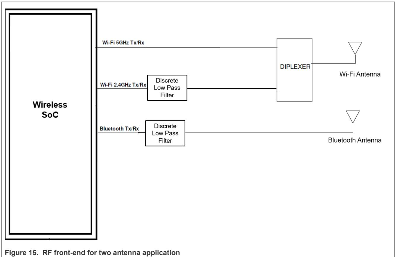
Figure 15. RF front-end for two antenna application
