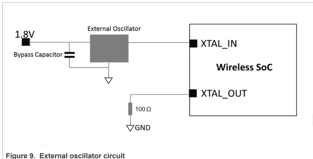
Figure 9. External oscillator circuit
