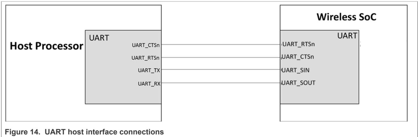
Figure 14. UART host interface connections
