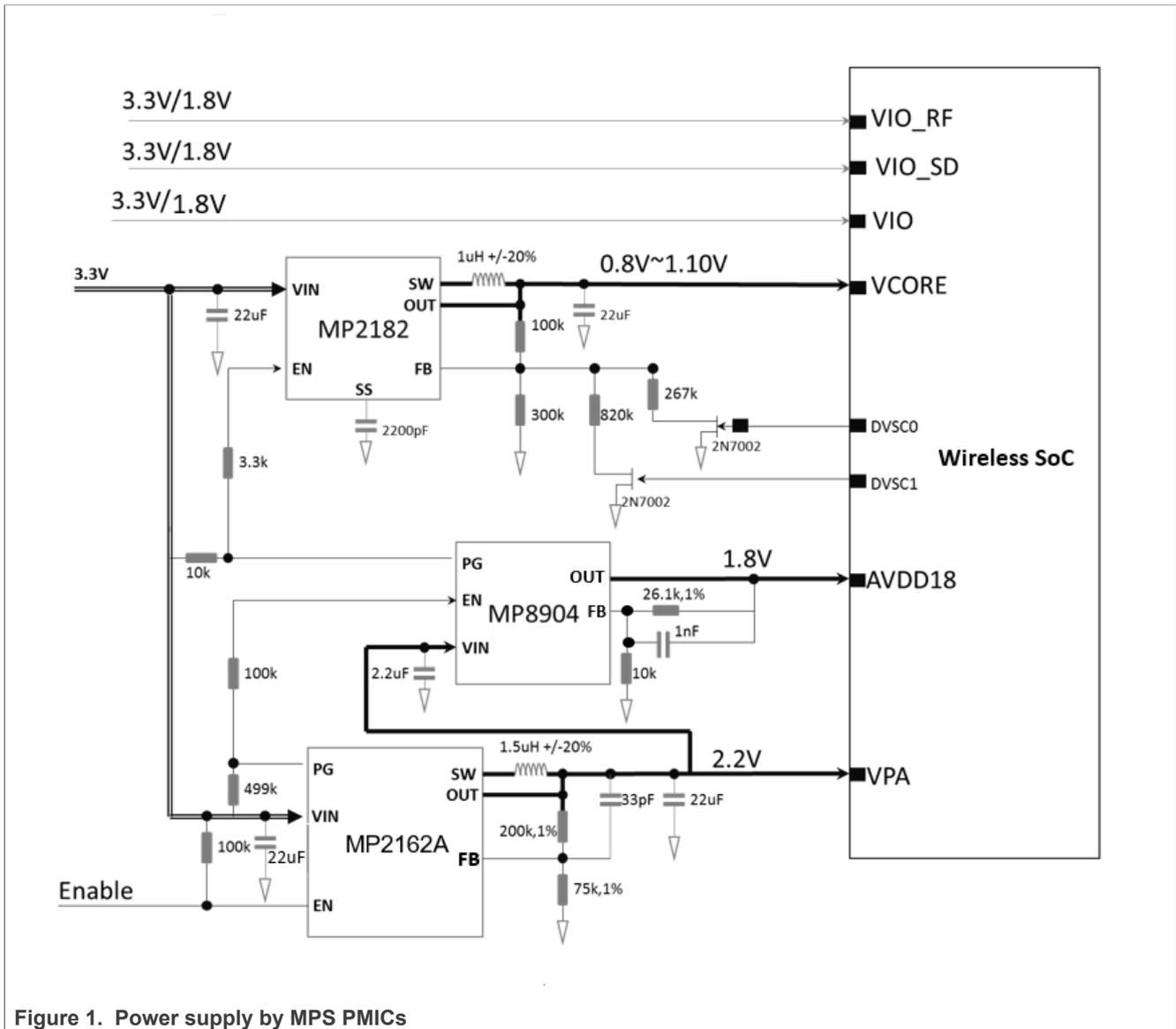
Figure 1. Power supply by MPS PMICs
