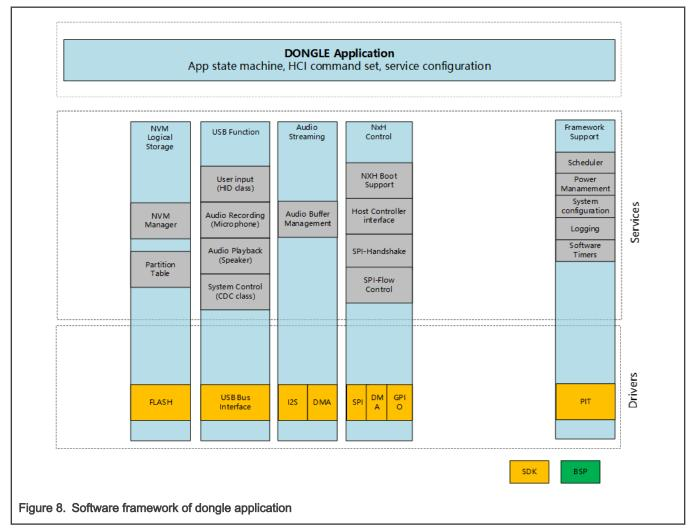
The dongle application implements the configuration of NxH3670 and the transmission of audio data.
