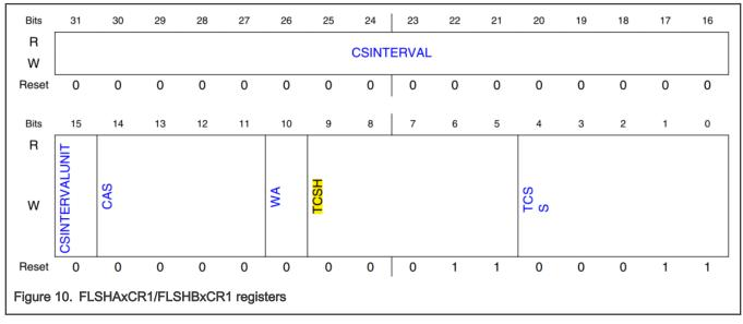
For example, for HyperRAM device, TCSH and TCSS is equivalent to the t<sub>CSH</sub> and t<sub>CSS</sub> timing parameters. For example, Table 2 shows the related parameters in 7KS0642GAHI02 HyperRAM device.
