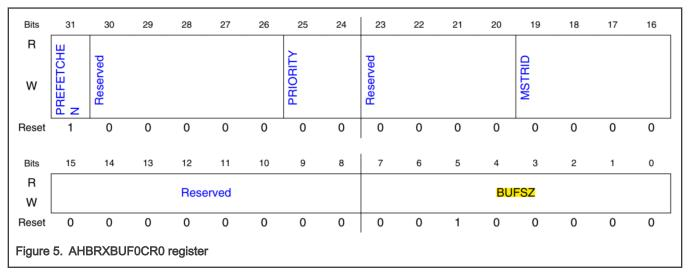
FlexSPI specifies different buffer size for different master. Some masters may have the dedicated prefetch buffer, which can optimize performance in some applications. The AHB RX buffer is assigned to different masters according to the register fields, AHBRXBUF0CR0 [MSTRID] - AHBRXBUF3CR0 [MSTRID].
