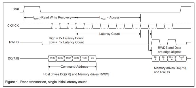
Figure 1 shows a read transaction with single latency count.
