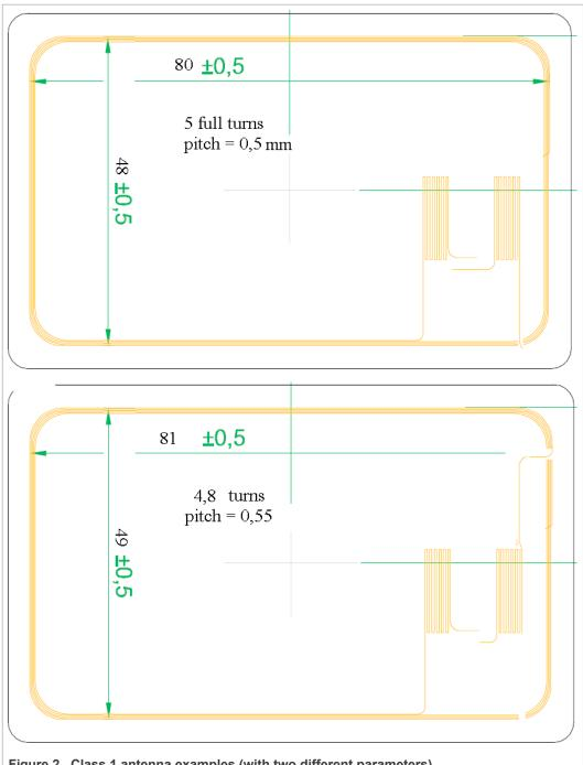
Figure 2. Class 1 antenna examples (with two different parameters)
