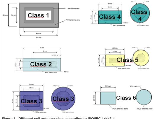
Figure 1. Different coil antenna sizes according to ISO/IEC 14443-1
