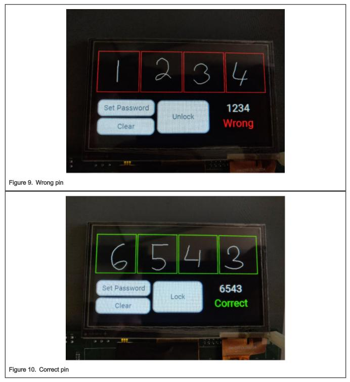
The simple example can be extended in several ways. For this application note, a simple digital lock with a 4-digit pin code as shown in Figure 9 and Figure 10 was implemented.
