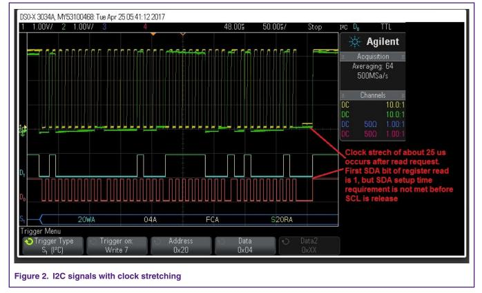
Figure 3. on page 3 shows the clock stretching timing.
