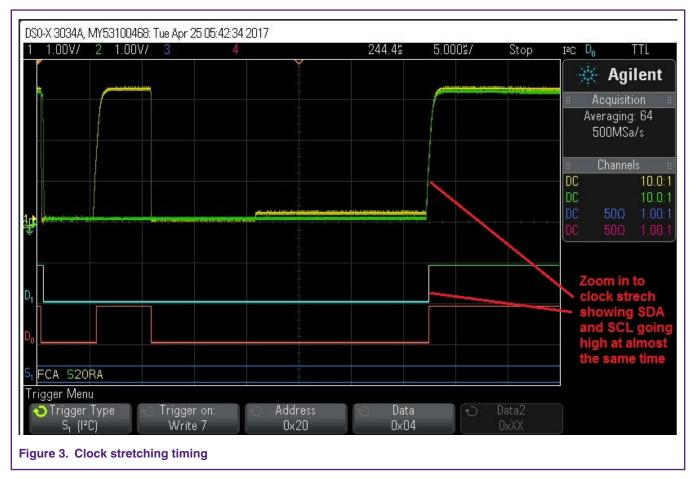
Figure 3. on page 3 shows the SDA and SCL release at almost the same time. For the I<sup>2</sup>C timing definition to match the values in Figure 4. on page 3, the tSU:DAT minimum value must be around 100 ns in the fast mode and 250 ns in the standard mode. Therefore, the above timing violates the specification.
