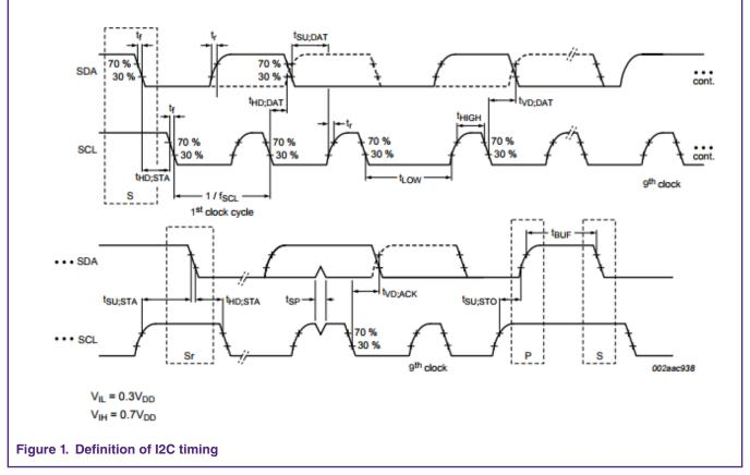
The Kinetis IP provides register I2Cx\_F to tune the timing. The reference manual provides the reference table on how to impact the I<sup>2</sup>C baud rate and data hold time. For the slave mode, this register also heavily impacts the timing and incorrect settings may
