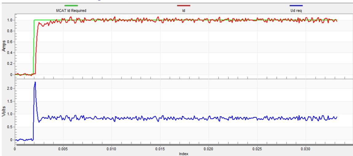
**Figure 44. Optimal step response of the  $I_d$  current controller**
