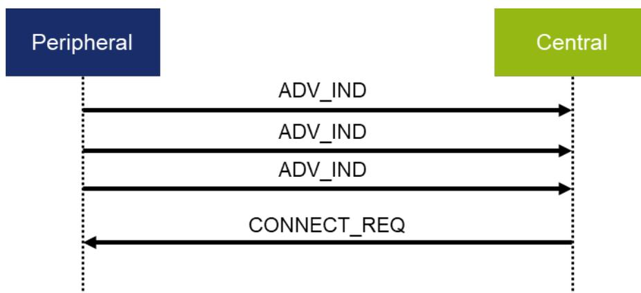
Figure 1. GAP peripheral and central
