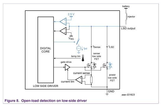
If a load is connected, the voltage on the LSD output pin is close to  $V_{BAT}$ . This voltage is compared to a 2.5 V comparator.
