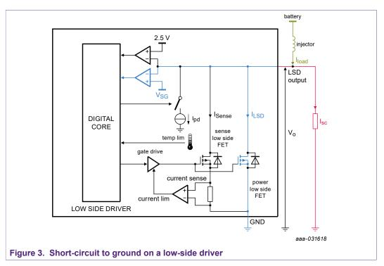
• In normal condition (when there is no short-circuit to ground and  $I_{sc} = 0$  A), the output voltage is  $V_o = I_{load} \times R_{DS(on)}$ . This voltage is compared to a reference  $V_{SG}$  (typically 30 mV, maximum value is 75 mV). If  $V_o > V_{SG}$ , the digital core detects no short-circuit to ground (no open load on).
