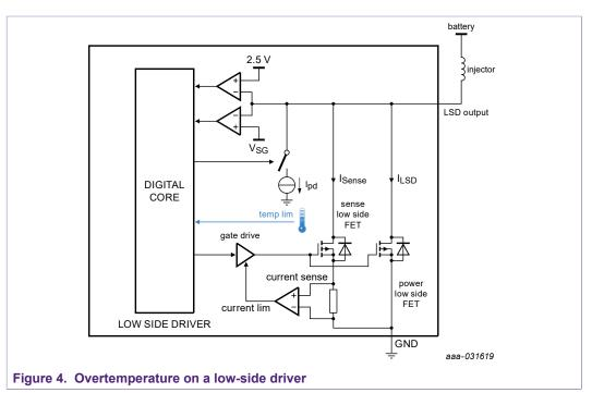
If the temperature on the LSD goes over 175  $^{\circ}$ C (typical), the output is switched off, the OT bit is set and no other driver is affected. When the bit is set, the fault must disappear and the bit must be manually set to logic 0 to be cleared.
