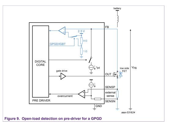
If the load is connected, the voltage seen on the FB pin is close to the battery voltage.
