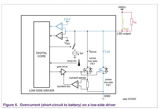
In addition, the corresponding bit OC in the status register is set. When the bit is set, the fault must disappear and the bit must be manually set to logic 0 to be cleared.
