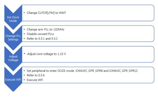
Assume that the core voltage is reduced to 132 MHz. If the core frequency switches from 24 MHz to 132 MHz, the core voltage should be increased first.
