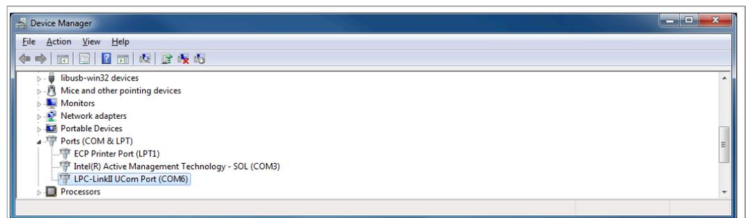
**Figure 18. Retrieving COM port number from Device Manager**
