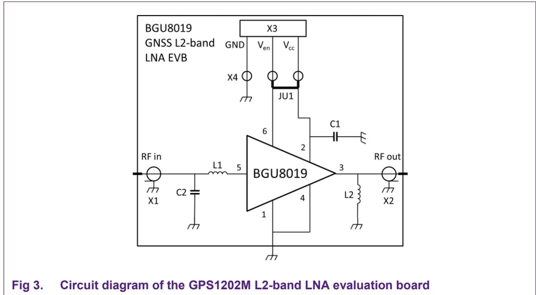
Fig 3. Circuit diagram of the GPS1202M L2-band LNA evaluation board
