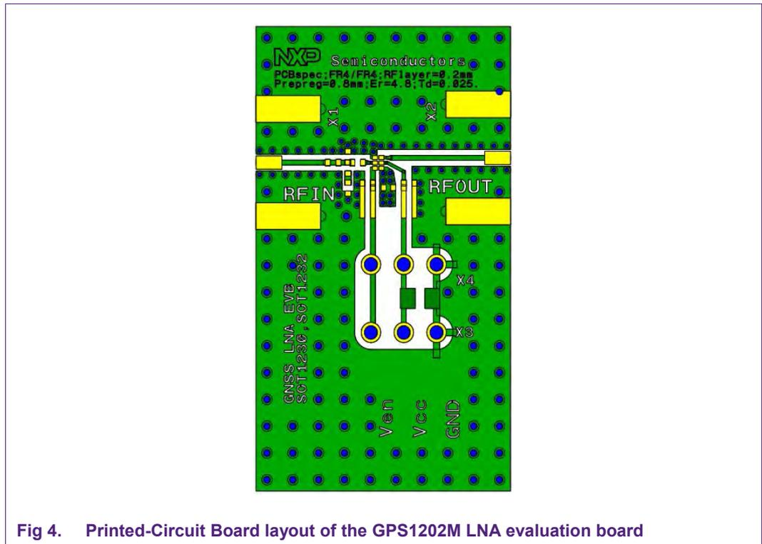
Fig 4. Printed-Circuit Board layout of the GPS1202M LNA evaluation board
