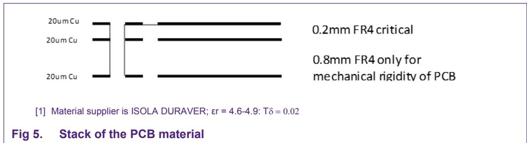
Fig 5. Stack of the PCB material
