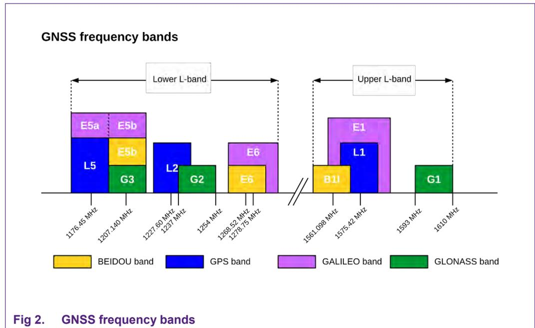
Fig 2. GNSS frequency bands
