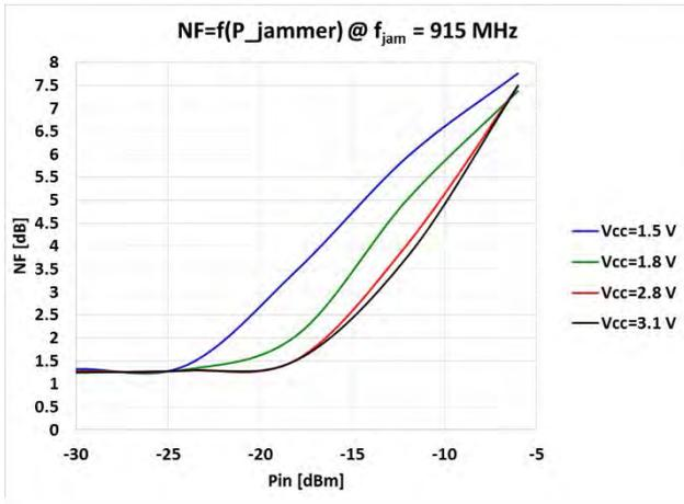
Fig 17. NF versus jammer power at 915 MHz
