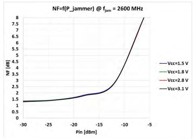
Fig 22. NF versus jammer power at 2600 MHz
