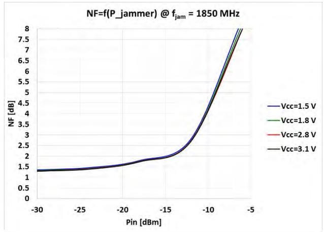
Fig 20. NF versus jammer power at 1850 MHz
