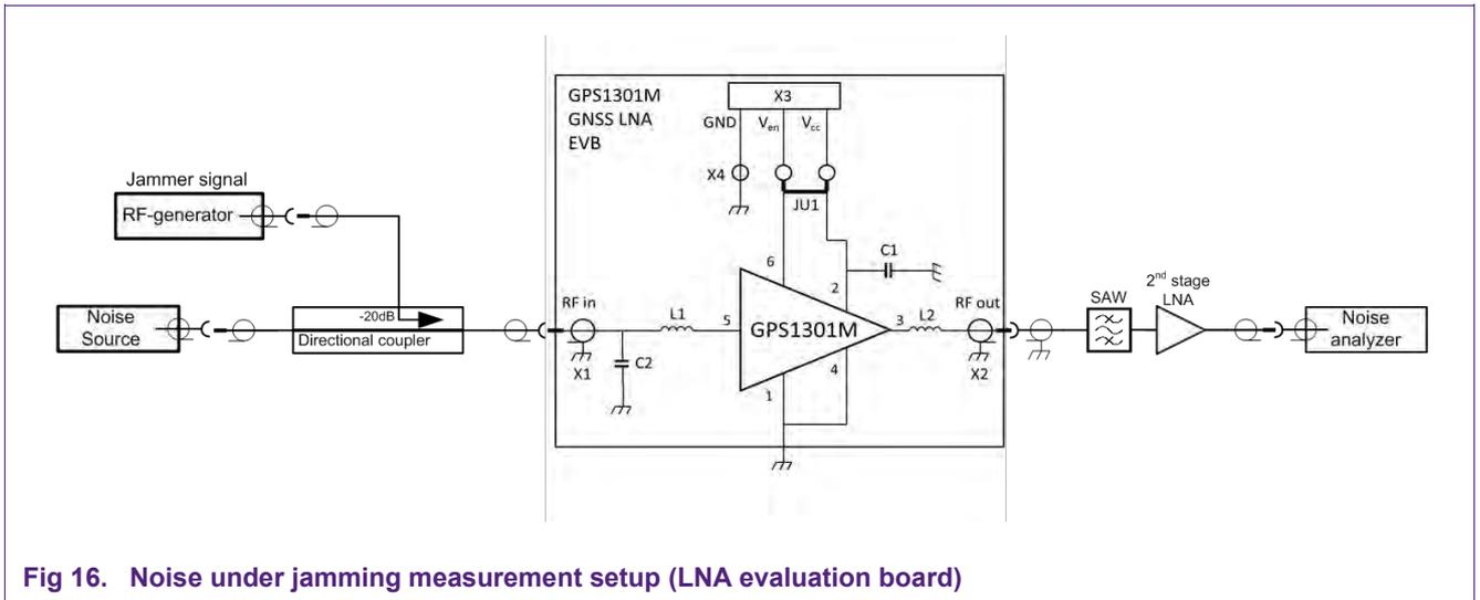
Fig 16. Noise under jamming measurement setup (LNA evaluation board)
