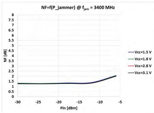
Fig 23. NF versus jammer power at 3400 MHz
