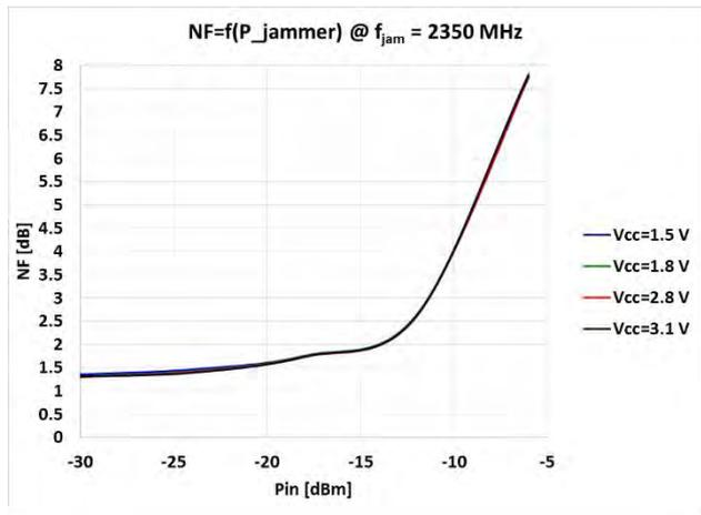
Fig 21. NF versus jammer power at 2350 MHz
