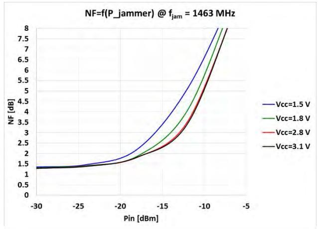
Fig 18. NF versus jammer power at 1463 MHz
