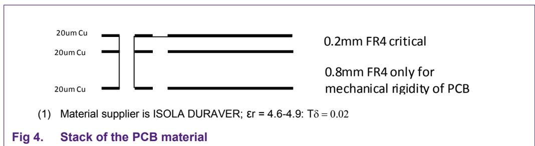
Fig 4. Stack of the PCB material
