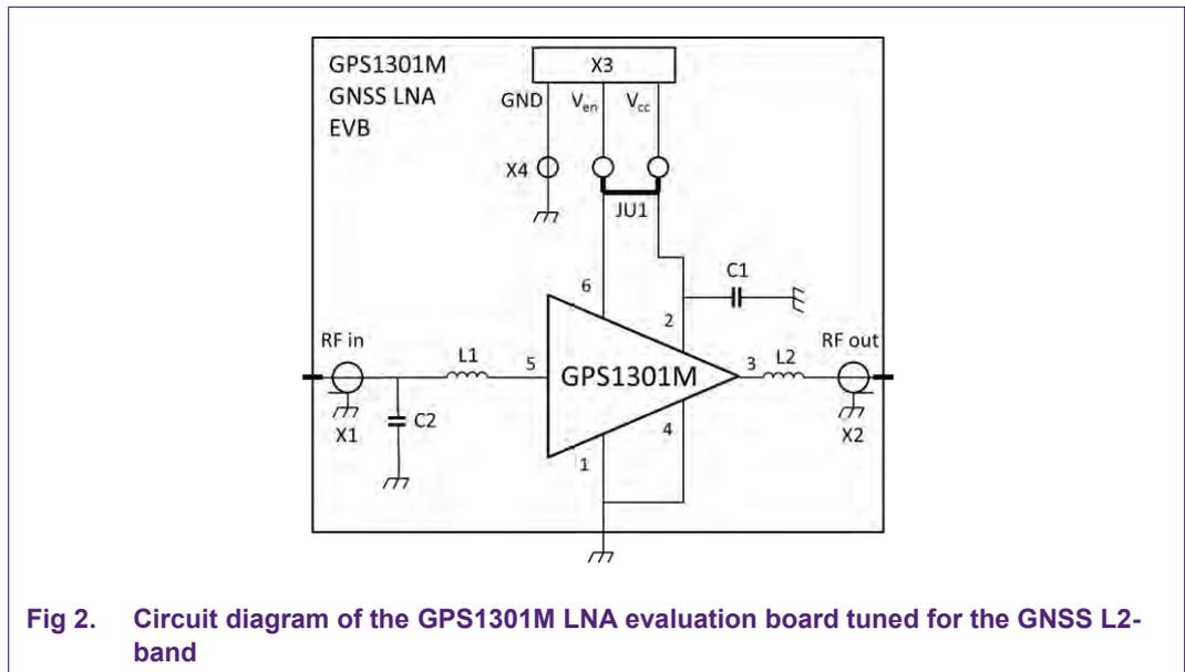
Fig 2. Circuit diagram of the GPS1301M LNA evaluation board tuned for the GNSS L2-band
