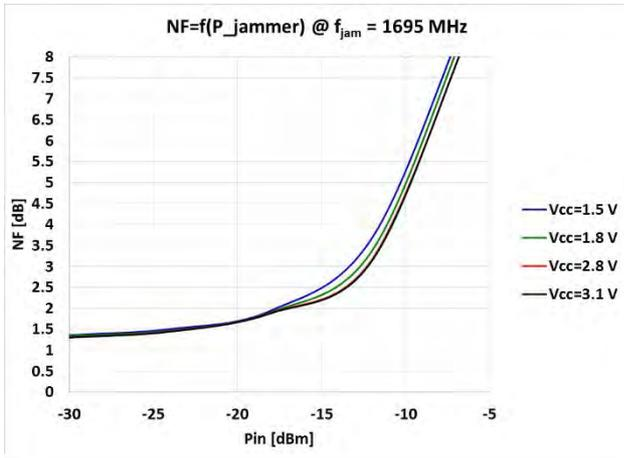
Fig 19. NF versus jammer power at 1695 MHz
