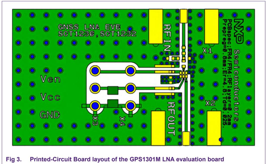
Fig 3. Printed-Circuit Board layout of the GPS1301M LNA evaluation board
