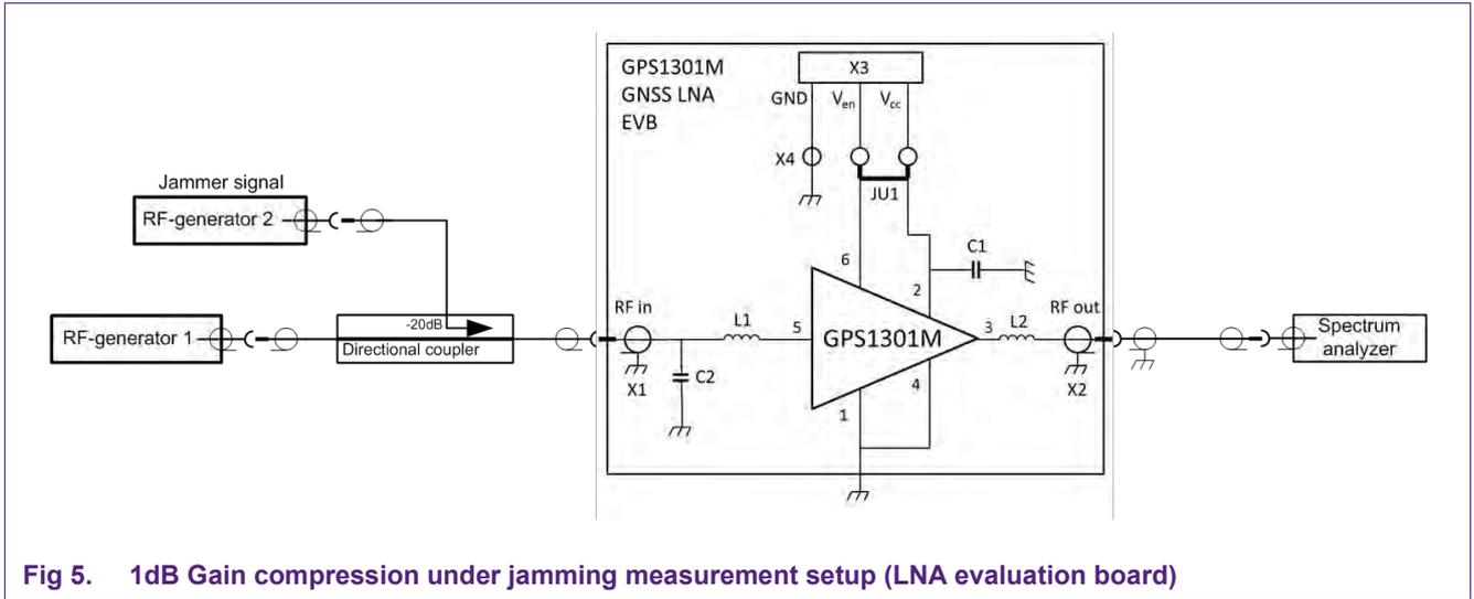
Fig 5. 1dB Gain compression under jamming measurement setup (LNA evaluation board)
