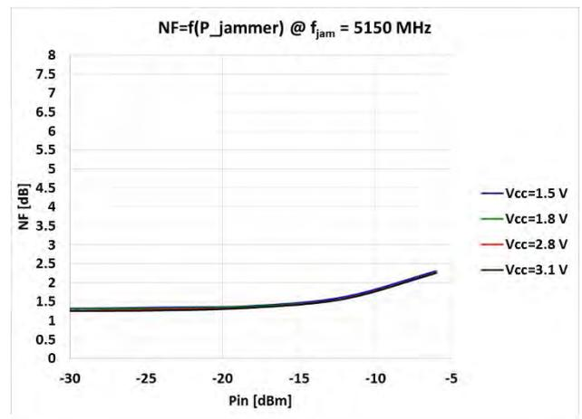
Fig 24. NF versus jammer power at 5150 MHz
