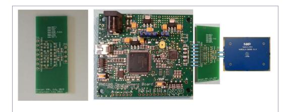
Fig 5. PNEV5180B board and main parts: MCU, empty matching network and loop antenna
