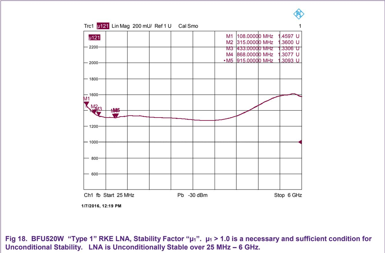
Fig 18. BFU520W “Type 1” RKE LNA, Stability Factor “ $\mu_1$ ”.  $\mu_1 > 1.0$  is a necessary and sufficient condition for Unconditional Stability. LNA is Unconditionally Stable over 25 MHz – 6 GHz.
