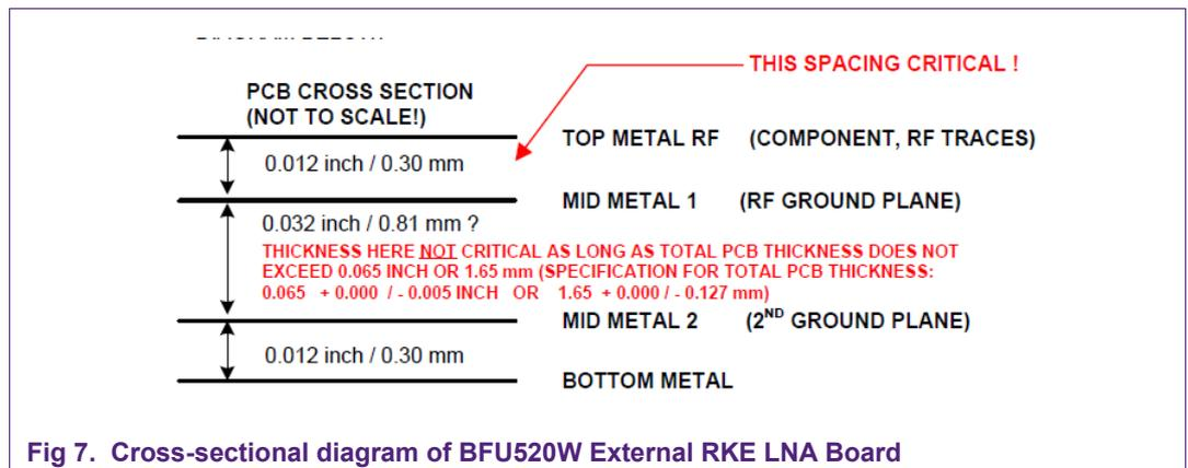
Fig 7. Cross-sectional diagram of BFU520W External RKE LNA Board
