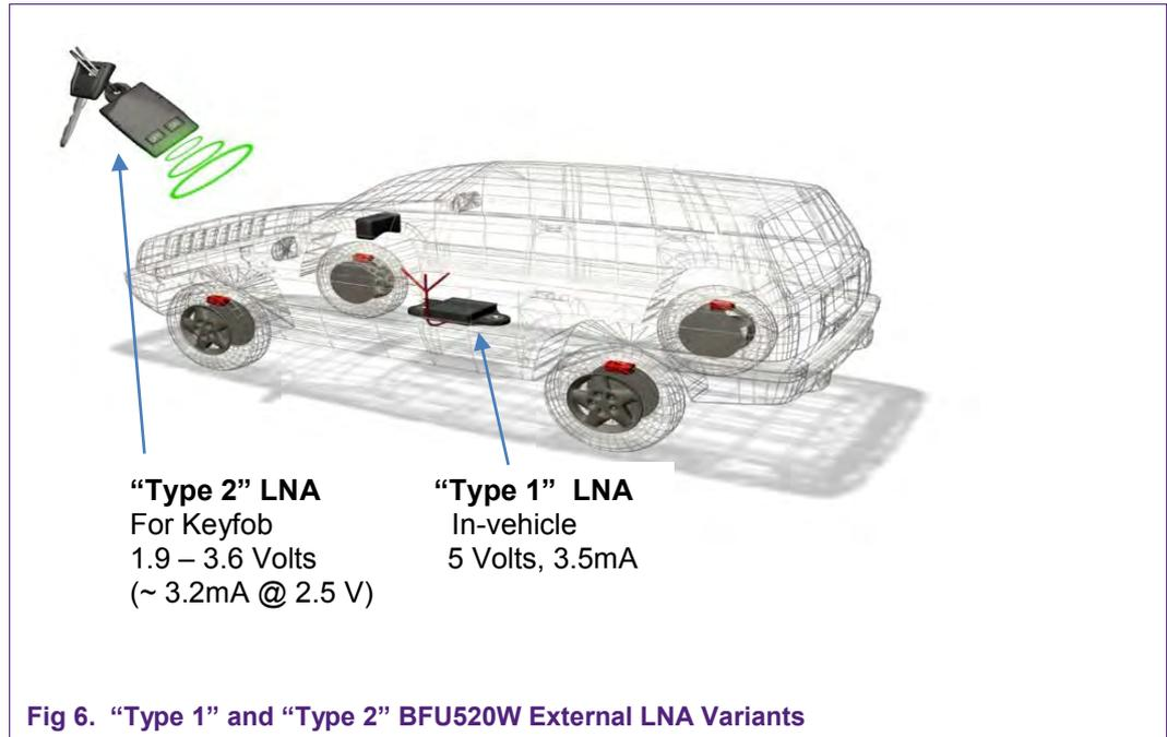
Fig 6. "Type 1" and "Type 2" BFU520W External LNA Variants
