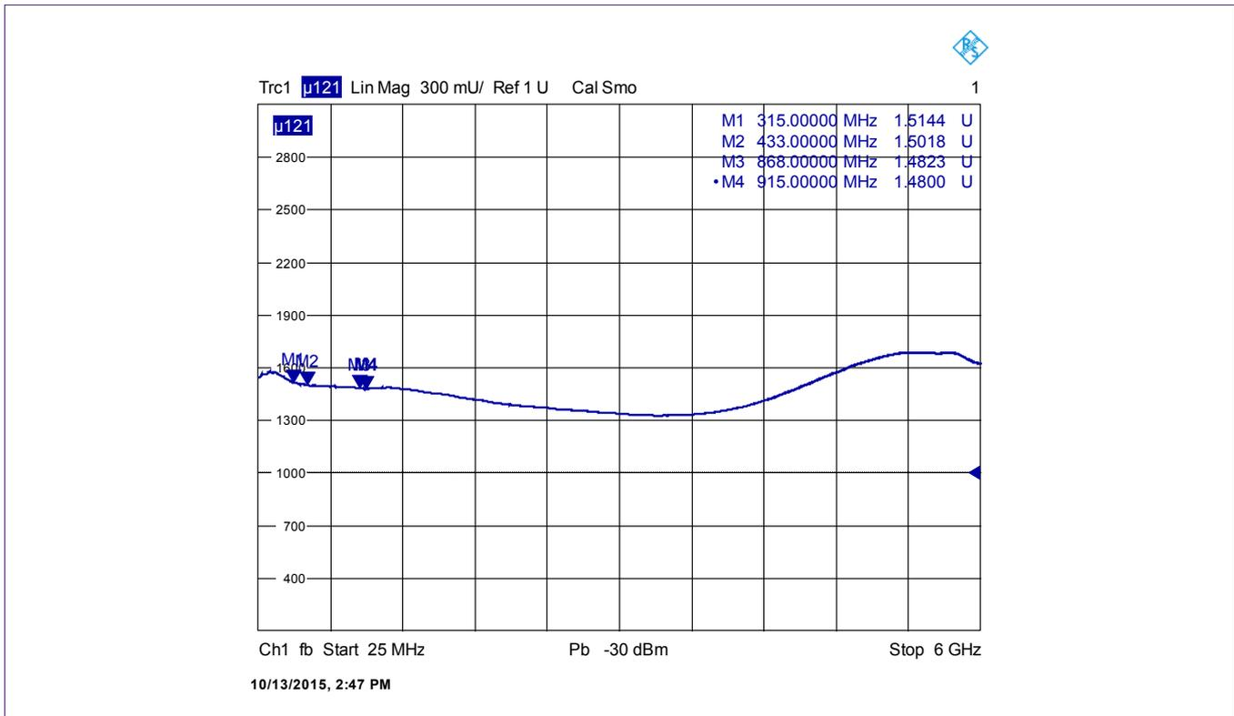
Fig 30. Stability factor  $\mu_1$  at 3.0 volts, “Type 2” BFU520W RKE LNA, for 25 MHz – 6 GHz.
