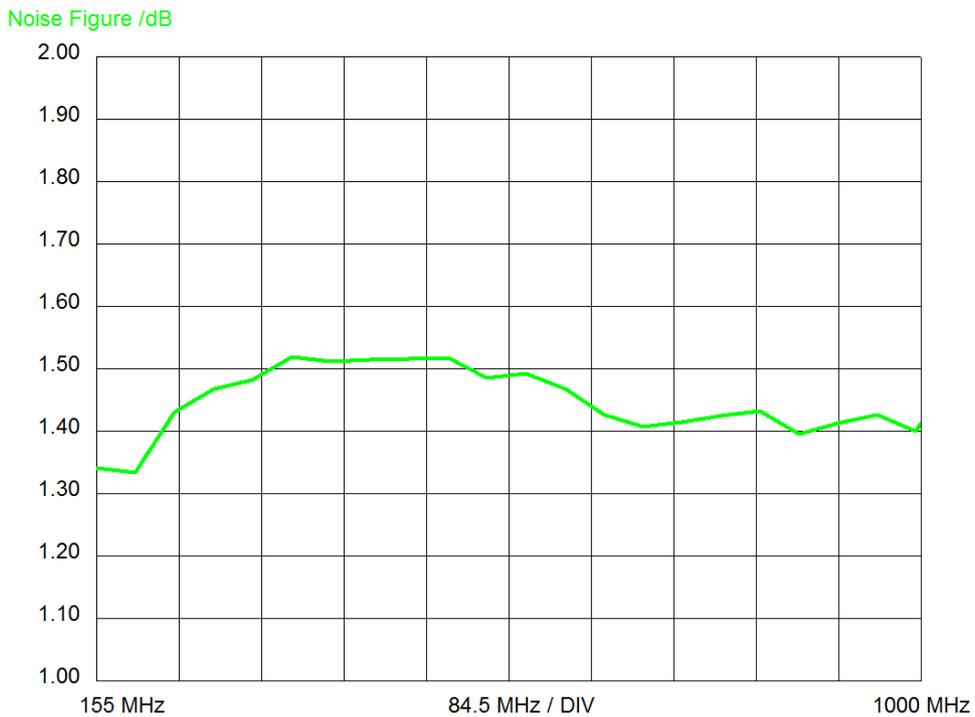
Fig 34. Noise Figure at 3.0 volts, “Type 2” BFU520W RKE LNA
