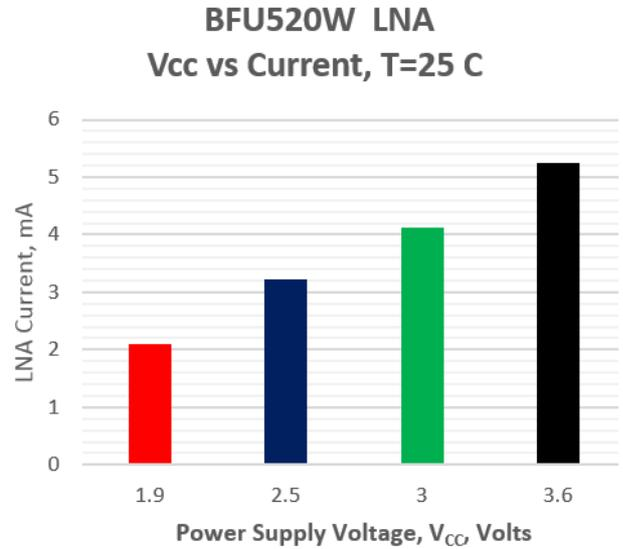
Fig 23. Variation in LNA current & collector-emitter voltage vs. battery voltage for a “Type 2” BFU520W RKE Keyfob LNA.
