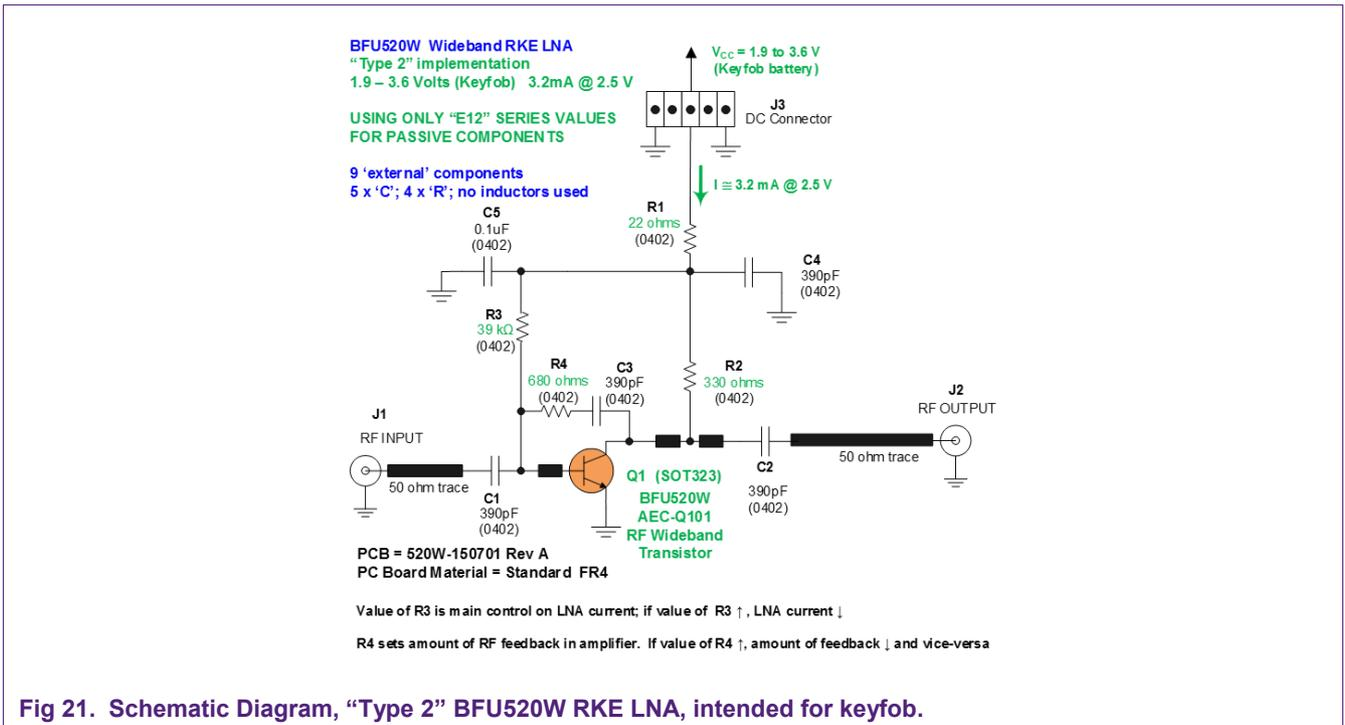
Fig 21. Schematic Diagram, “Type 2” BFU520W RKE LNA, intended for keyfob.
