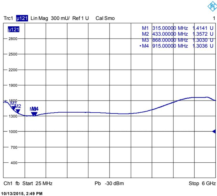
Fig 28. Stability factor  $\mu_1$  at 1.9 volts, “Type 2” BFU520W RKE LNA, for 25 MHz – 6 GHz.
