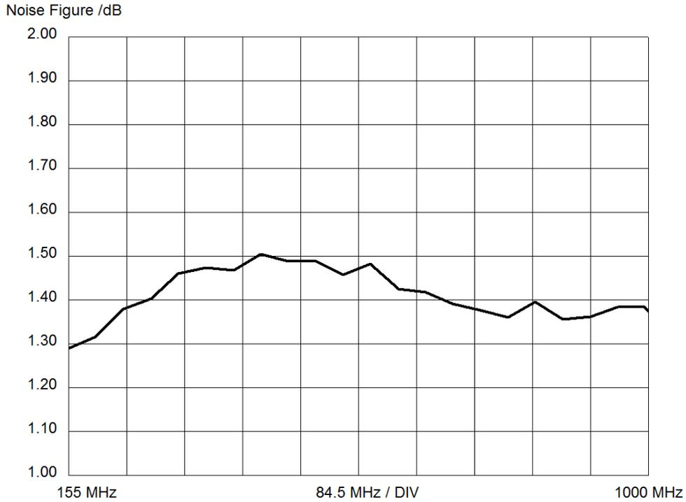
Fig 35. Noise Figure at 3.6 volts, “Type 2” BFU520W RKE LNA
