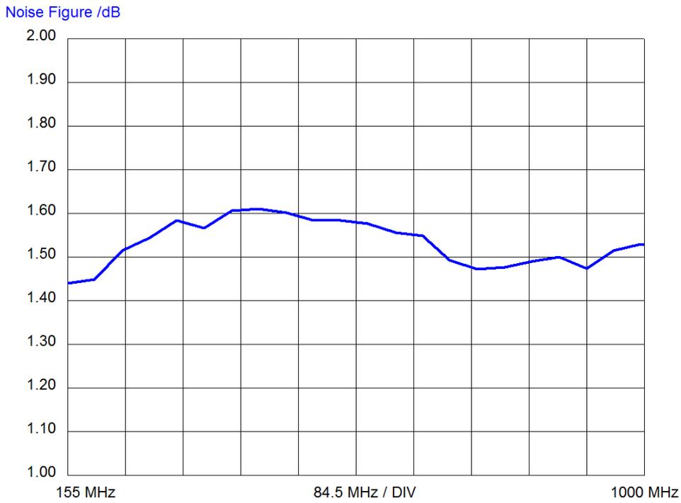
Fig 33. Noise Figure at 2.5 volts, “Type 2” BFU520W RKE LNA
