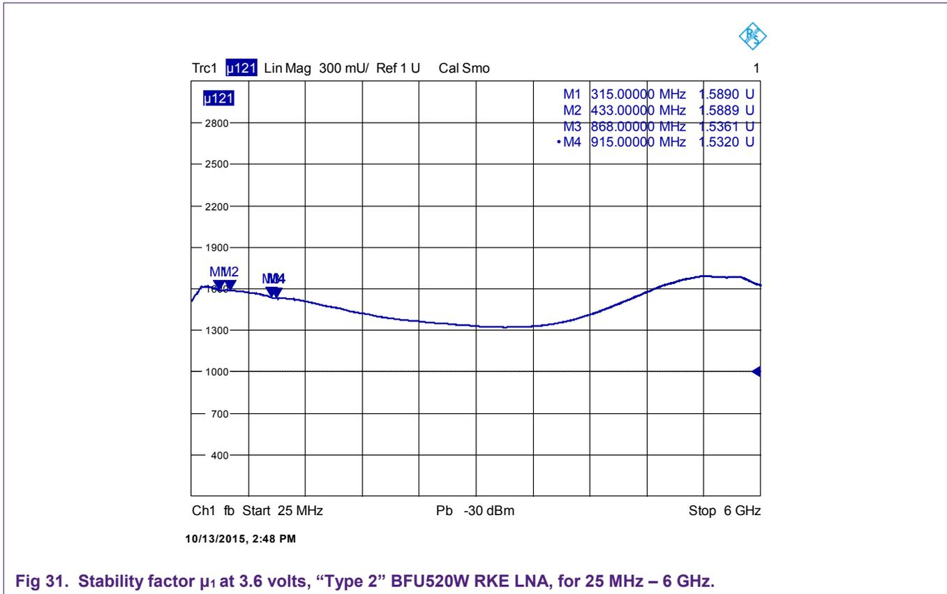
Fig 31. Stability factor  $\mu_1$  at 3.6 volts, “Type 2” BFU520W RKE LNA, for 25 MHz – 6 GHz.
