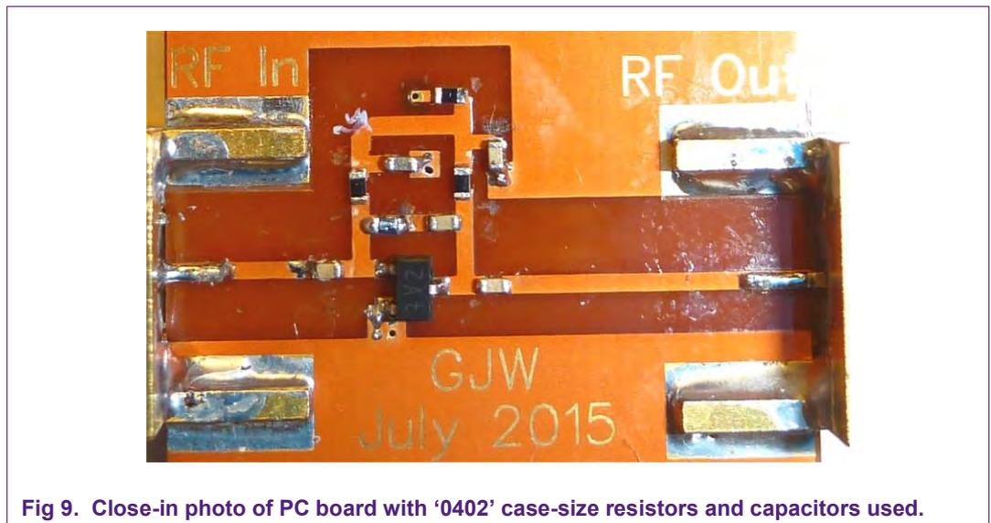
Fig 9. Close-in photo of PC board with '0402' case-size resistors and capacitors used.
