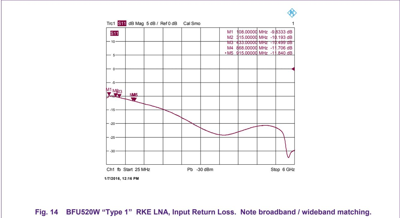
Fig. 14 BFU520W “Type 1” RKE LNA, Input Return Loss. Note broadband / wideband matching.
