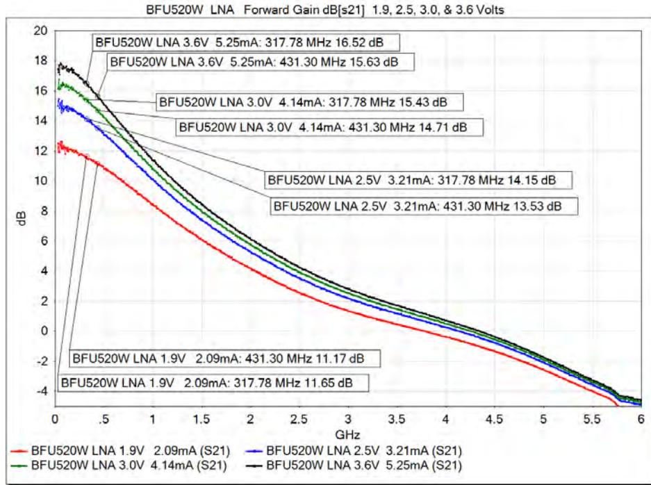
Fig 25. Gain vs Battery Voltage for a “Type 2” BFU520W RKE LNA, for 25 MHz – 6 GHz. We see a total gain variation of ~ -4.5 dB at 315 or 433 MHz as voltage decreases from 3.6 V down to 1.9V.
