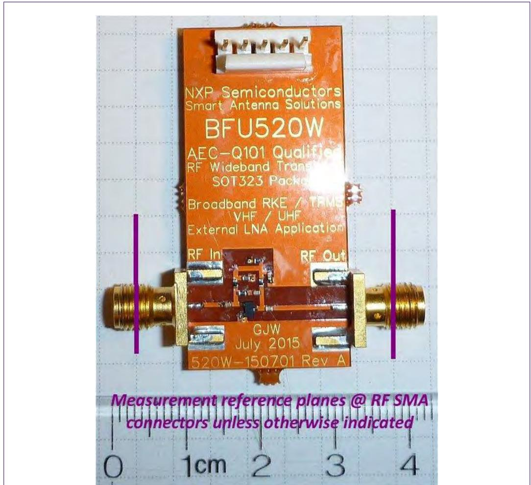
Fig 8. Photo of assembled BFU520W LNA PC board. Measurement reference planes for data shown in this document are as shown at RF connectors unless otherwise indicated.
