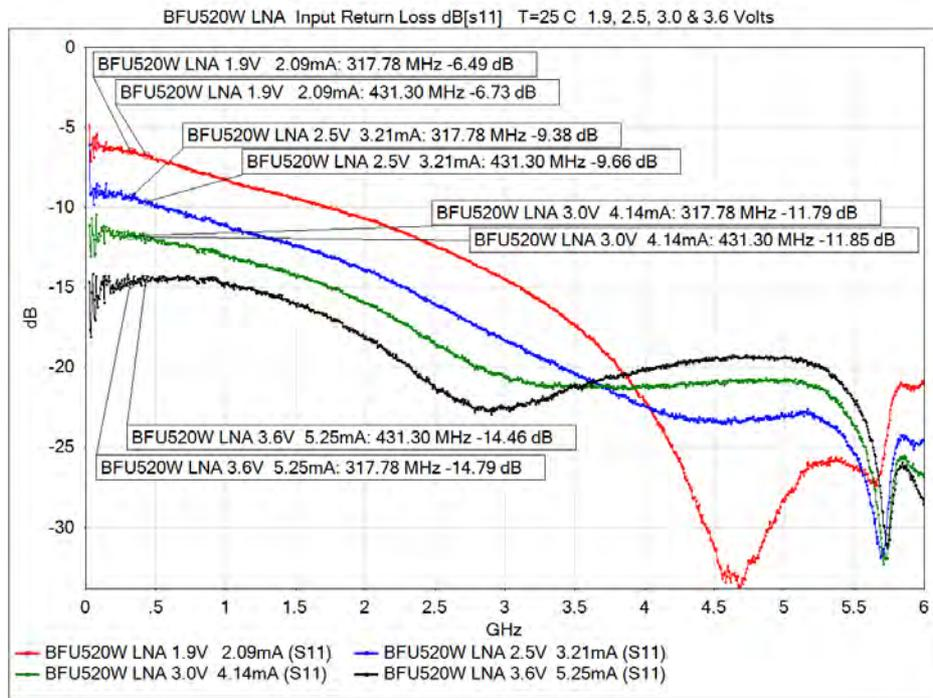
Fig 24. Input Return Loss vs Battery Voltage for a “Type 2” BFU520W RKE LNA, for 25 MHz – 6 GHz. Note, input match degrades as voltage decreases.
