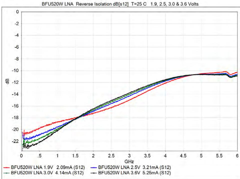
Fig 26. Reverse Isolation vs Battery Voltage for a “Type 2” BFU520W RKE LNA, for 25 MHz – 6 GHz.
