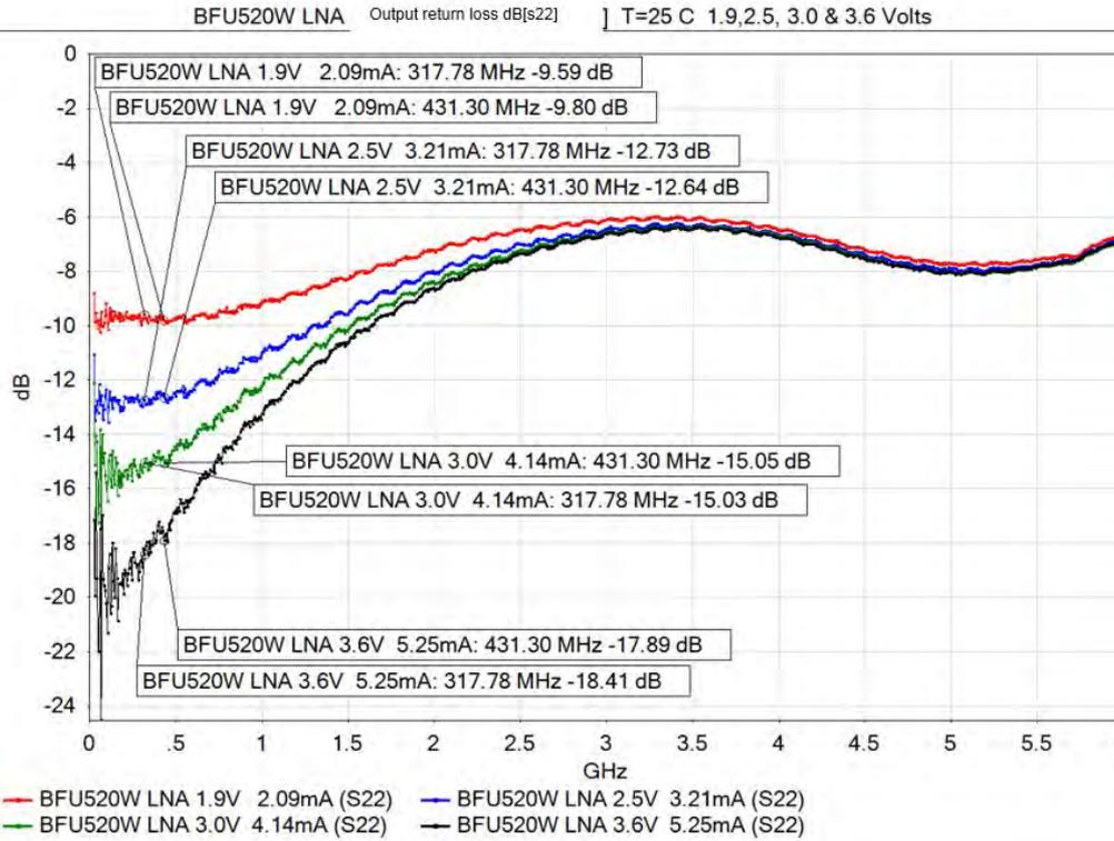
Fig 27. Output Return Loss vs Battery Voltage for a “Type 2” BFU520W RKE LNA, for 25 MHz – 6 GHz.
