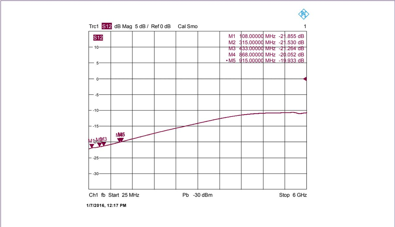
Fig 16. BFU520W “Type 1” RKE LNA, Reverse Isolation
