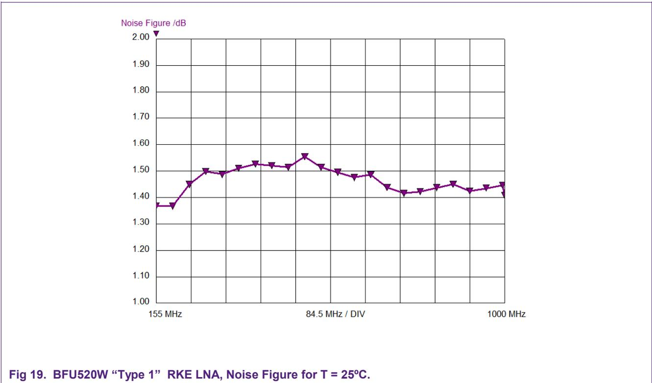
Fig 19. BFU520W “Type 1” RKE LNA, Noise Figure for T = 25°C.
