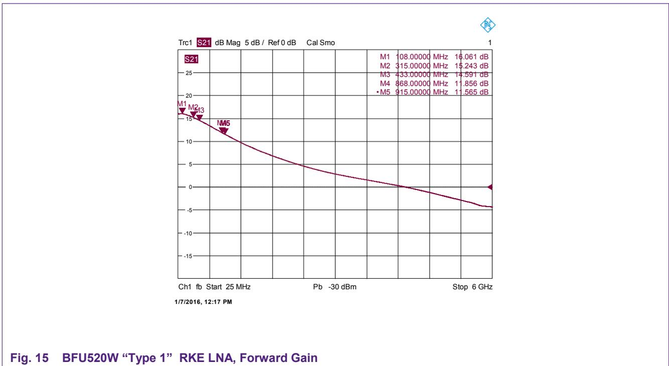
Fig. 15 BFU520W “Type 1” RKE LNA, Forward Gain
