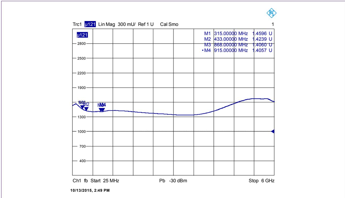
Fig 29. Stability factor  $\mu_1$  at 2.5 volts, “Type 2” BFU520W RKE LNA, for 25 MHz – 6 GHz.
