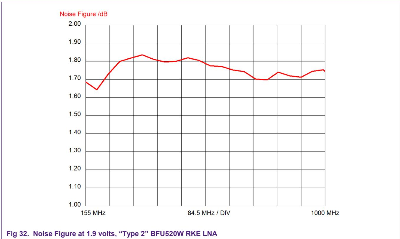
Fig 32. Noise Figure at 1.9 volts, “Type 2” BFU520W RKE LNA
