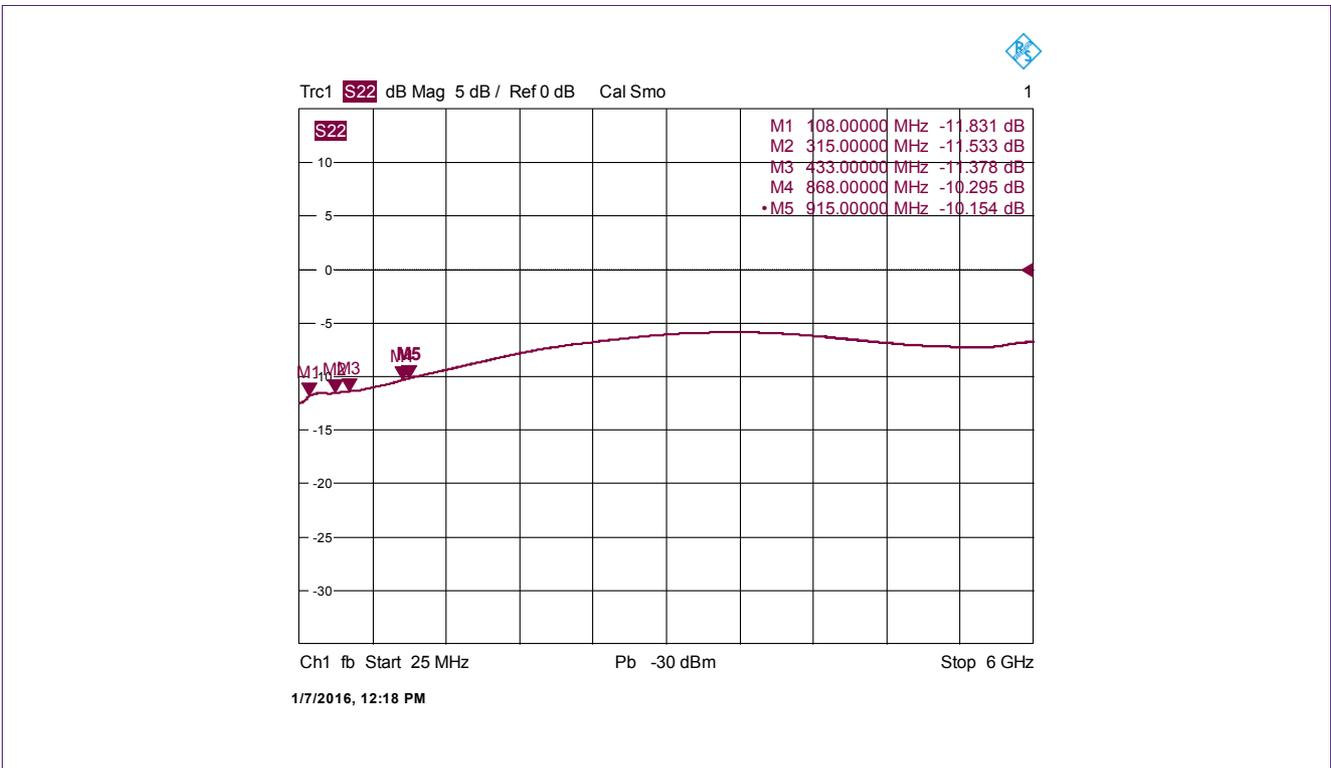
Fig 17. BFU520W “Type 1” RKE LNA, Output Return Loss. Note broadband / wideband matching.
