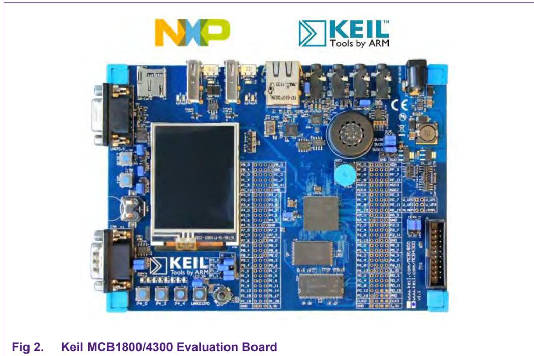
Fig 2. Keil MCB1800/4300 Evaluation Board
