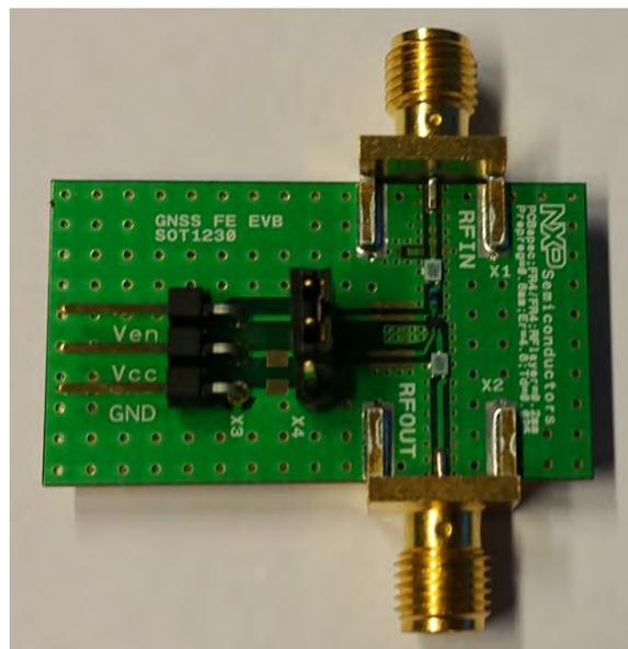
Fig 1. BGU8019 GNSS front-end evaluation board
