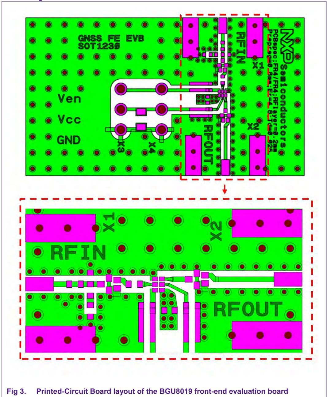
Fig 3. Printed-Circuit Board layout of the BGU8019 front-end evaluation board
