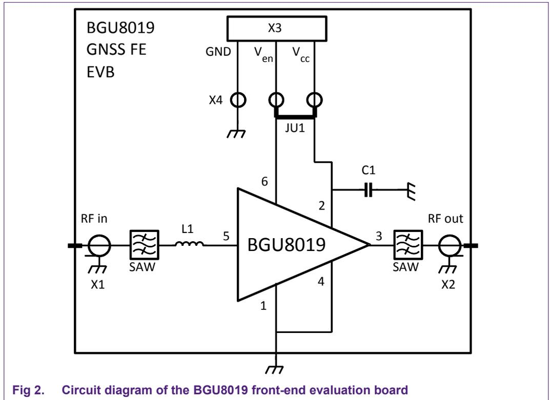
Fig 2. Circuit diagram of the BGU8019 front-end evaluation board
