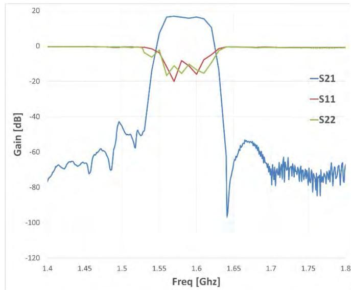
Fig 8. Typical pass band response at Vcc = 2.85 V
