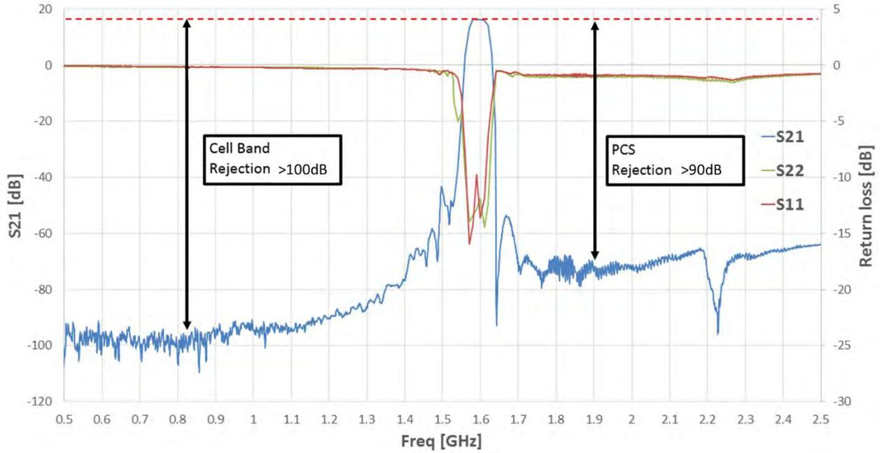
Fig 7. Typical S-parameter plot at Vcc = 2.85 V
