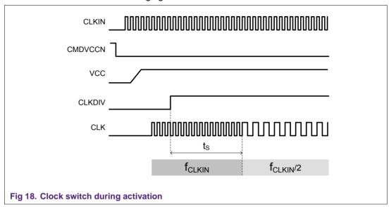
The clock starts with the value specified at activation. Then the clock frequency switch occurs after a maximum of 4 CLKIN periods after a change is seen on CLKDIV ( $t_s < t_{smax} = 4$  clock cycles).
