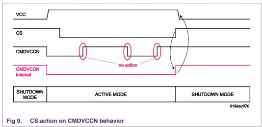
The signal CMDVCCN Internal represents the value that is seen by the TDA8037: the value is latched as soon as CS goes low, and can only change after CS goes back high.
