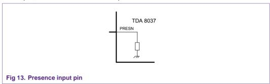
The way to connect the switch of a smart card connector depends on its gender (normally open or normally closed).
