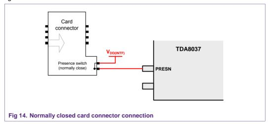
When the card is not inserted, the switch is closed, and the PRESN pin is not active and the card is assumed to be absent.
