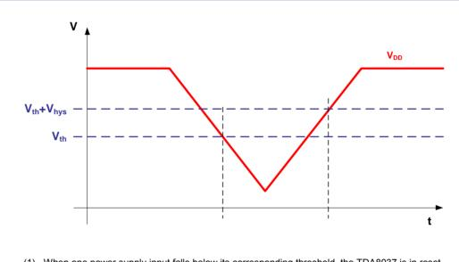
(1) When one power supply input falls below its corresponding threshold, the TDA8037 is in reset mode. When all the levels are above their threshold + the hysteresis, the TDA8037 is ON.
