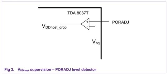
The TDA8037 compares the pin voltage level on pin PORADJ to an internal Reference voltage called Vbg (for Bandgap voltage).
