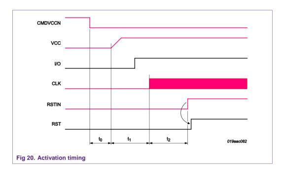
$t_{\text{0}}$  is the time between CMDVcc High and the start of the rise of Vcc. It lasts around 50  $\mu s$ .
