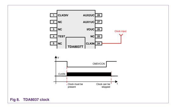
The clock frequency can be managed by the host on CLKIN. On the TDA8037T, CLKDIV can also be used to switch the frequency. However on the TDA8037T, be sure the <a href="CLKDIV">CLKDIV</a> pin is set to <a href="Iow level">low level</a> before changing the frequency on CLKIN.
