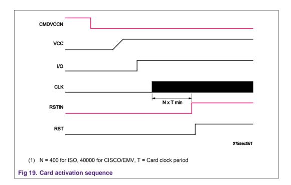
The input clock must be OK for this sequence to occur. As the clock is supplied externally, the clock must be present and stable before the falling edge of CMDVCCN.
