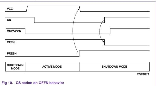
This shows that when the card is removed (or by extension when any fault is detected), the TDA automatically deactivate the card, in order to protect it.
