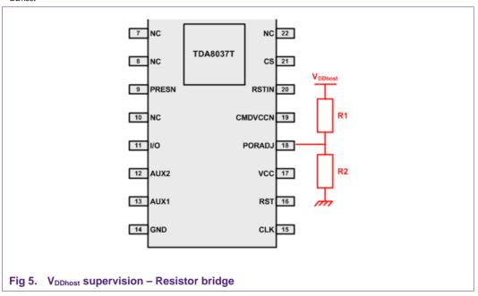
In this case  $V_{PORADJ} = V_{DDhost}.R2/(R1+R2)$  and  $V_{DDhost}$  is monitored indirectly: the TDA8037 enters the reset mode when  $V_{DDhost}.R2/(R1 + R2)$  falls below  $V_{ba}$ .
