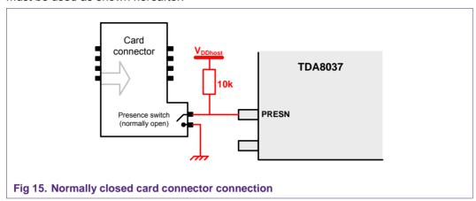
When the card is not inserted, the switch is open and PRESN is pulled-up to HIGH level. The pin is not active so the card is seen as absent.
