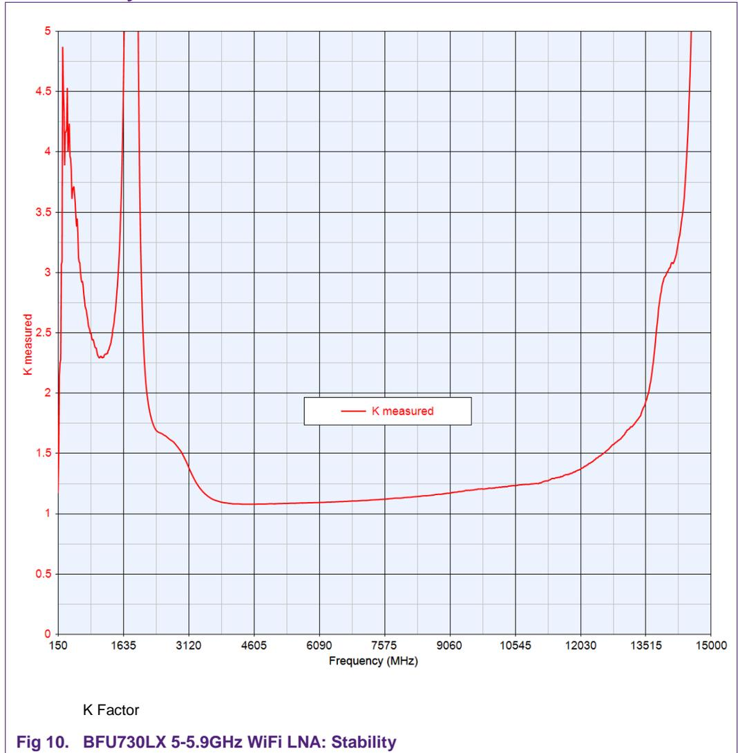
Fig 10. BFU730LX 5-5.9GHz WiFi LNA: Stability
