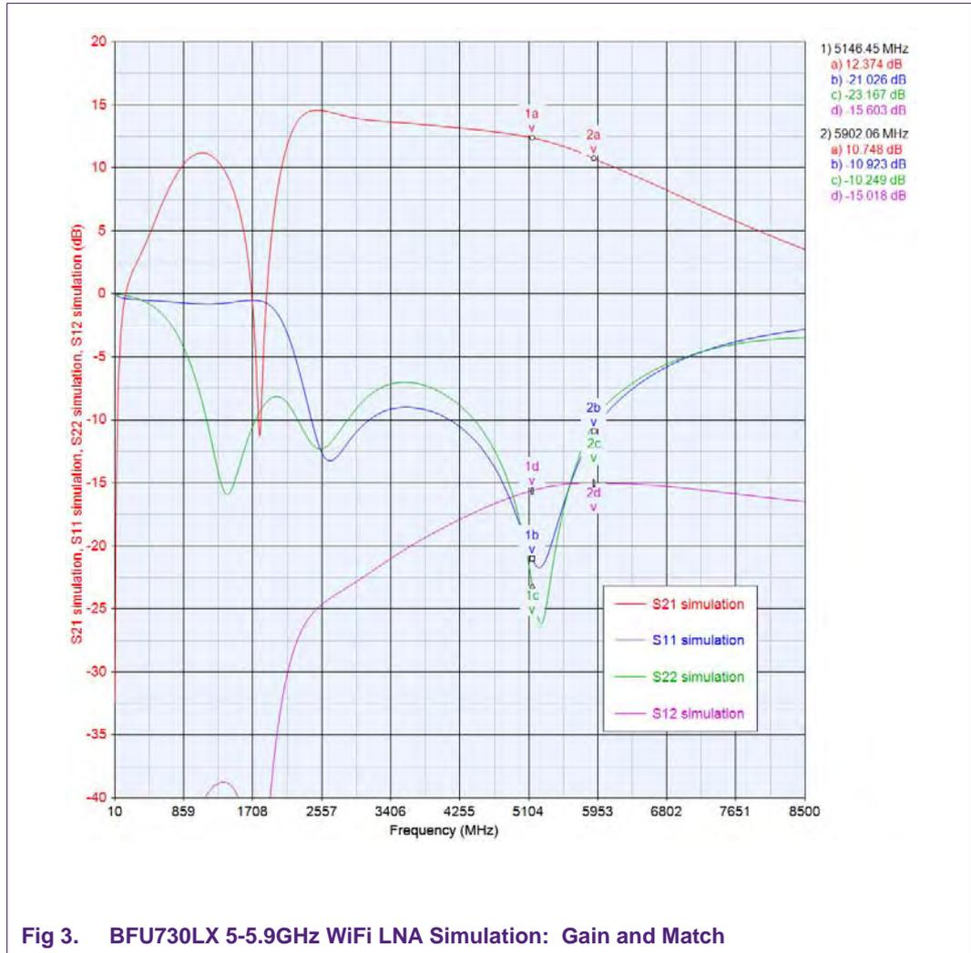
Fig 3. BFU730LX 5-5.9GHz WiFi LNA Simulation: Gain and Match
