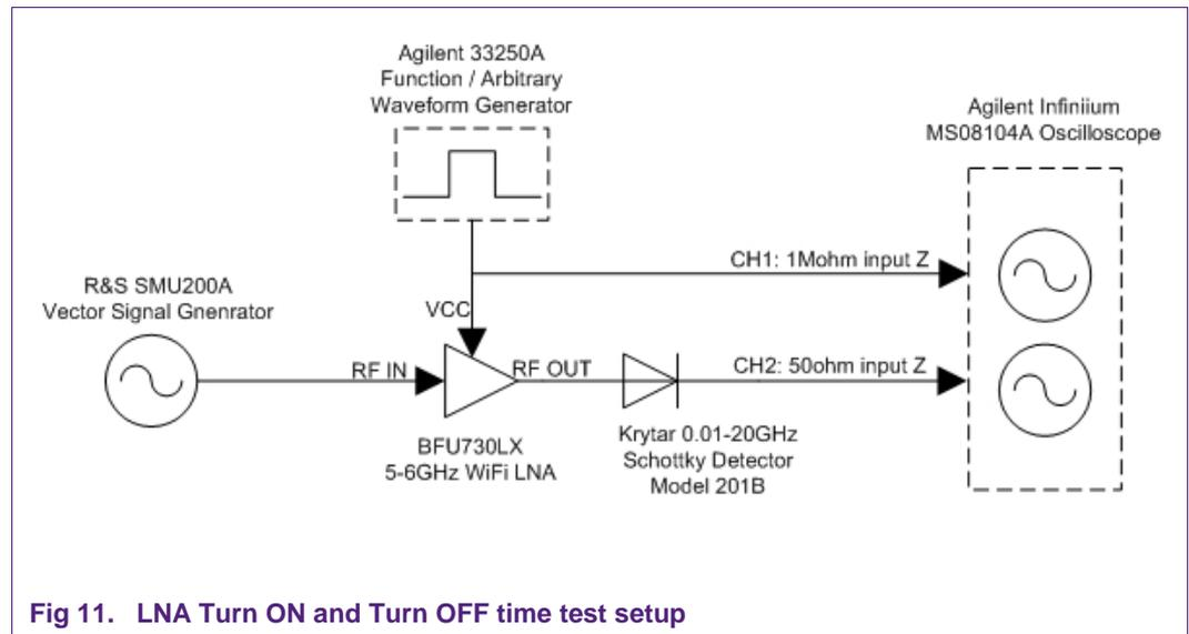
Fig 11. LNA Turn ON and Turn OFF time test setup
