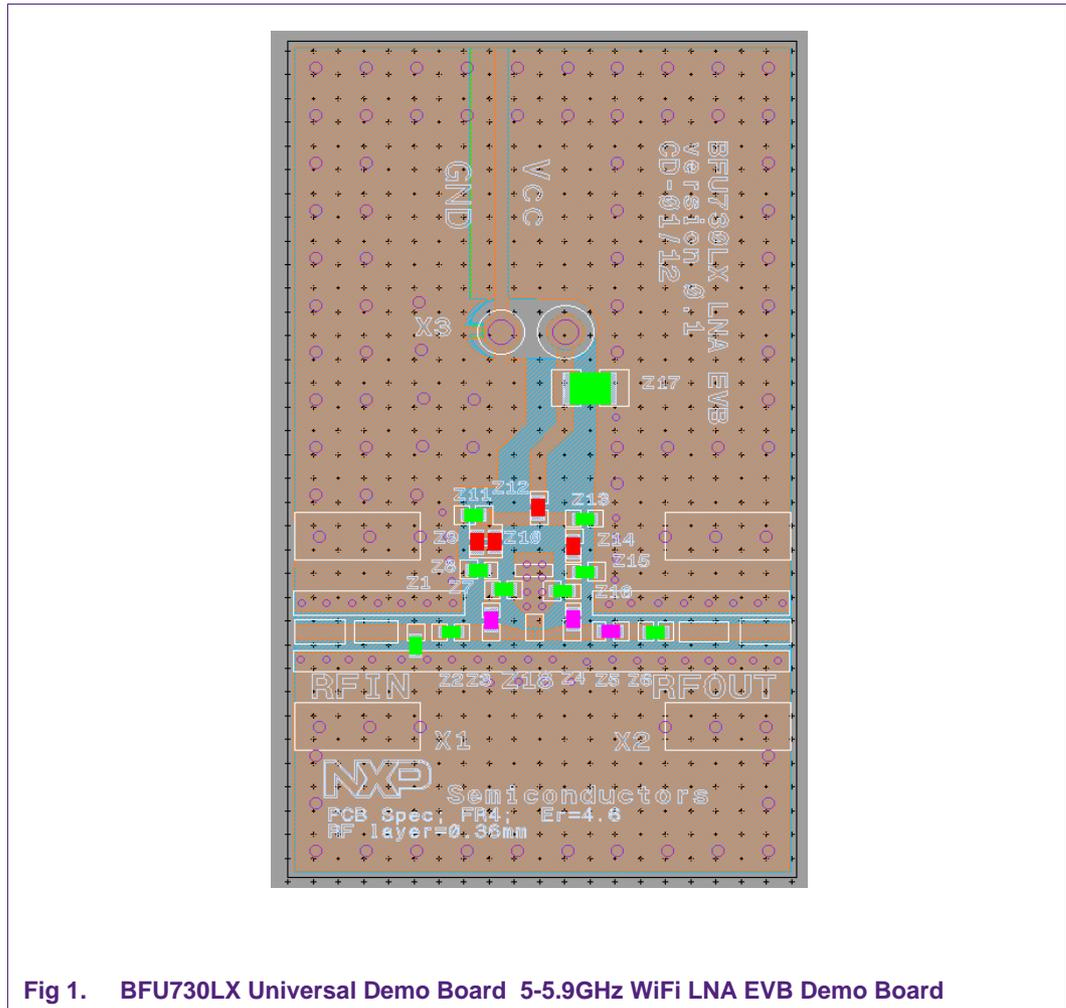
Fig 1. BFU730LX Universal Demo Board 5-5.9GHz WiFi LNA EVB Demo Board
