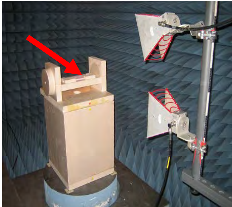
Fig 2. Measurement Setup: Anechoic chamber
