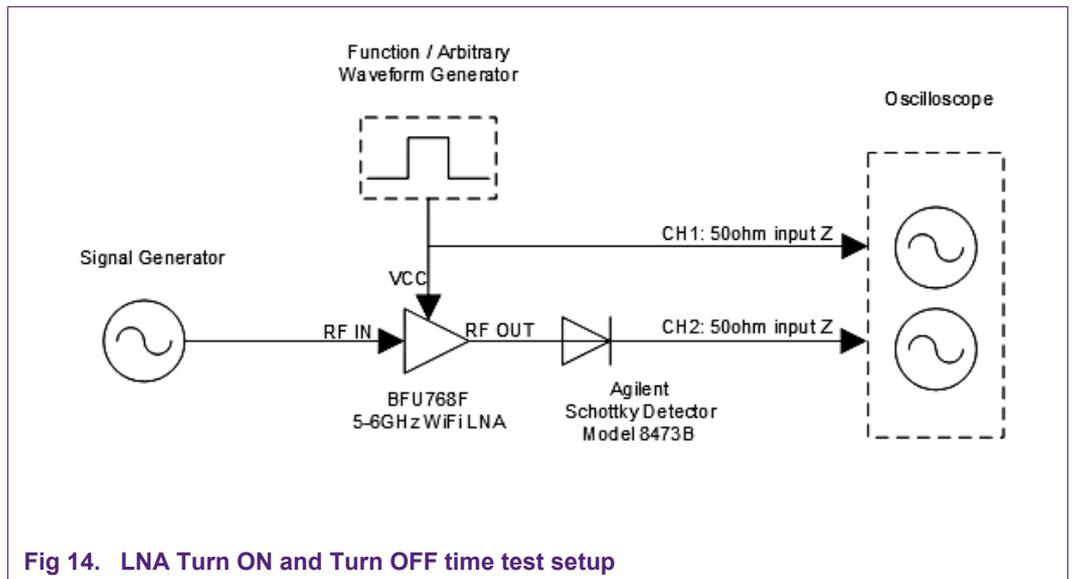
Fig 14. LNA Turn ON and Turn OFF time test setup
