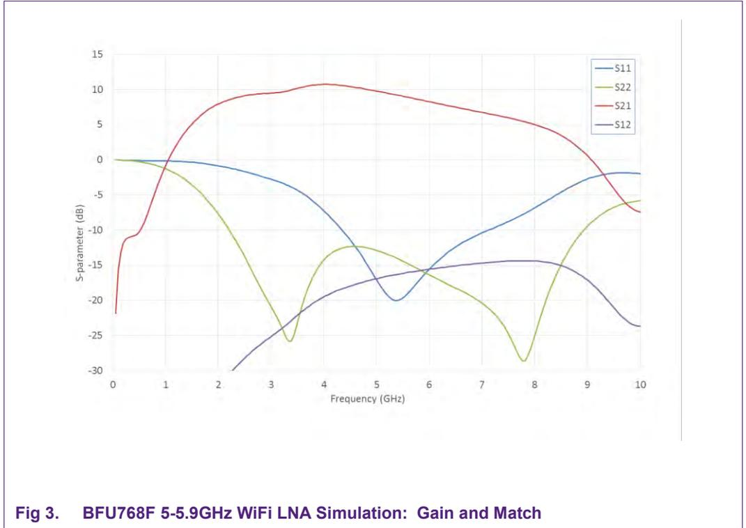
Fig 3. BFU768F 5-5.9GHz WiFi LNA Simulation: Gain and Match
