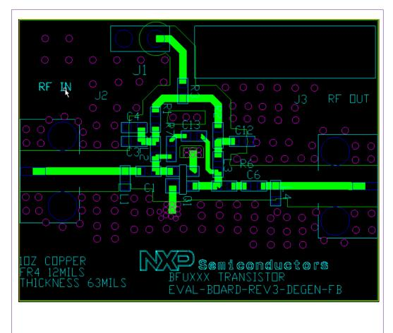
Fig 1. BFUXXX Universal Demo Board/BFU730F 2.4-2.5GHz WiFi LNA EVB Demo Board
