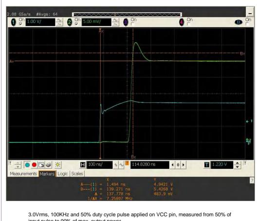
input pulse to 90% of max. output power
