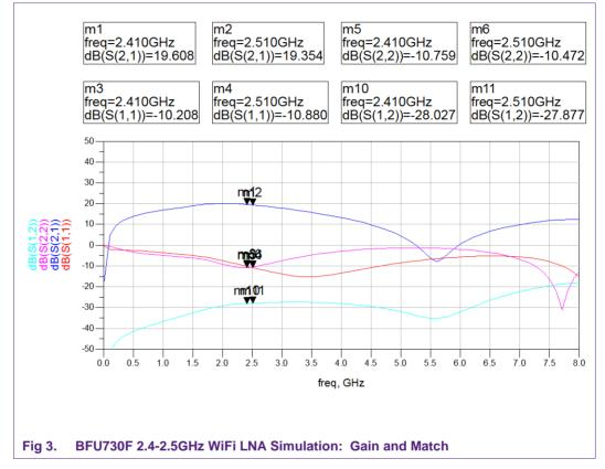
Low Noise Fast Turn ON/OFF 2.4-2.5GHz WiFi LNA with BFU730F
