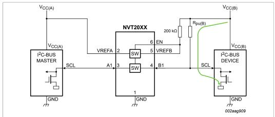
Figure 7. Current path through NVT20xx when B-side driver is turned on and  $V_{CC(B)}$  -  $V_{CC(A)} \ge 1 \text{ V}$
