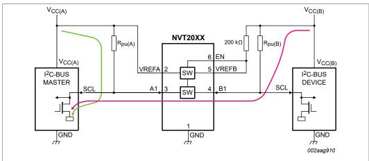
Figure 8. Current path through NVT20xx when A-side driver is driven LOW and  $V_{\text{CC}(B)}$  -  $V_{\text{CC}(A)}$  < 1 V
