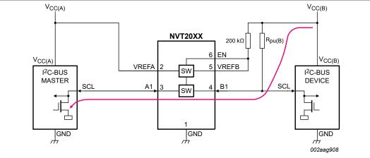
Figure 6. Current path through NVT20xx when A-side driver is turned on and  $V_{CC(B)}$  -  $V_{CC(A)} \ge 1 \text{ V}$
