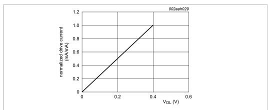
Figure 5. Derating curve for normalized drive current versus  $V_{\text{OL}}$ , when  $V_{\text{OL}}$  is specified at 0.4 V
