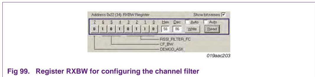
**Fig 99. Register RXBW for configuring the channel filter**
