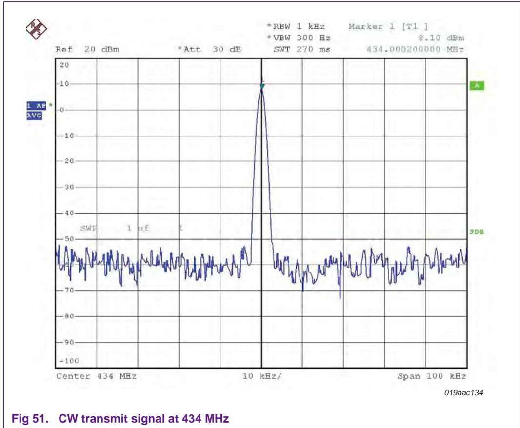
Fig 51. CW transmit signal at 434 MHz
