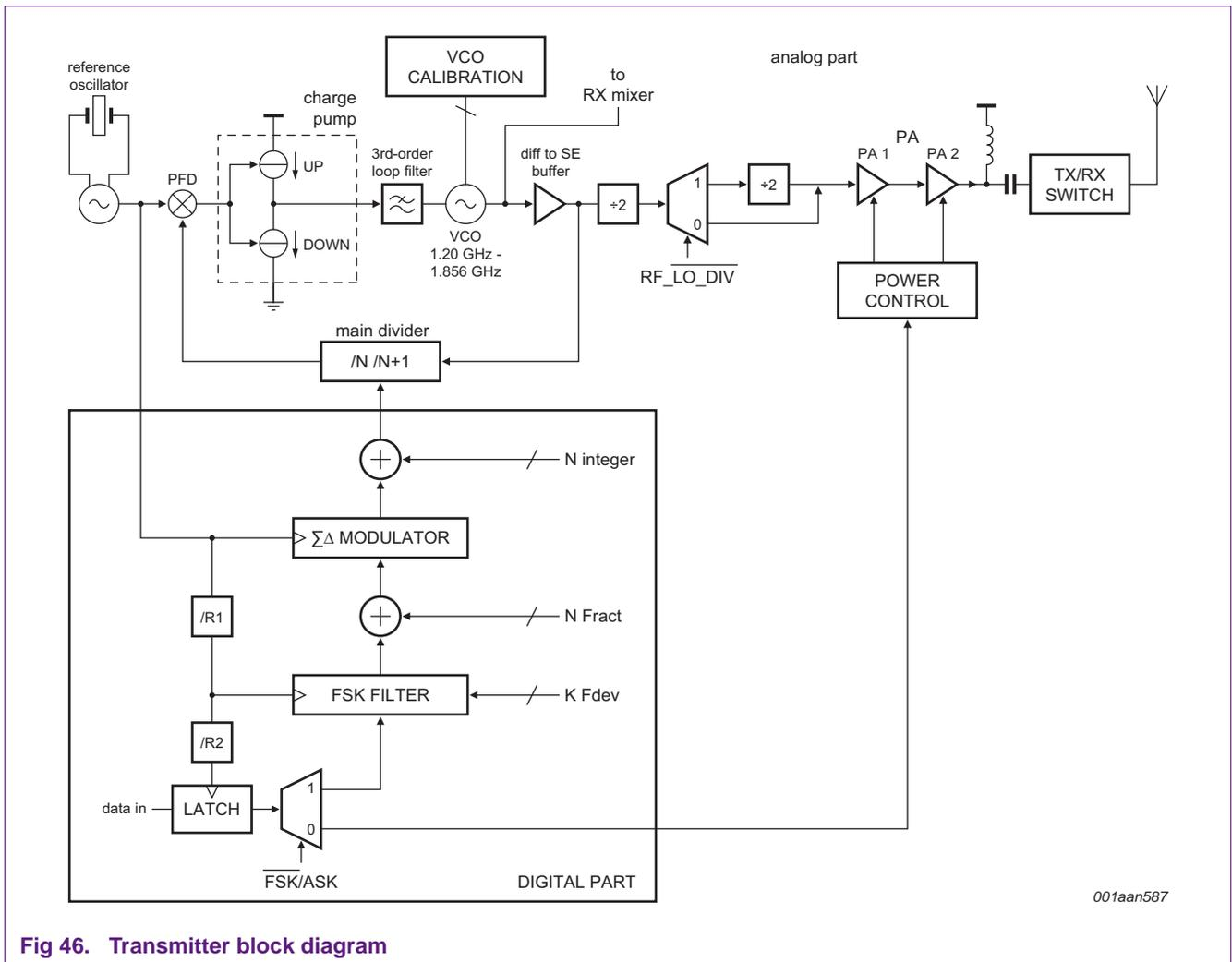
Fig 46. Transmitter block diagram
