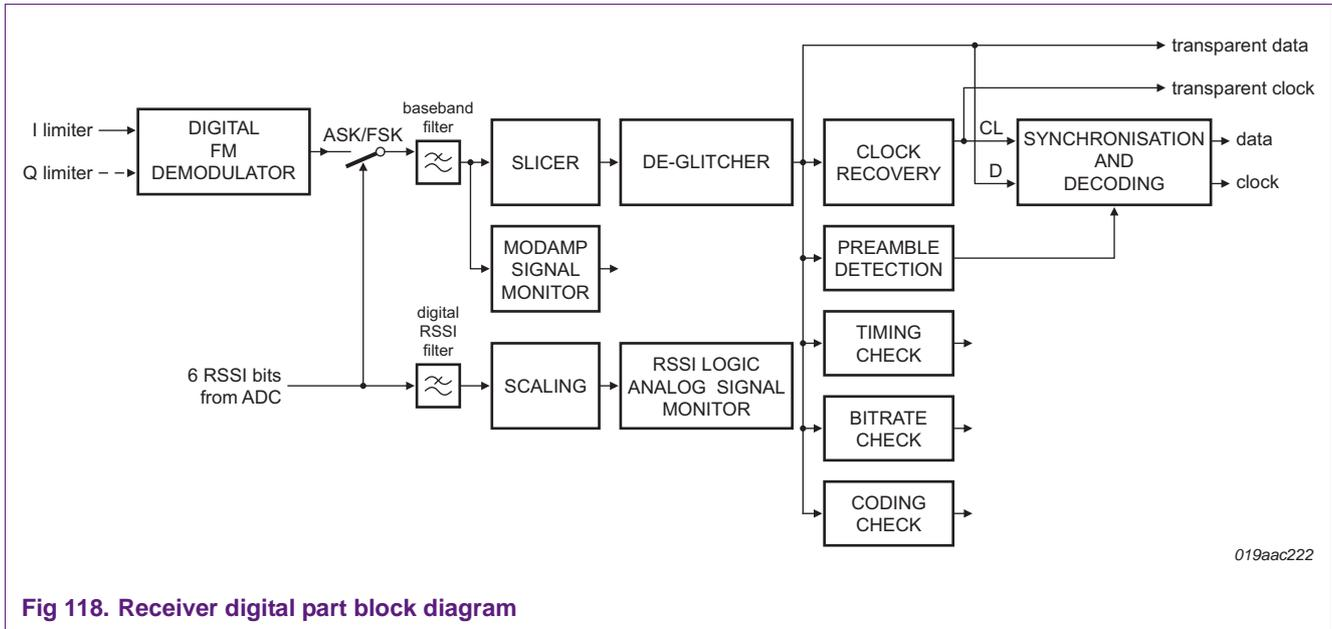
Fig 118. Receiver digital part block diagram
