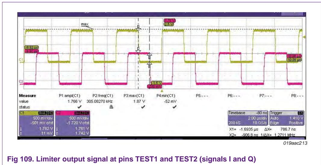
Fig 109. Limiter output signal at pins TEST1 and TEST2 (signals I and Q)
