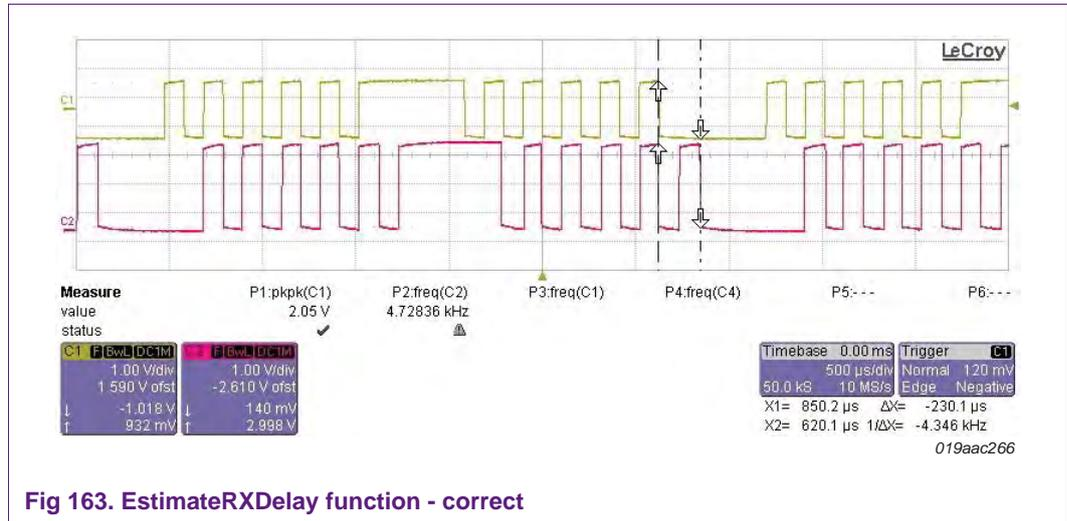
Fig 163. EstimateRXDelay function - correct
