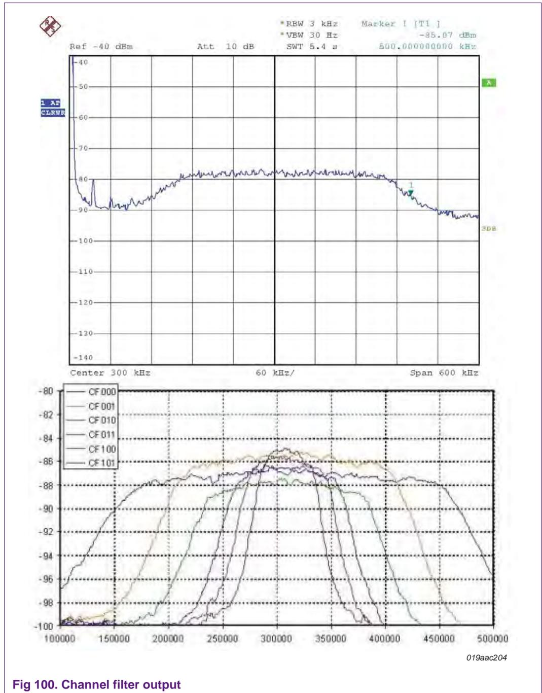
Fig 100. Channel filter output
