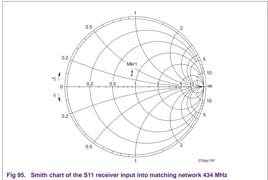
**Fig 95. Smith chart of the S11 receiver input into matching network 434 MHz**
