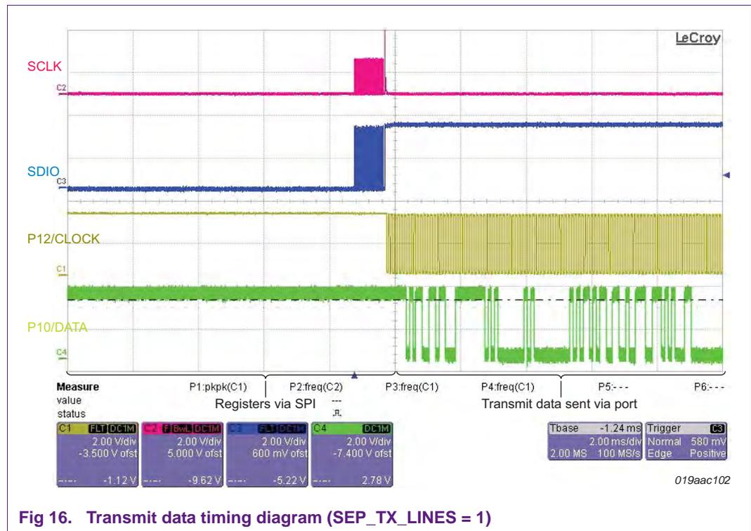
Fig 16. Transmit data timing diagram (SEP\_TX\_LINES = 1)
