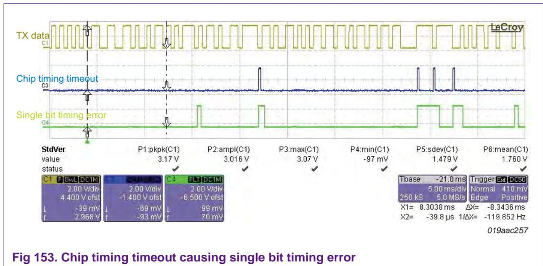
Fig 153. Chip timing timeout causing single bit timing error
