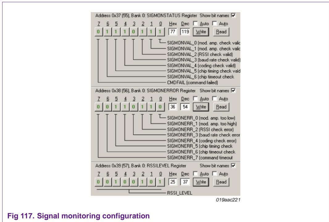
Fig 117. Signal monitoring configuration
