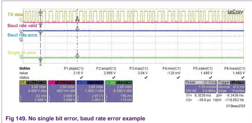
Fig 149. No single bit error, baud rate error example
