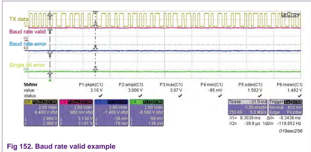
Fig 152. Baud rate valid example
