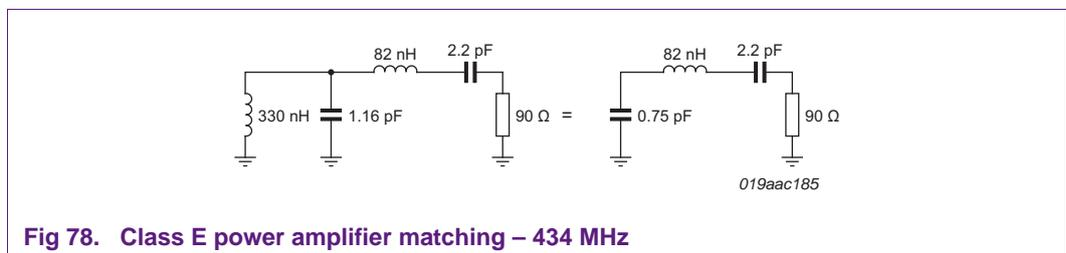
Fig 78. Class E power amplifier matching – 434 MHz
