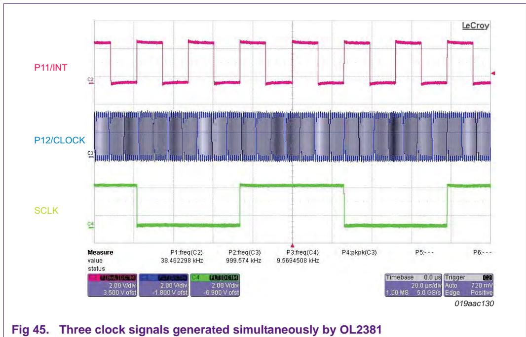
Fig 45. Three clock signals generated simultaneously by OL2381
