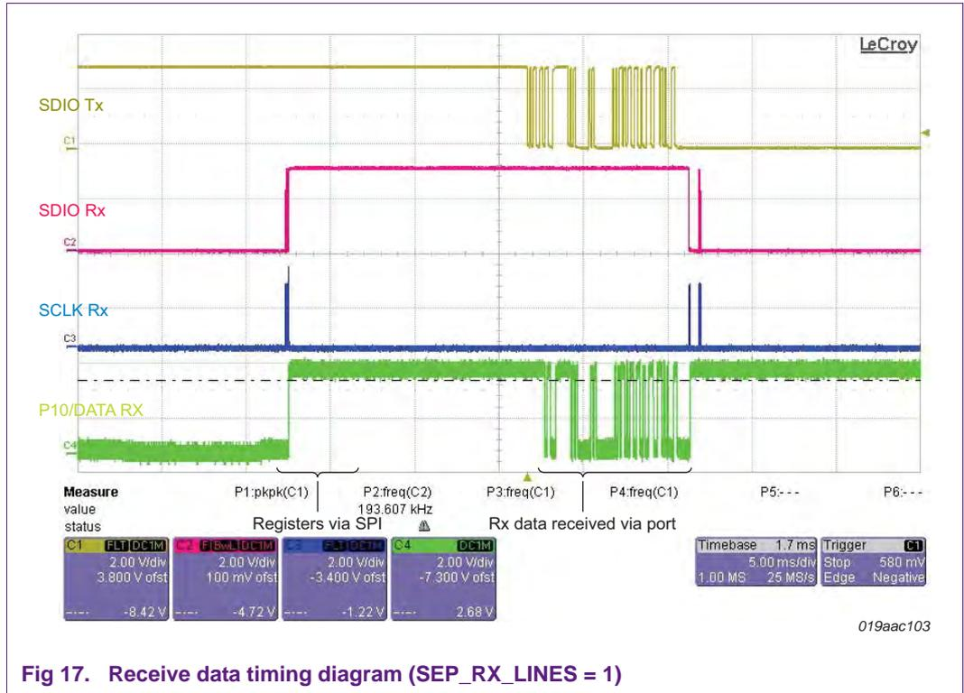
Fig 17. Receive data timing diagram (SEP\_RX\_LINES = 1)
