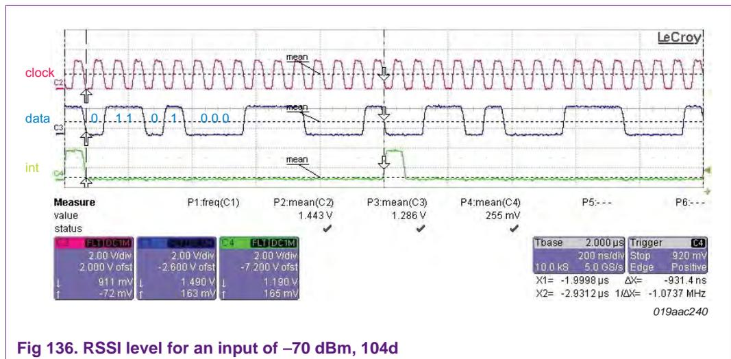
**Fig 136. RSSI level for an input of -70 dBm, 104d**
