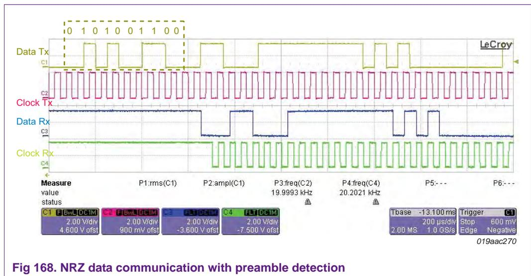
Fig 168. NRZ data communication with preamble detection
