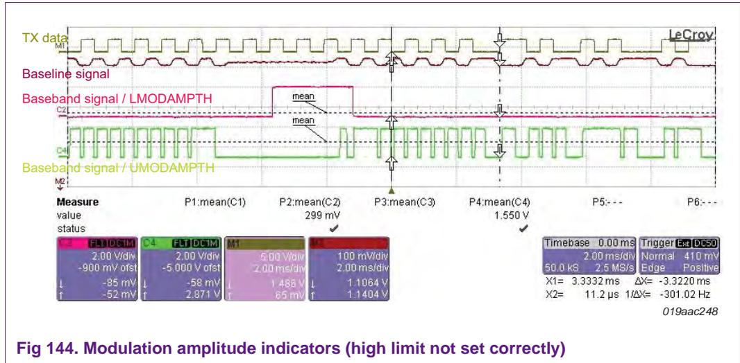
Fig 144. Modulation amplitude indicators (high limit not set correctly)
