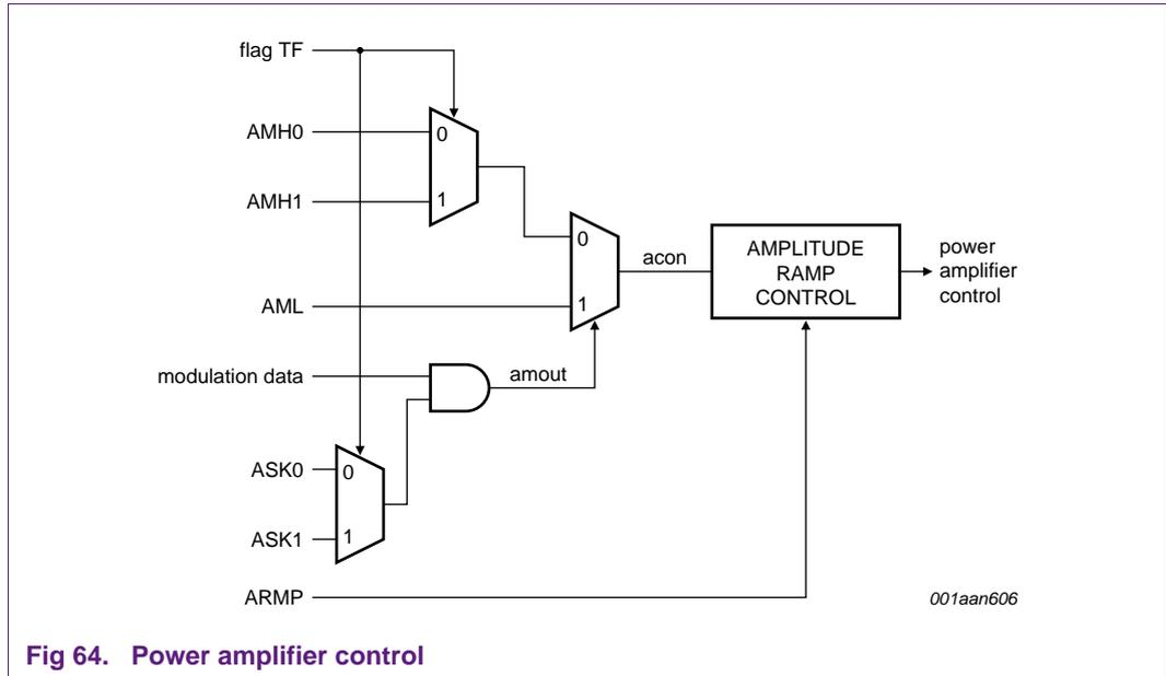
Fig 64. Power amplifier control
