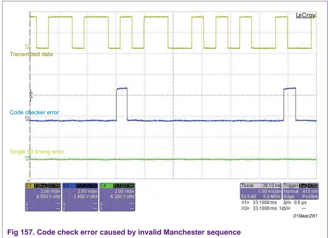
Fig 157. Code check error caused by invalid Manchester sequence
