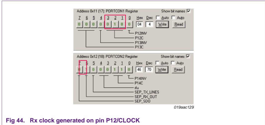
Fig 44. Rx clock generated on pin P12/CLOCK
