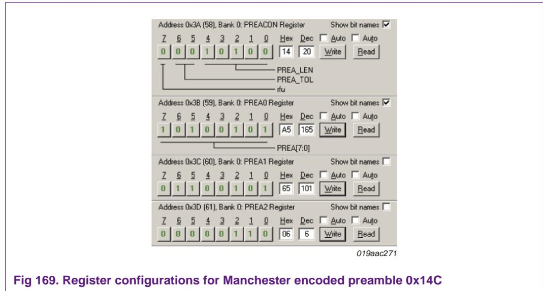
**Fig 169. Register configurations for Manchester encoded preamble 0x14C**
