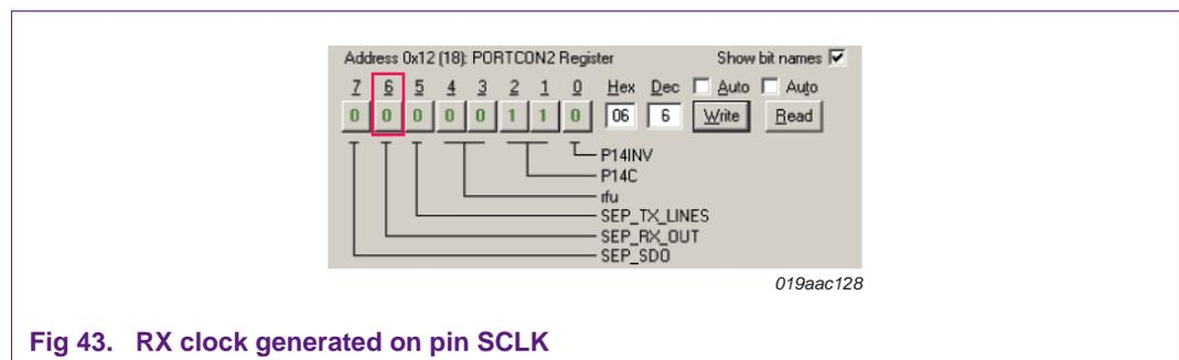
Fig 43. RX clock generated on pin SCLK
