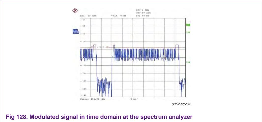
Fig 128. Modulated signal in time domain at the spectrum analyzer
