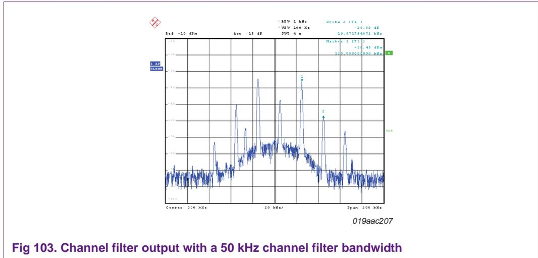
**Fig 103. Channel filter output with a 50 kHz channel filter bandwidth**
