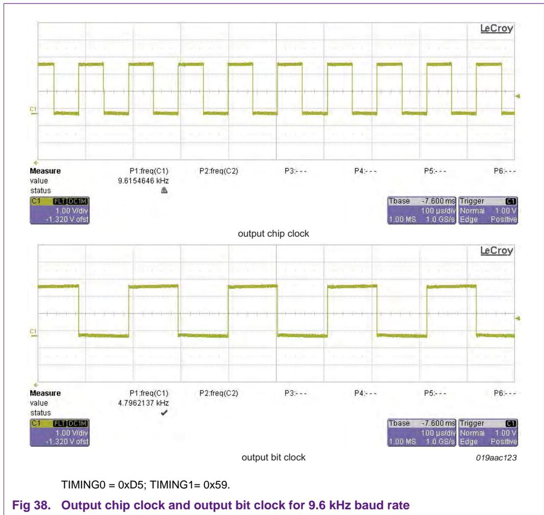
Fig 38. Output chip clock and output bit clock for 9.6 kHz baud rate
