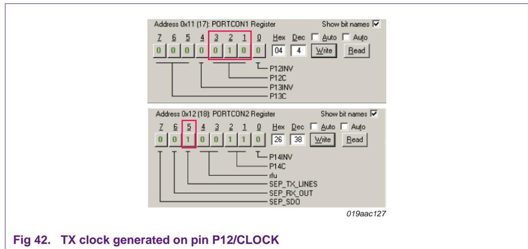
Fig 42. TX clock generated on pin P12/CLOCK
