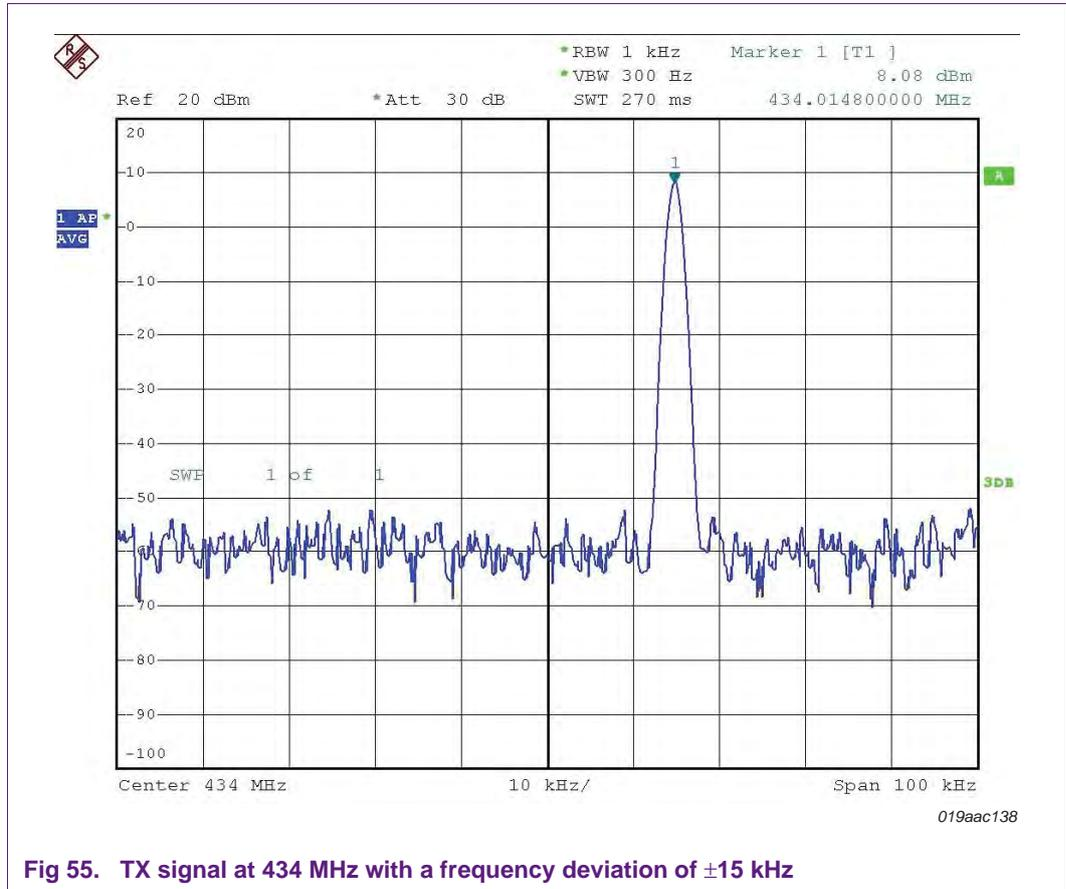
Fig 55. TX signal at 434 MHz with a frequency deviation of ±15 kHz
