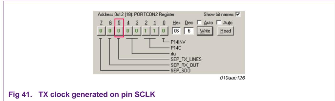
Fig 41. TX clock generated on pin SCLK
