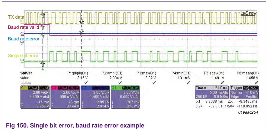
Fig 150. Single bit error, baud rate error example
