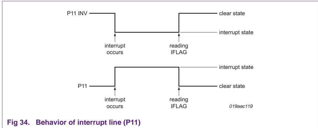
Fig 34. Behavior of interrupt line (P11)
