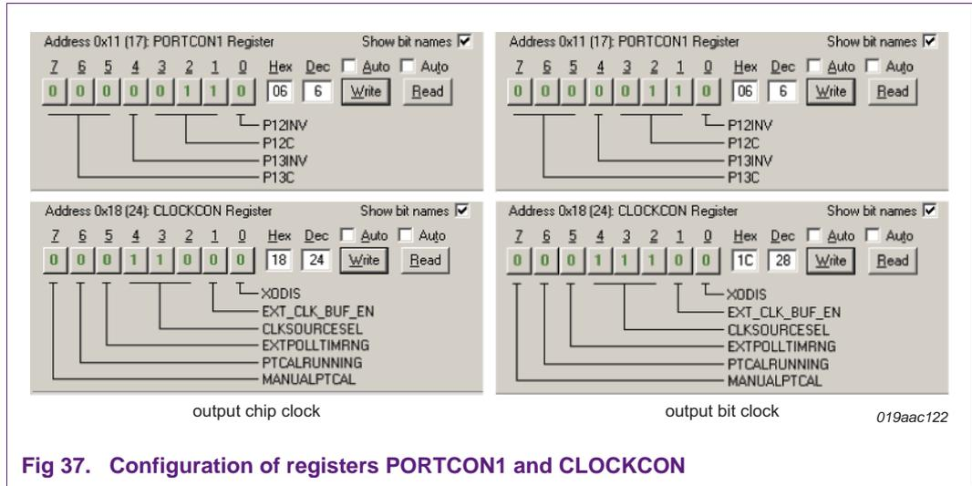
Fig 37. Configuration of registers PORTCON1 and CLOCKCON
