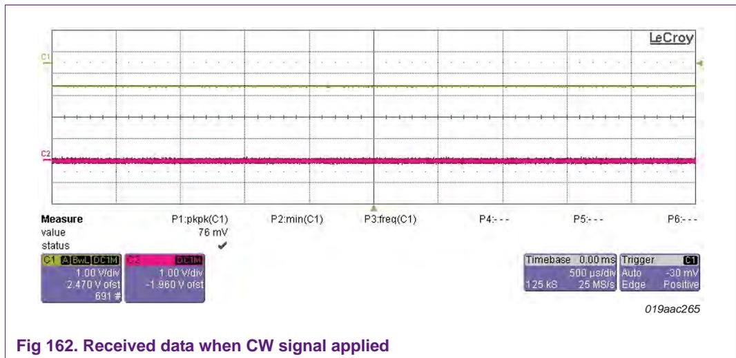
Fig 162. Received data when CW signal applied
