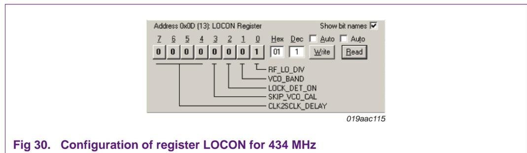
Fig 30. Configuration of register LOCON for 434 MHz
