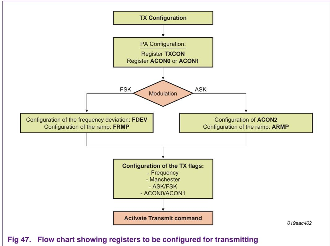
Fig 47. Flow chart showing registers to be configured for transmitting
