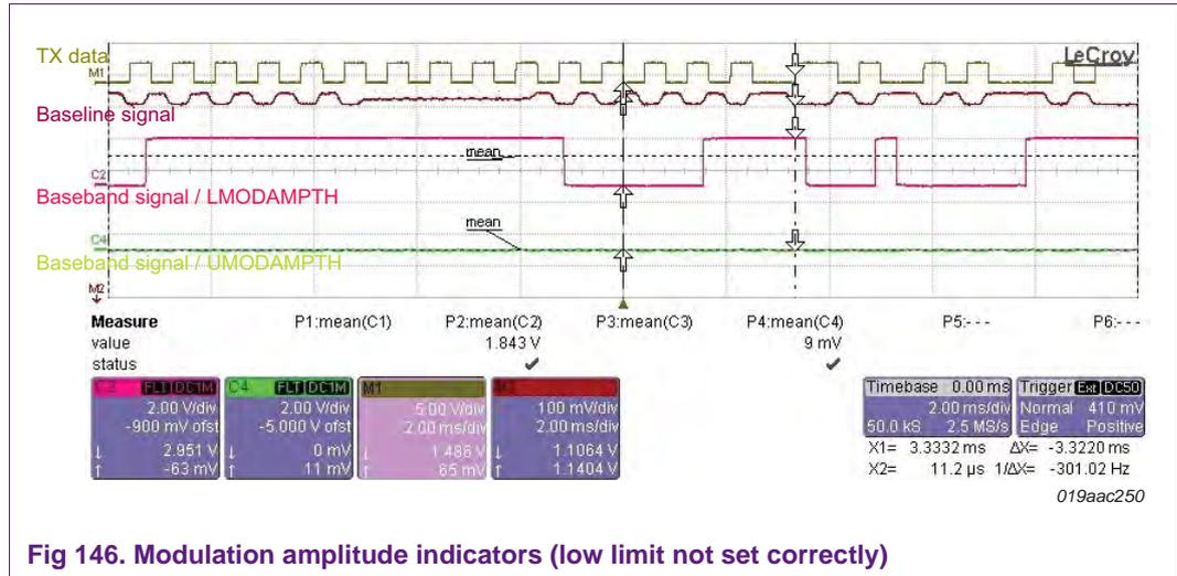
Fig 146. Modulation amplitude indicators (low limit not set correctly)
