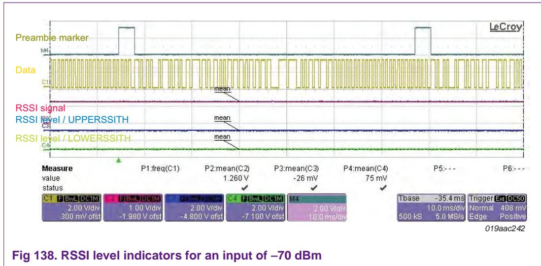
Fig 138. RSSI level indicators for an input of -70 dBm
