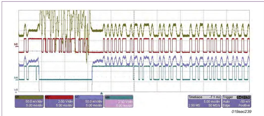
Fig 135. Baseband filter output and slicer output: interferer with 1 dB less power present
