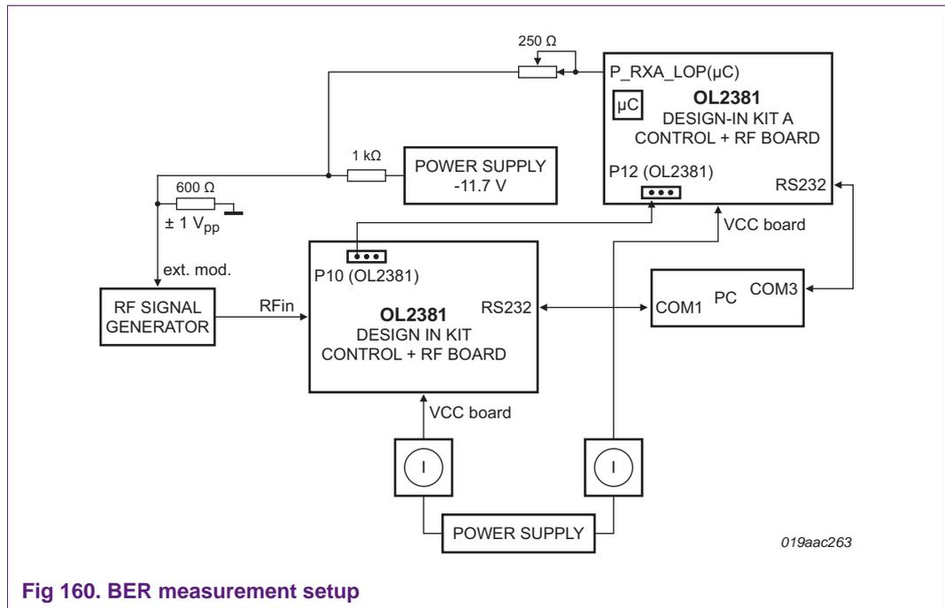
Fig 160. BER measurement setup
