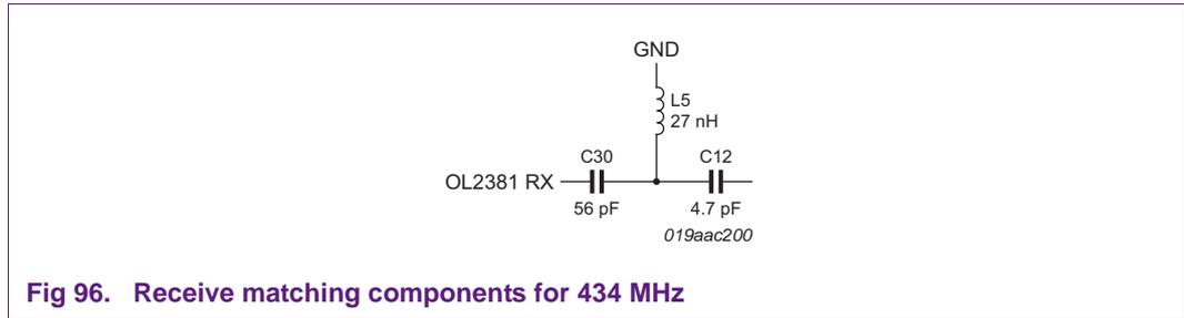
Fig 96. Receive matching components for 434 MHz
