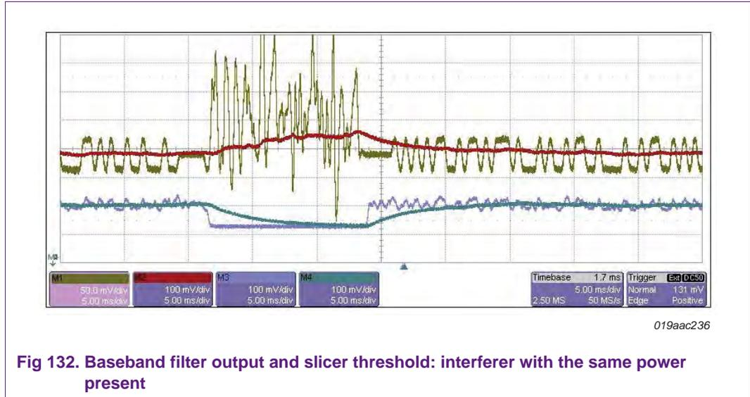
**Fig 132. Baseband filter output and slicer threshold: interferer with the same power present**
