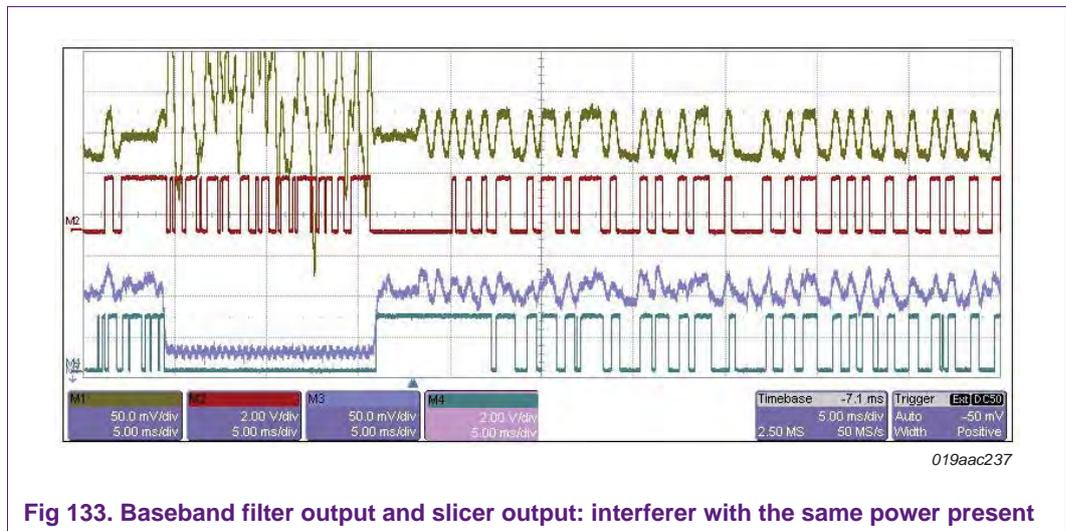
**Fig 133. Baseband filter output and slicer output: interferer with the same power present**
