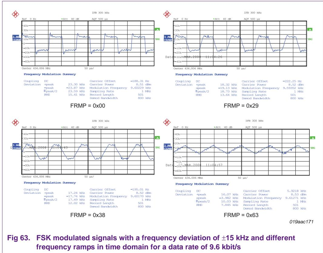
Fig 63. FSK modulated signals with a frequency deviation of ±15 kHz and different frequency ramps in time domain for a data rate of 9.6 kbit/s
