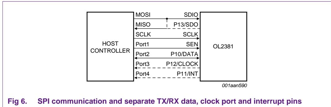
Fig 6. SPI communication and separate TX/RX data, clock port and interrupt pins
