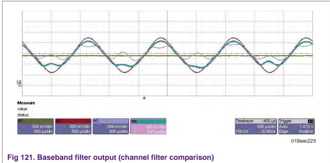
Fig 121. Baseband filter output (channel filter comparison)
