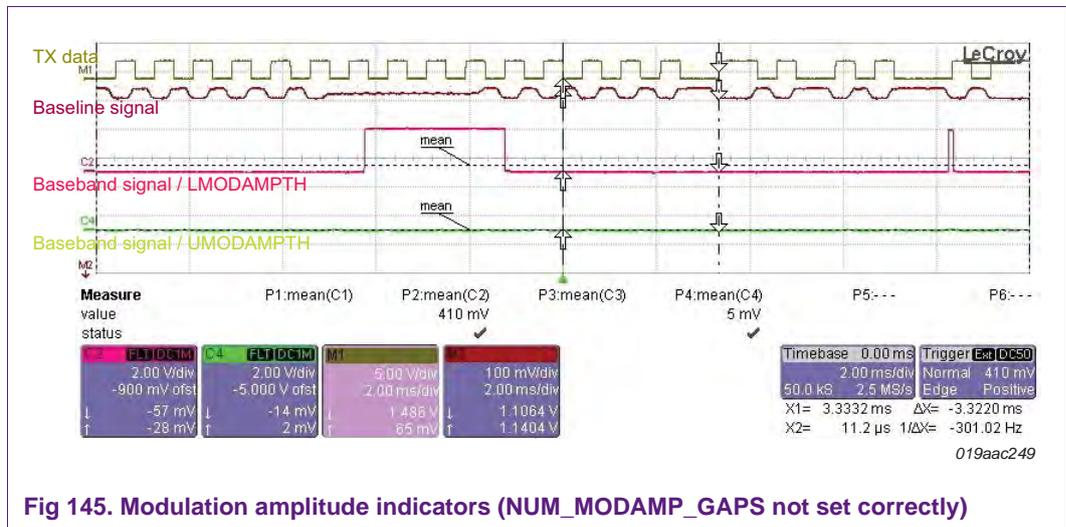
Fig 145. Modulation amplitude indicators (NUM\_MODAMP\_GAPS not set correctly)
