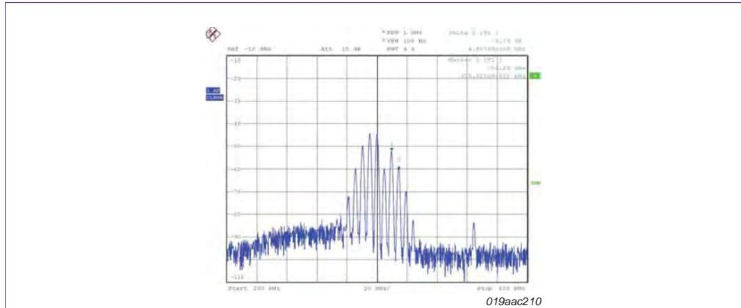
Fig 106. Channel filter output when RC calibration is omitted
