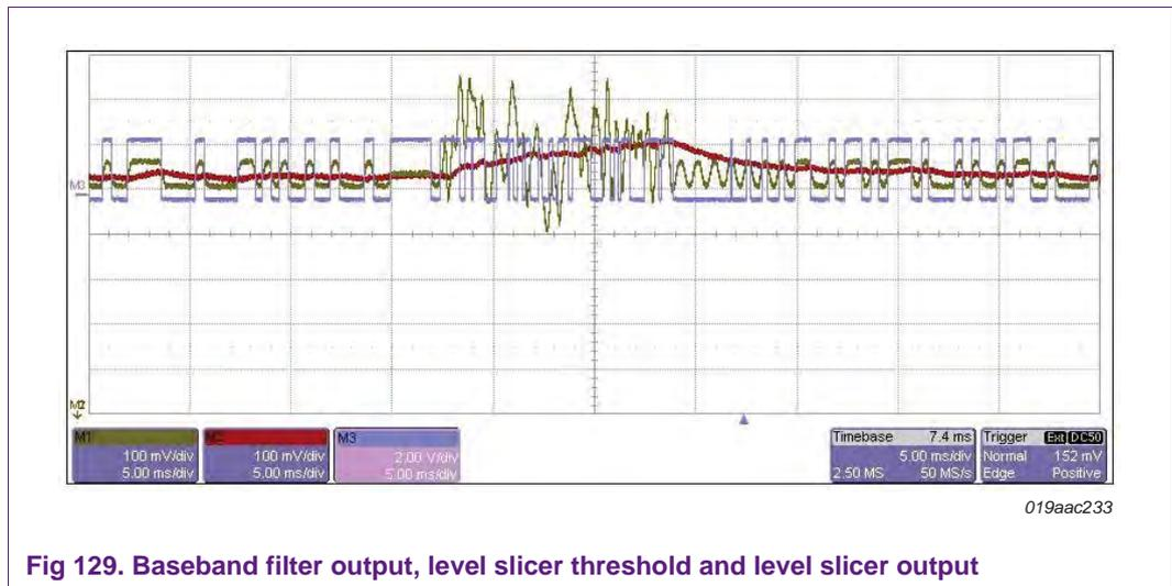
Fig 129. Baseband filter output, level slicer threshold and level slicer output
