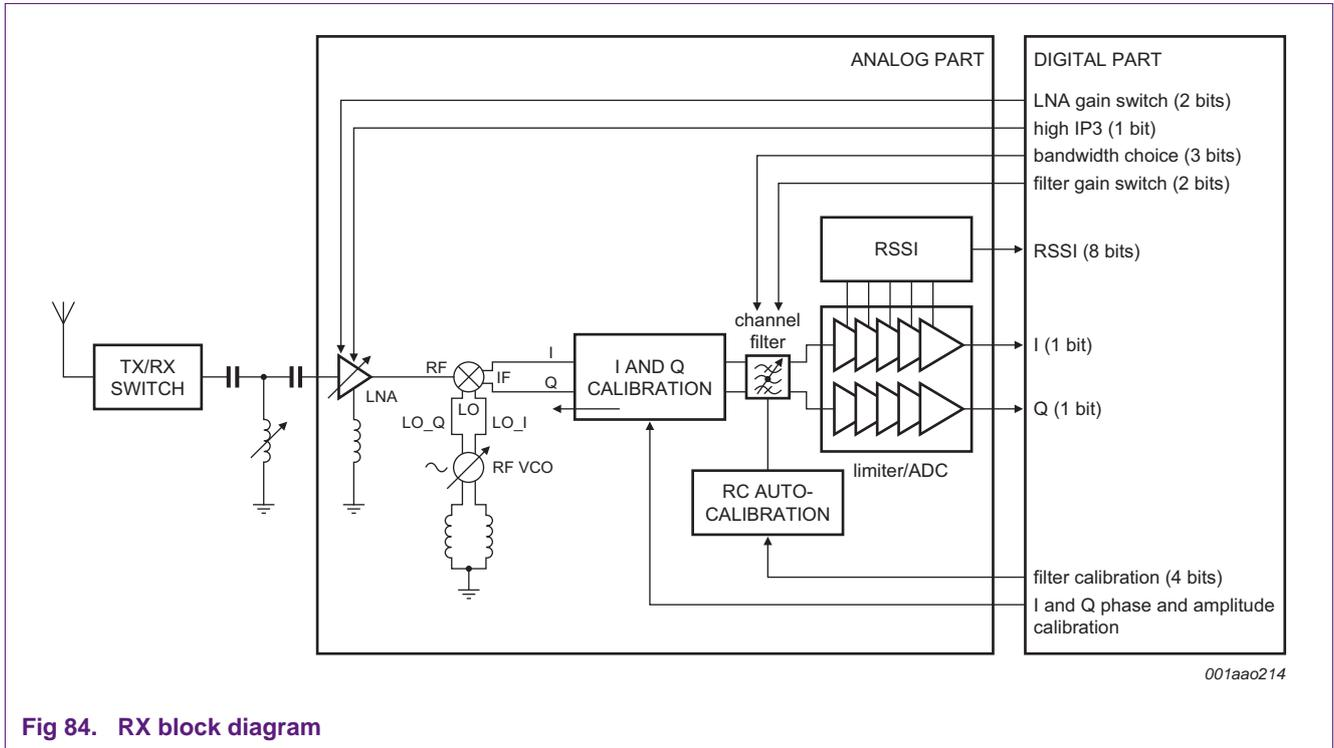
Fig 84. RX block diagram
