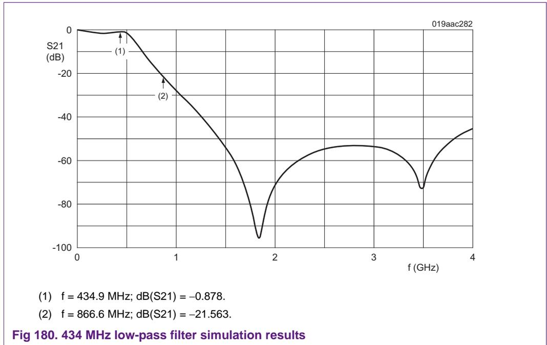
Fig 180. 434 MHz low-pass filter simulation results
