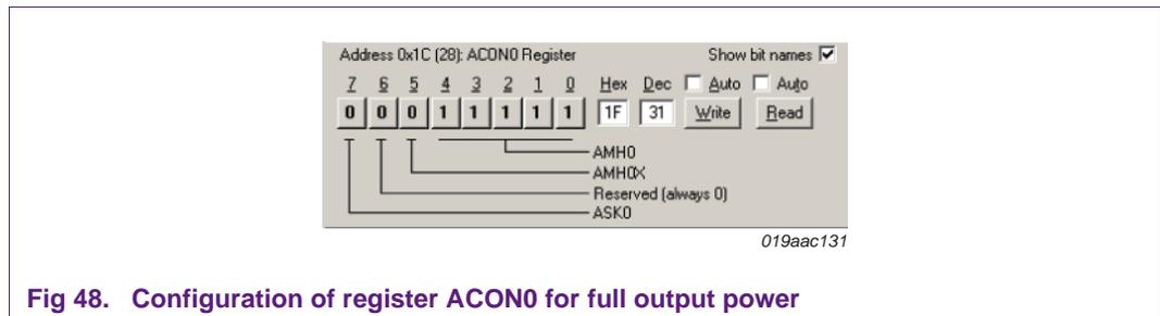
Fig 48. Configuration of register ACON0 for full output power
