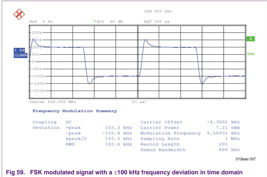
Fig 59. FSK modulated signal with a ±100 kHz frequency deviation in time domain
