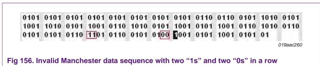
Fig 156. Invalid Manchester data sequence with two “1s” and two “0s” in a row
