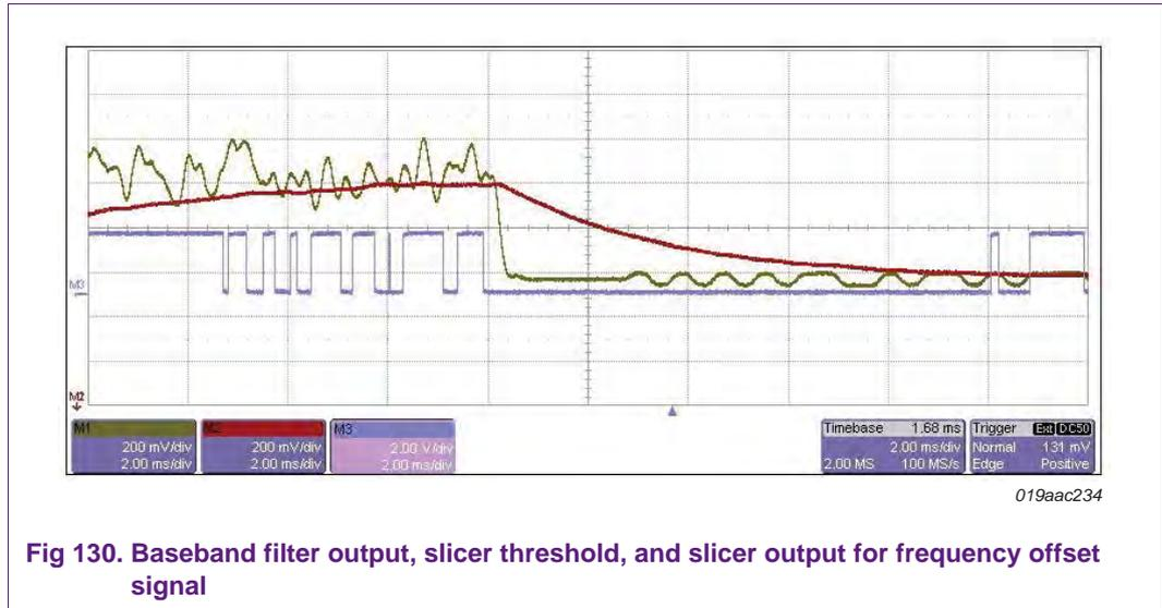
**Fig 130. Baseband filter output, slicer threshold, and slicer output for frequency offset signal**
