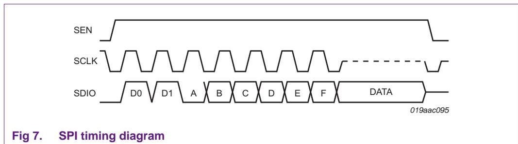
Fig 7. SPI timing diagram
