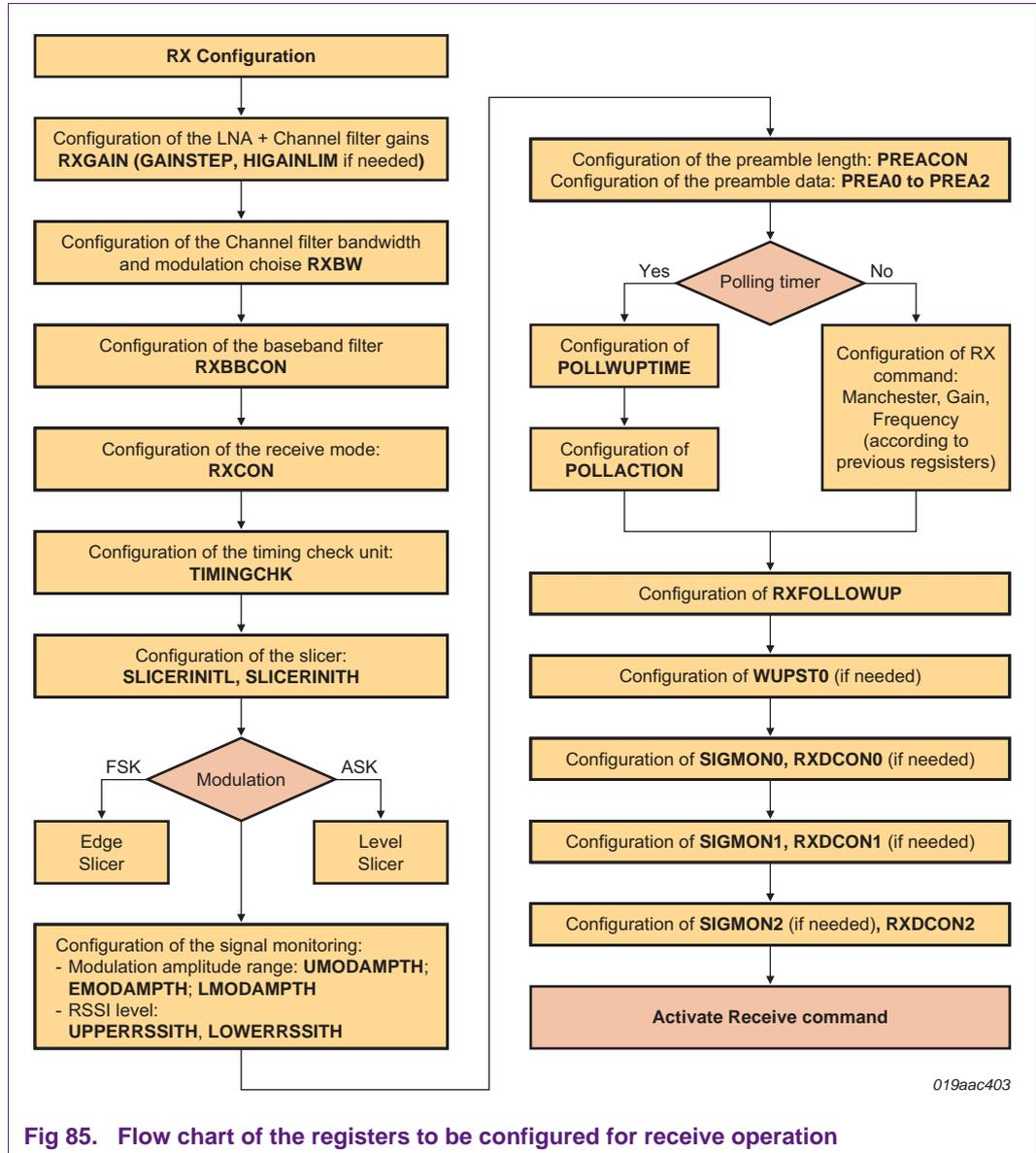
Fig 85. Flow chart of the registers to be configured for receive operation
