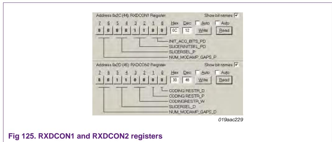
**Fig 125. RXDCON1 and RXDCON2 registers**
