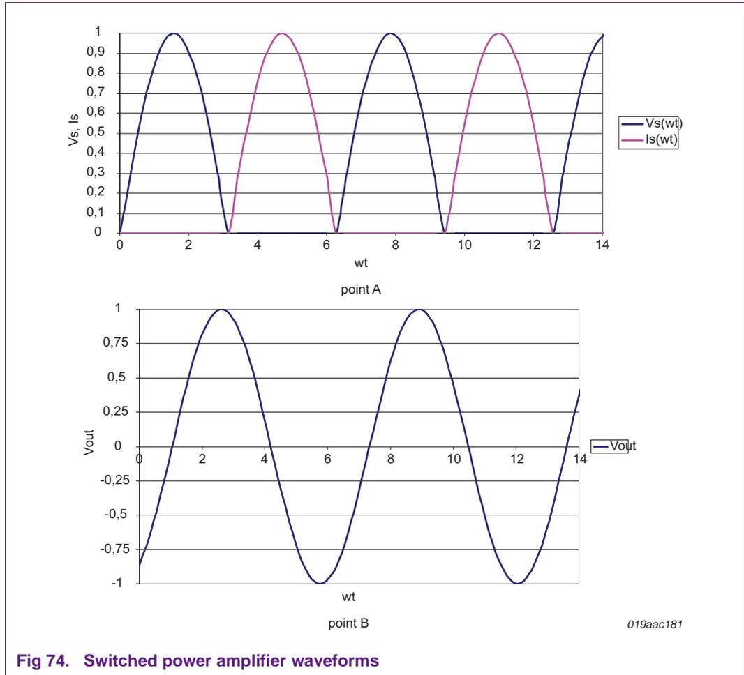
Fig 74. Switched power amplifier waveforms
