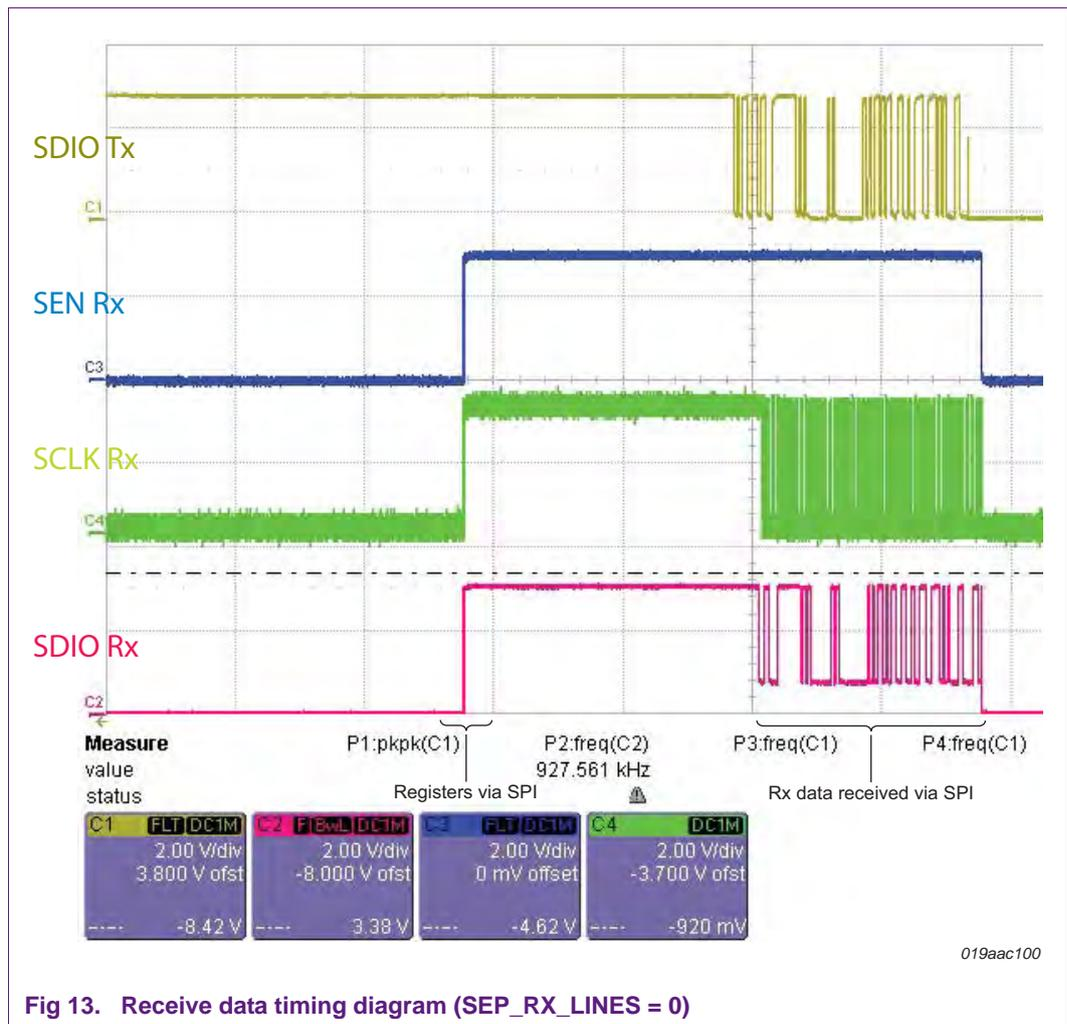
Fig 13. Receive data timing diagram (SEP\_RX\_LINES = 0)
