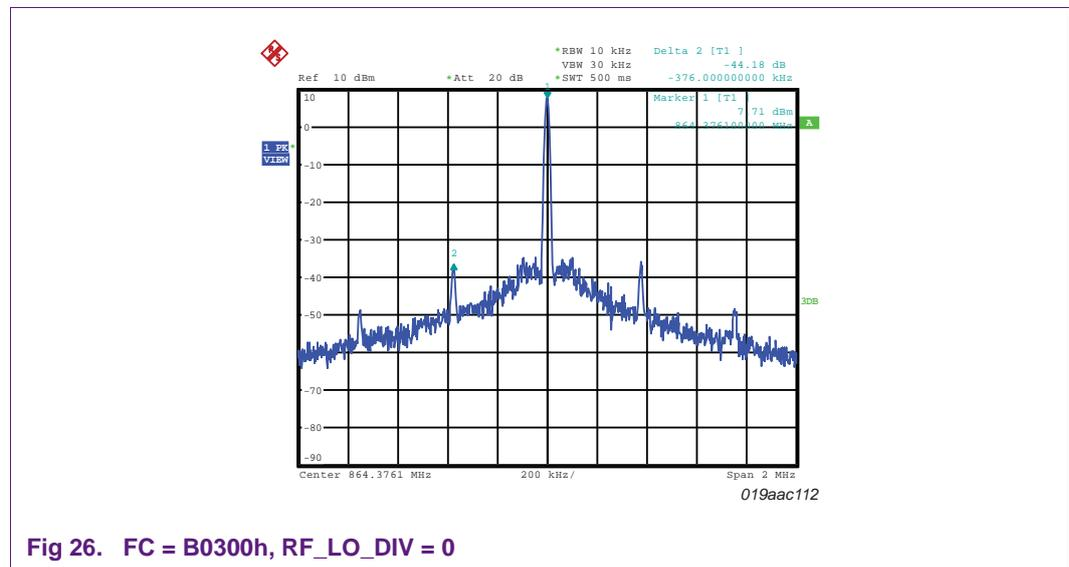
The influence of flag Double\_SD\_Result to the spurious emission is small. If the flag is set, the output signal will show an increased phase noise. Avoid configuring the OL2381 to FSK in transmit mode if the flag is set.
