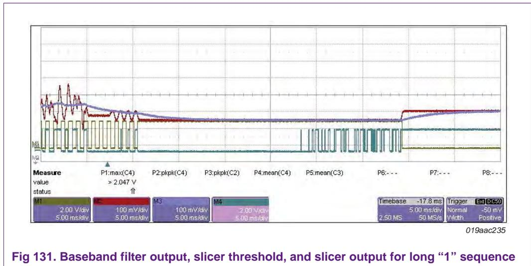
**Fig 131. Baseband filter output, slicer threshold, and slicer output for long “1” sequence**
