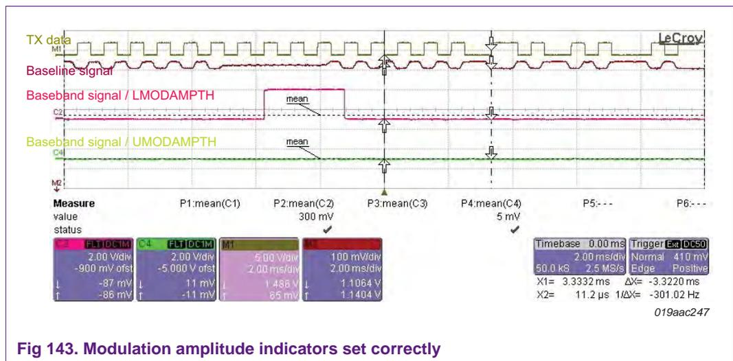
Fig 143. Modulation amplitude indicators set correctly
