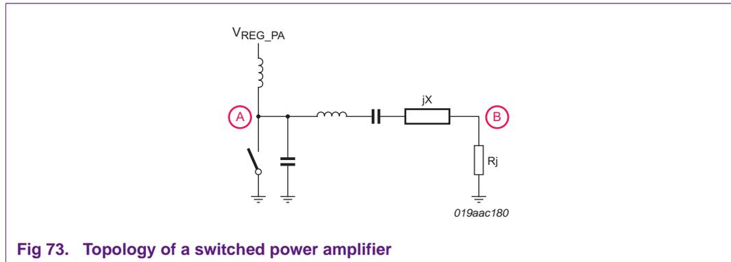
**Fig 73. Topology of a switched power amplifier**
