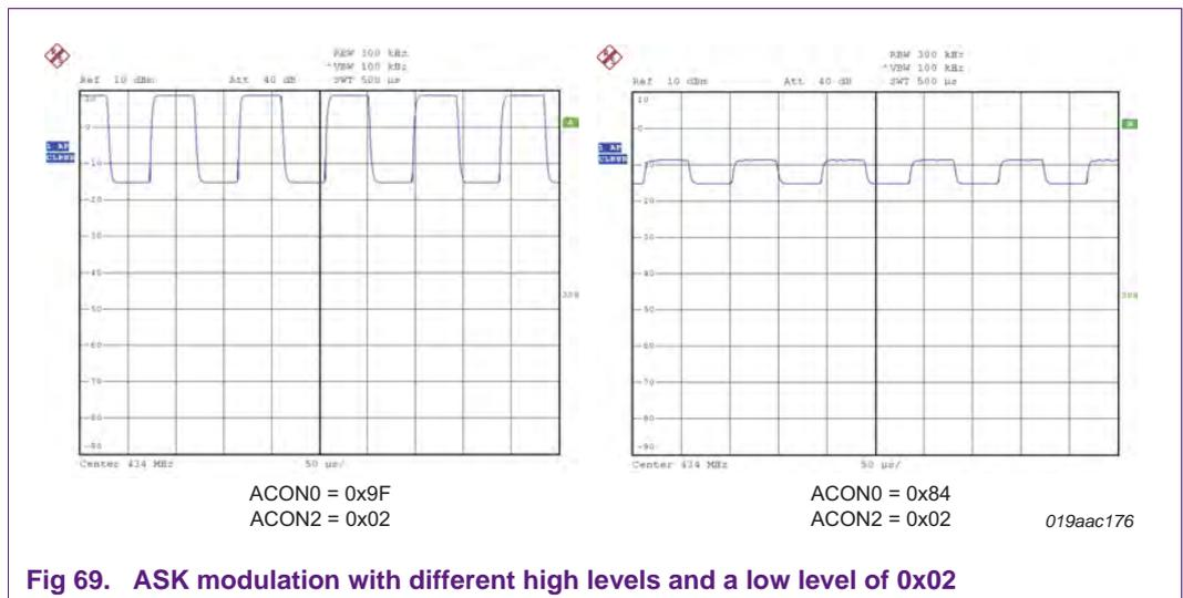
It is possible to modify ASK modulation baud rate by modifying registers TIMING0 and TIMING1 as shown in [Figure 31 on page 31](#). All previous display examples for ASK modulation were created with a baud rate of 9.6 kbit/s. Therefore register TIMING0 is set to 0xD5 and register TIMING1 is set to 0x59.
