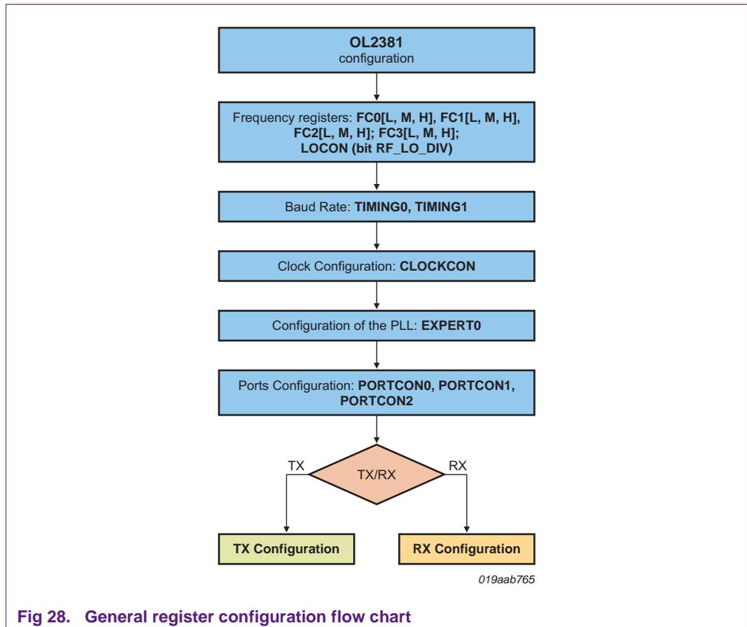
Fig 28. General register configuration flow chart
