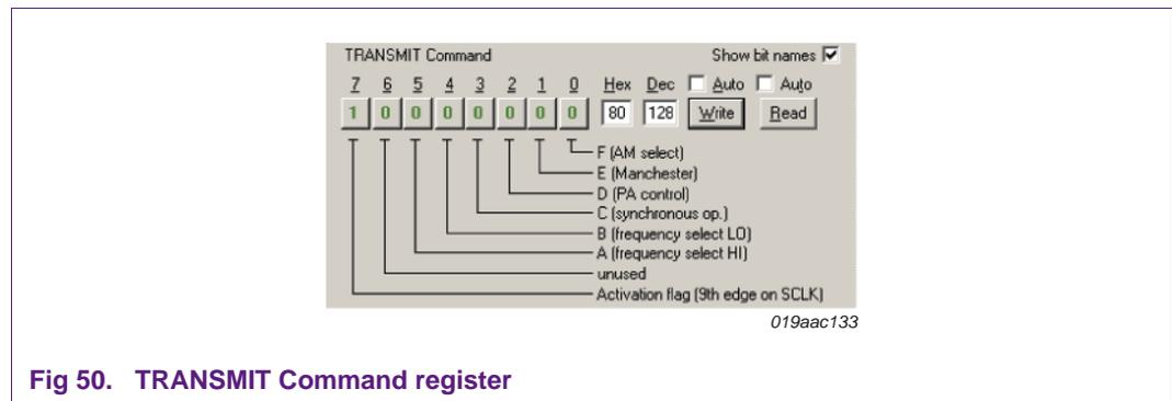
**Fig 50. TRANSMIT Command register**
