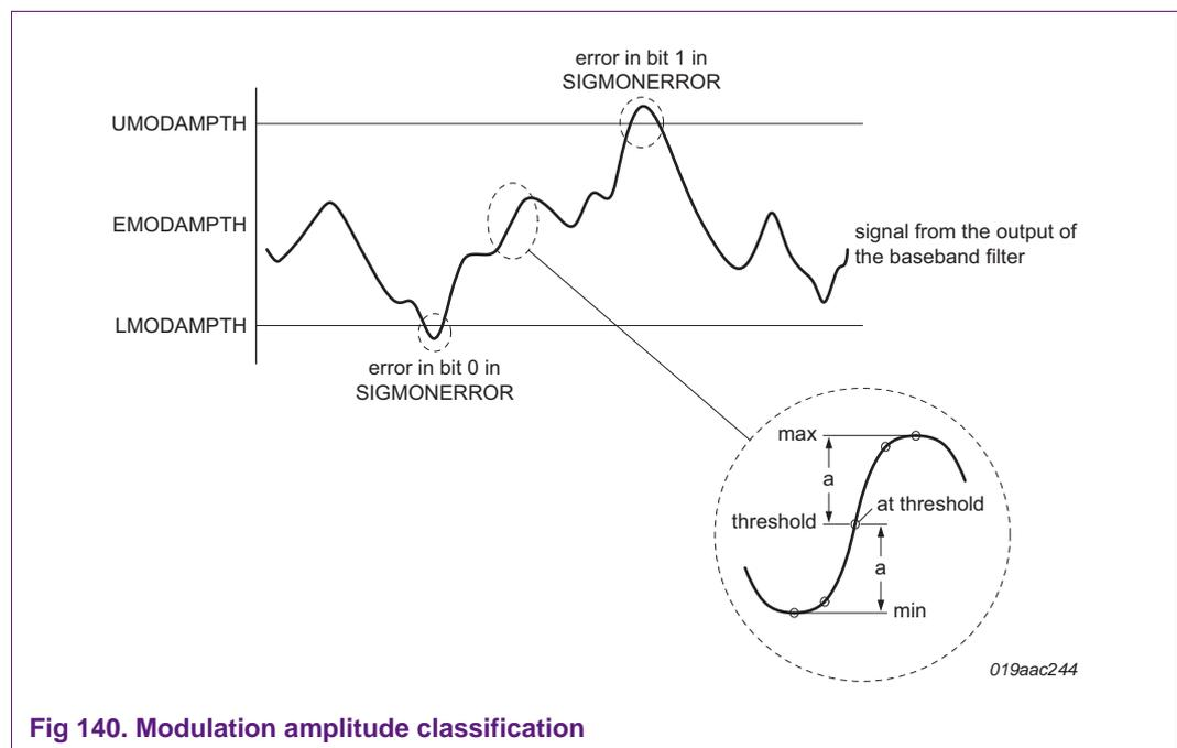
Fig 140. Modulation amplitude classification
