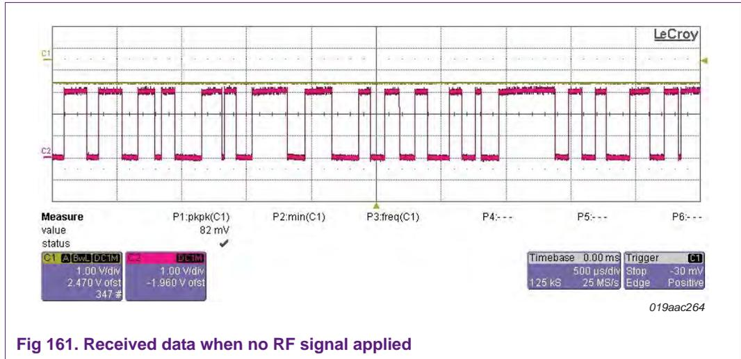
Fig 161. Received data when no RF signal applied
