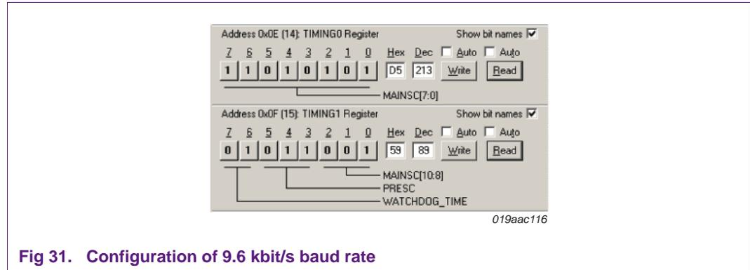
**Fig 31. Configuration of 9.6 kbit/s baud rate**
