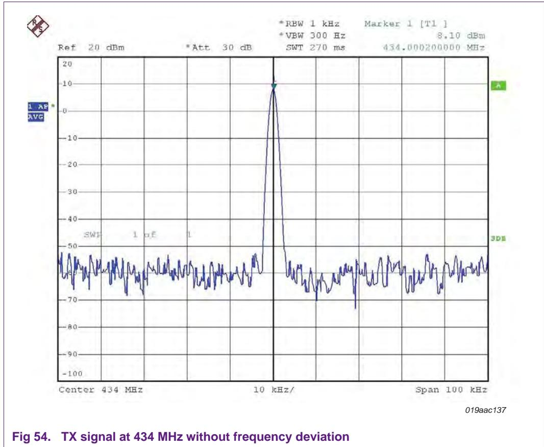
Fig 54. TX signal at 434 MHz without frequency deviation
