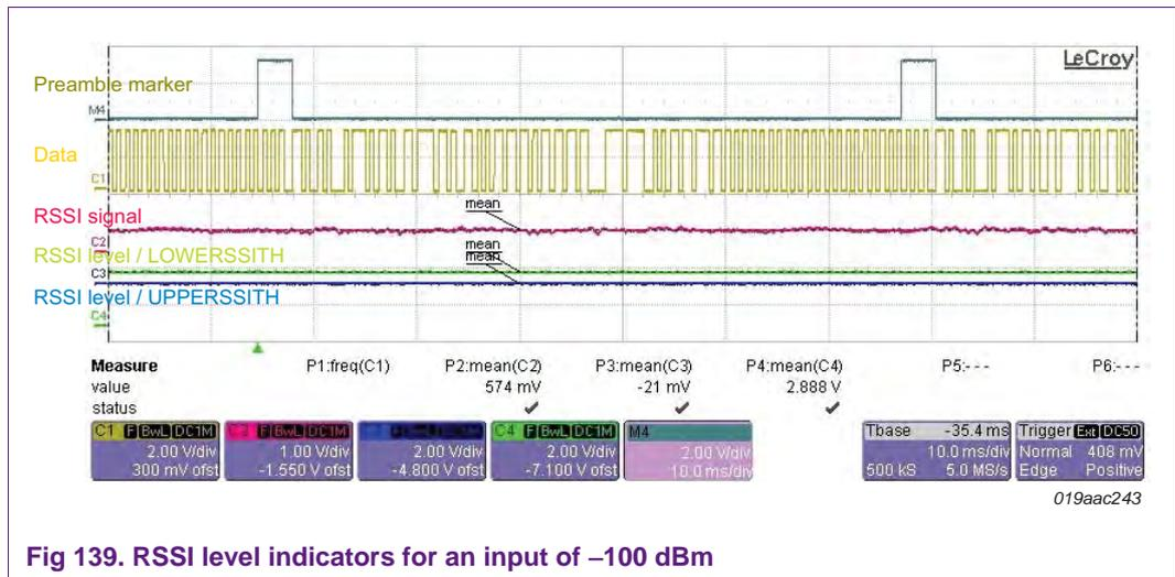
Fig 139. RSSI level indicators for an input of -100 dBm
