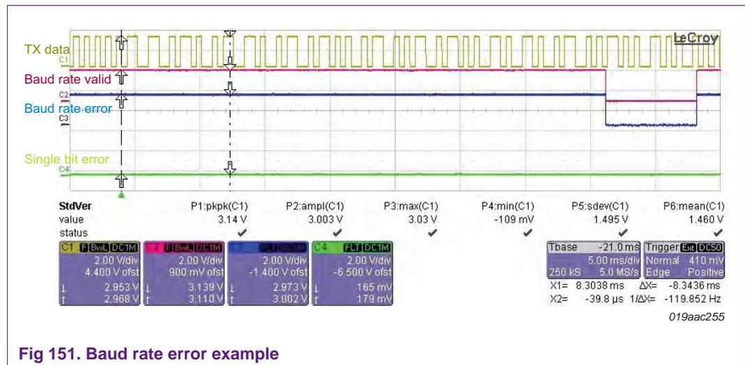
Fig 151. Baud rate error example
