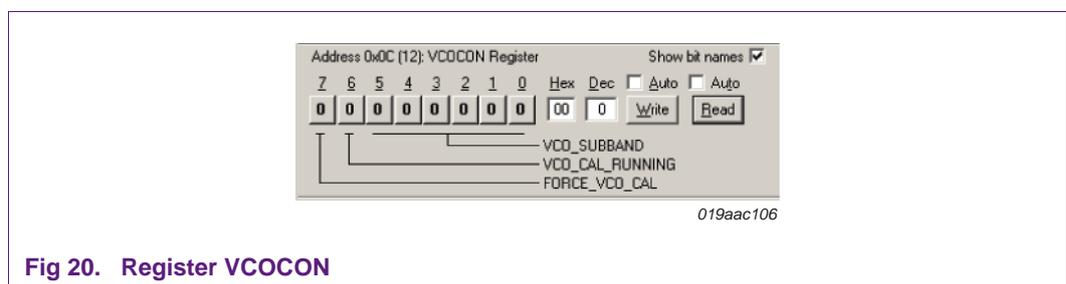
**Fig 20. Register VCOCON**
