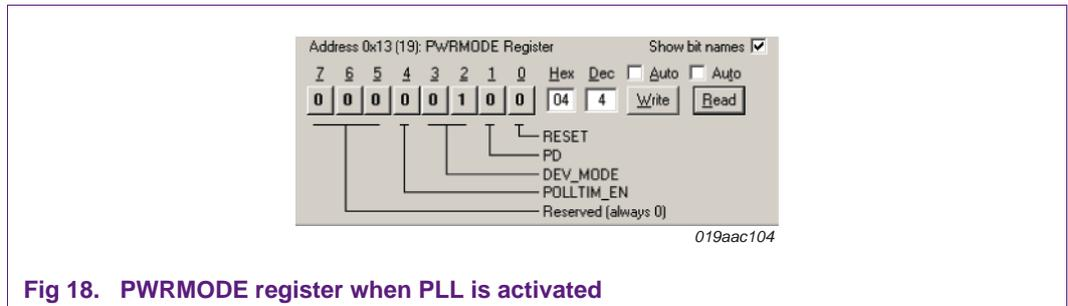
Fig 18. PWRMODE register when PLL is activated
