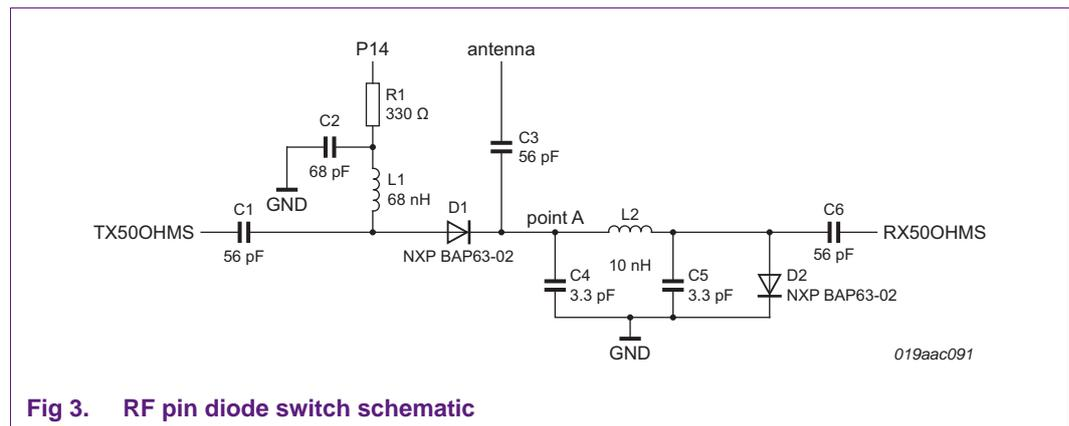
Fig 3. RF pin diode switch schematic
