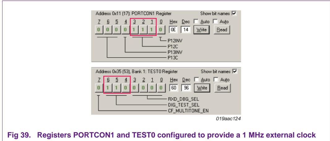
Fig 39. Registers PORTCON1 and TEST0 configured to provide a 1 MHz external clock
