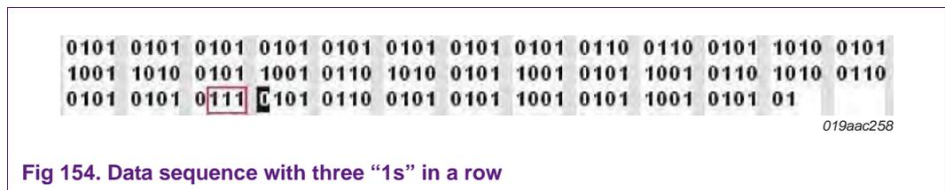
**Fig 154. Data sequence with three “1s” in a row**
