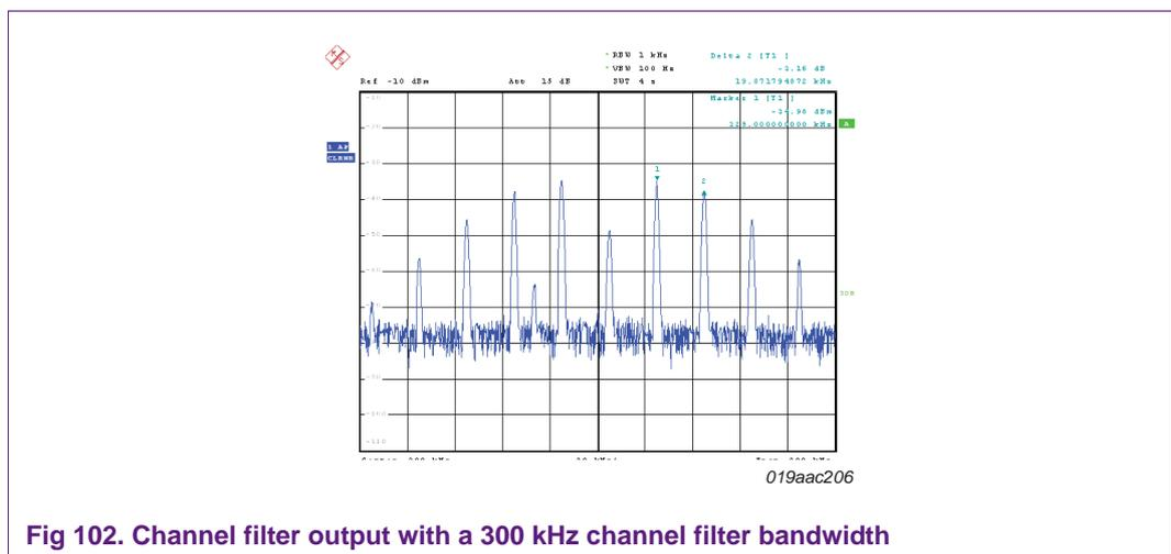
Fig 102. Channel filter output with a 300 kHz channel filter bandwidth
