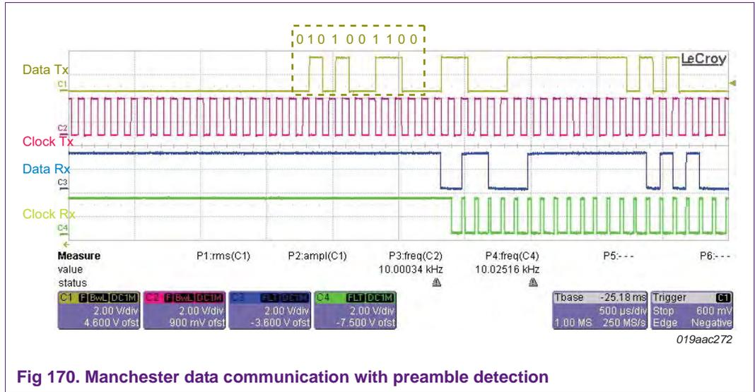
Fig 170. Manchester data communication with preamble detection
