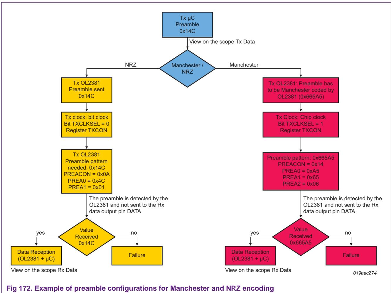
Fig 172. Example of preamble configurations for Manchester and NRZ encoding
