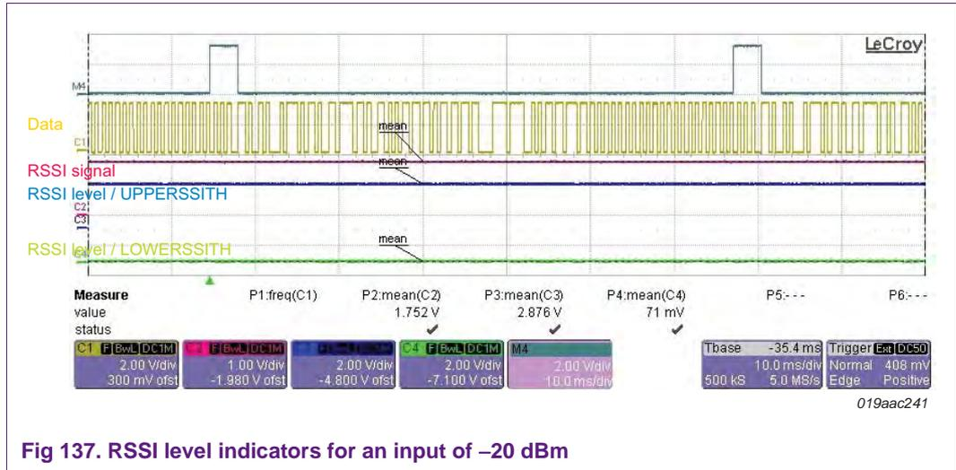
Fig 137. RSSI level indicators for an input of -20 dBm
