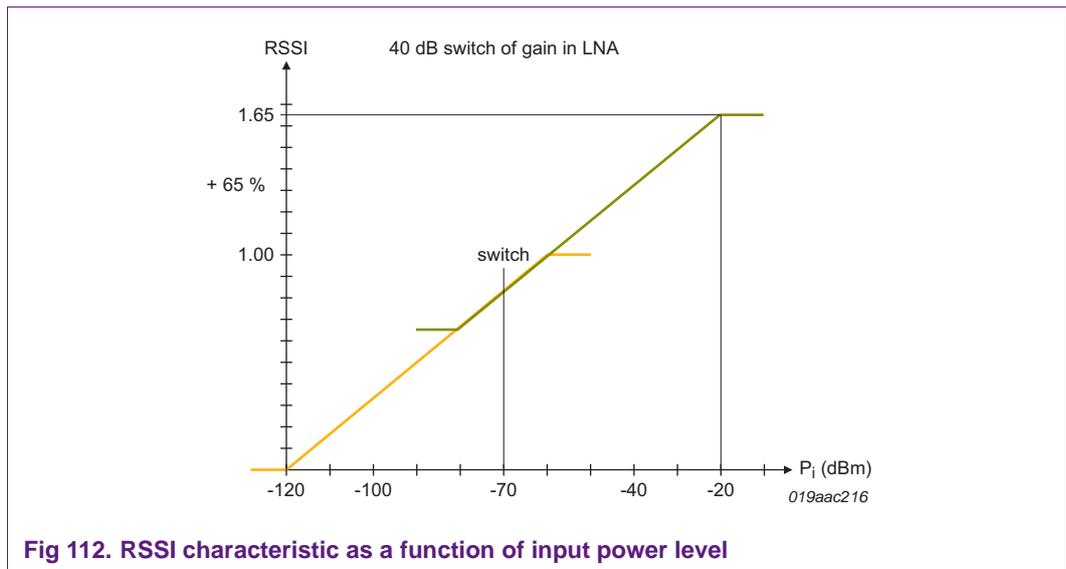
Fig 112. RSSI characteristic as a function of input power level
