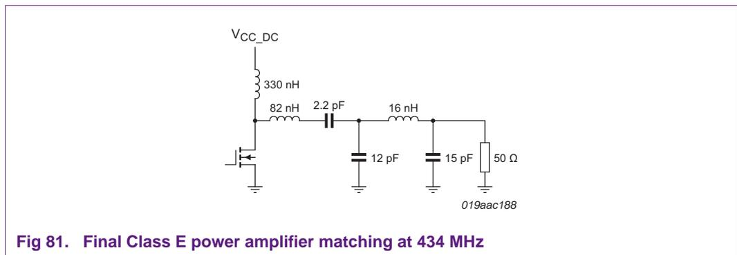
Fig 81. Final Class E power amplifier matching at 434 MHz
