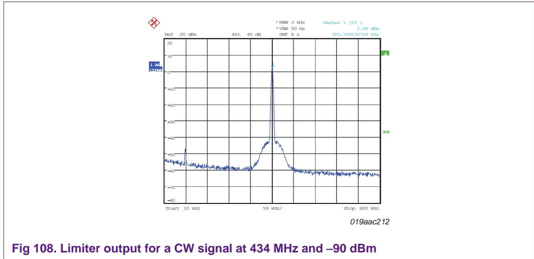
Fig 108. Limiter output for a CW signal at 434 MHz and -90 dBm
