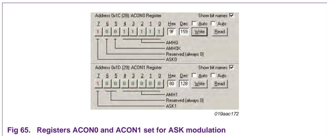
Fig 65. Registers ACON0 and ACON1 set for ASK modulation
