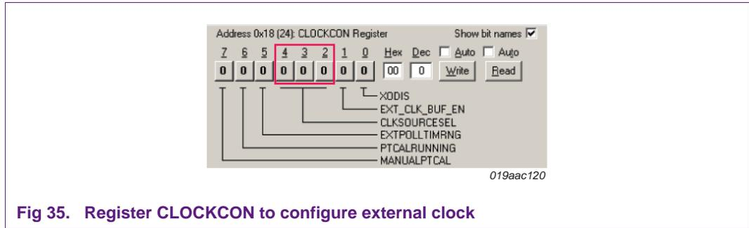
Fig 35. Register CLOCKCON to configure external clock
