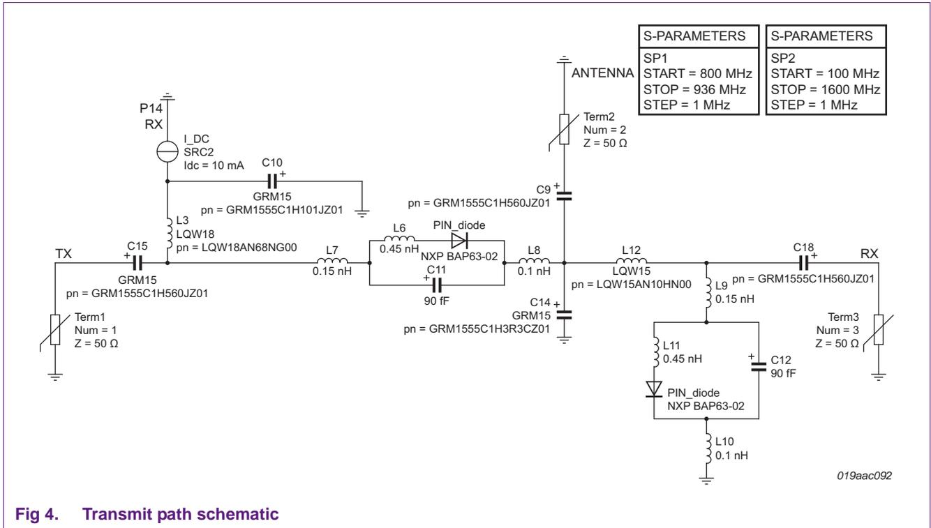
Fig 4. Transmit path schematic
