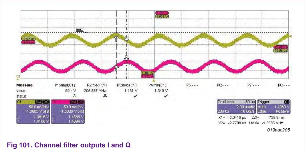
Fig 101. Channel filter outputs I and Q
