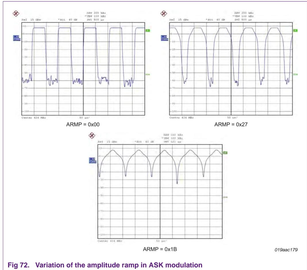
**Fig 72. Variation of the amplitude ramp in ASK modulation**
