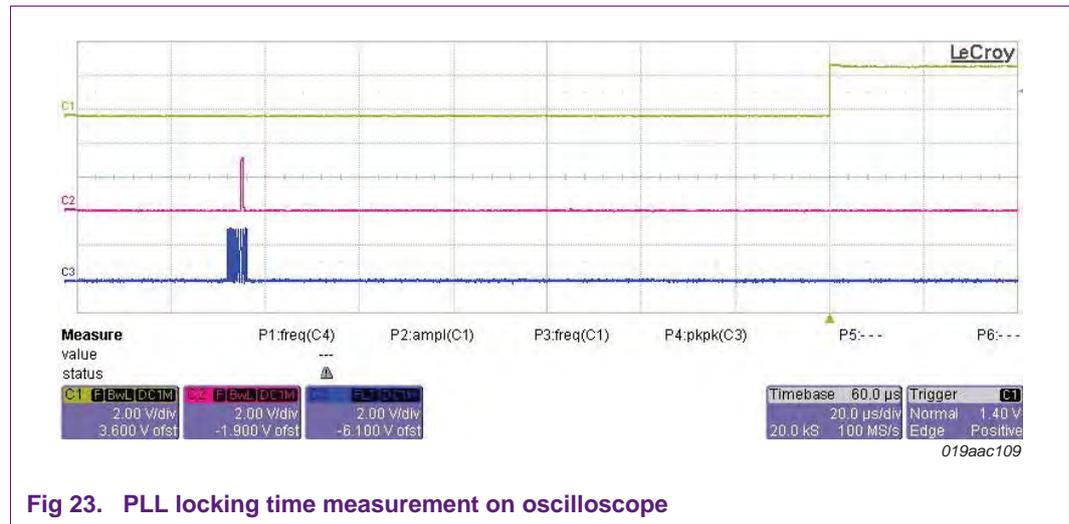
Fig 23. PLL locking time measurement on oscilloscope
