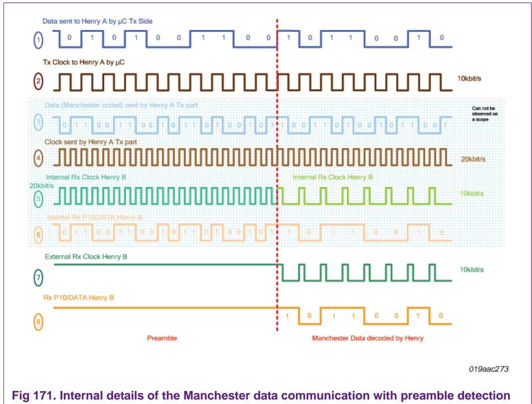
Fig 171. Internal details of the Manchester data communication with preamble detection
