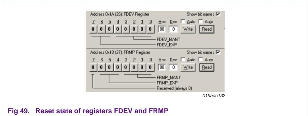
**Fig 49. Reset state of registers FDEV and FRMP**
