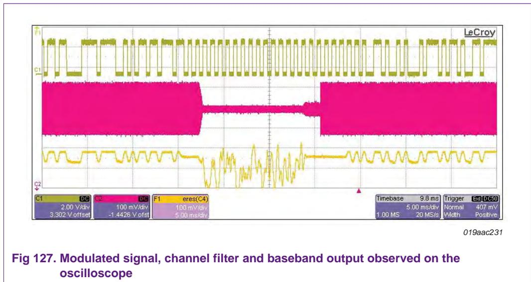
Fig 127. Modulated signal, channel filter and baseband output observed on the oscilloscope
