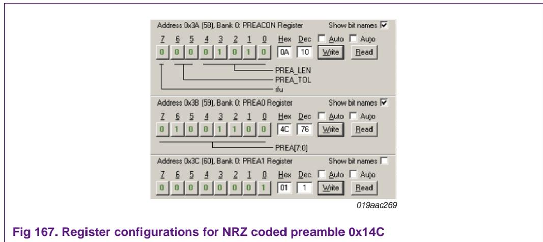
Fig 167. Register configurations for NRZ coded preamble 0x14C
