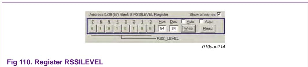
Fig 110. Register RSSILEVEL
