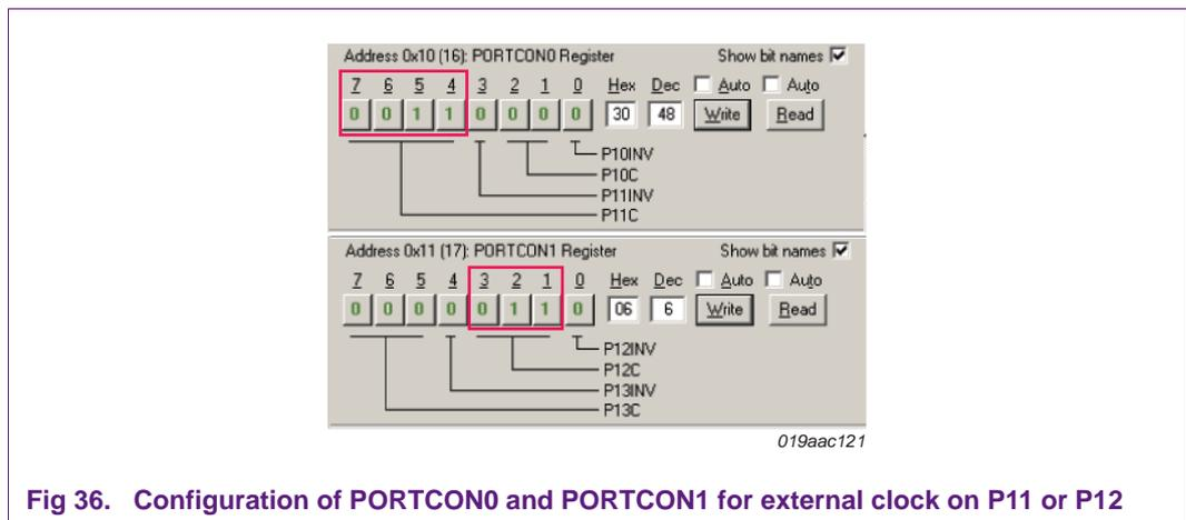
Fig 36. Configuration of PORTCON0 and PORTCON1 for external clock on P11 or P12
