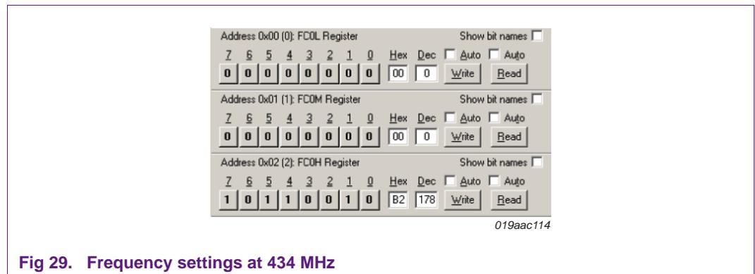
Fig 29. Frequency settings at 434 MHz
