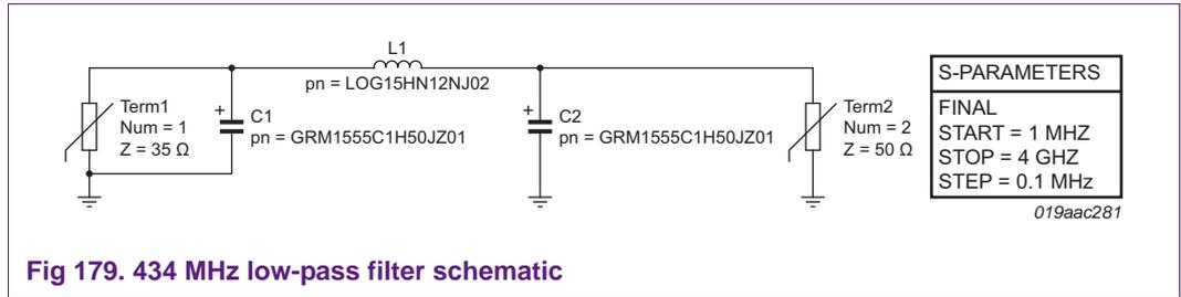
Fig 179. 434 MHz low-pass filter schematic
