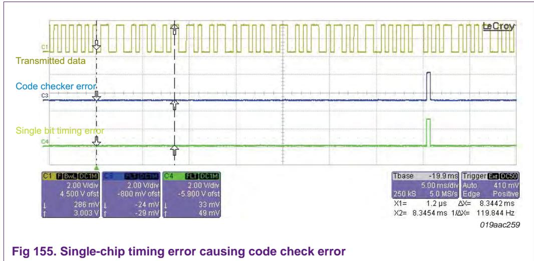
Fig 155. Single-chip timing error causing code check error
