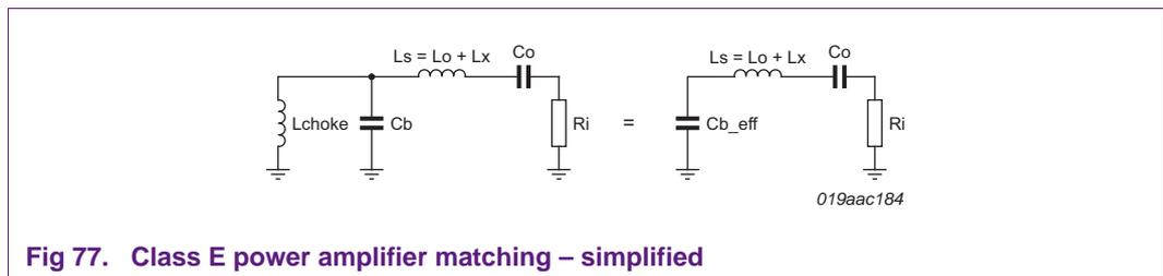
Fig 77. Class E power amplifier matching – simplified
