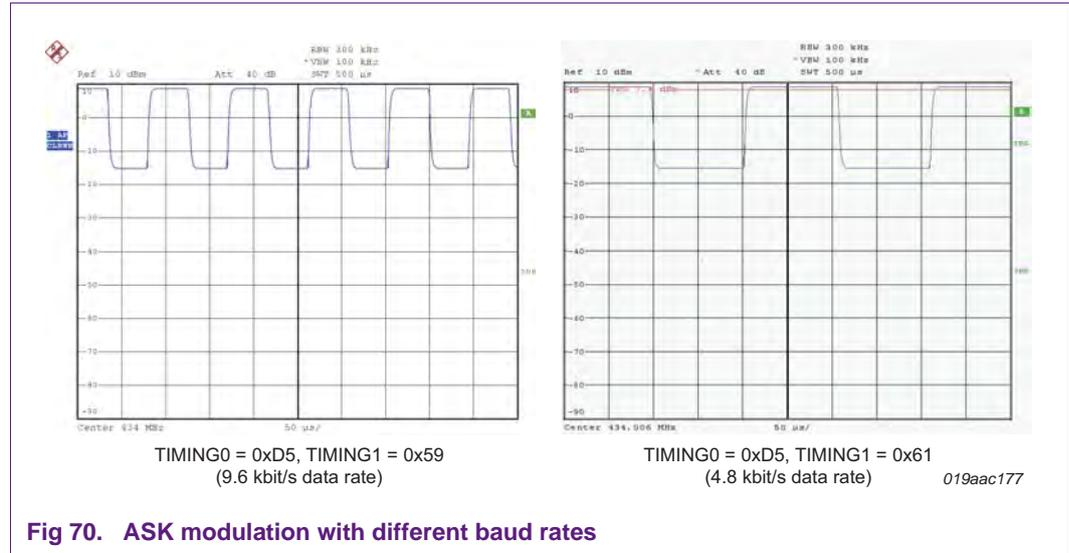
Fig 70. ASK modulation with different baud rates
