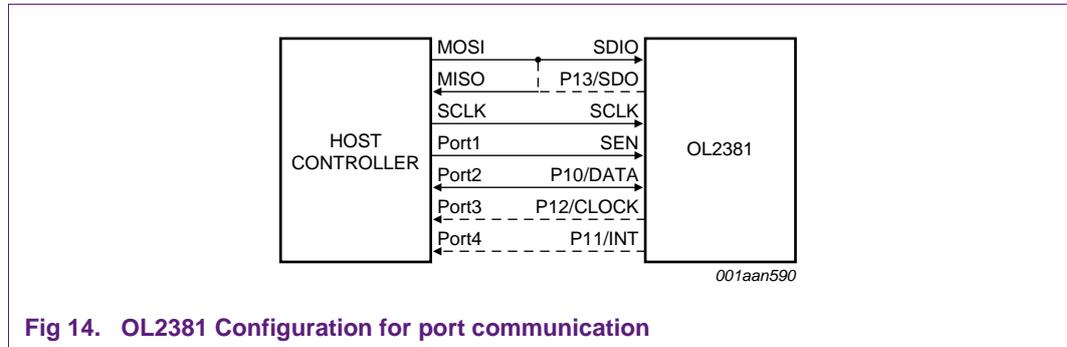
Pin P10/DATA is used for TX/RX data input/output, P12/CLOCK delivers the associated clock signal and P11/INT can be configured for data or interrupt output between the OL2381 and host controller.
