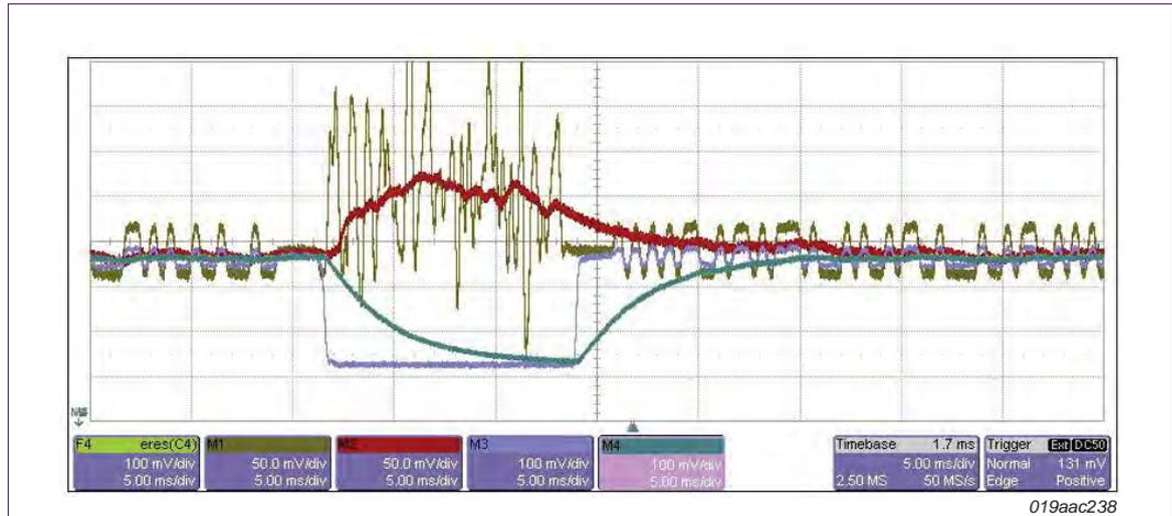
Fig 134. Baseband filter output and slicer threshold: interferer with 1 dB less power present
