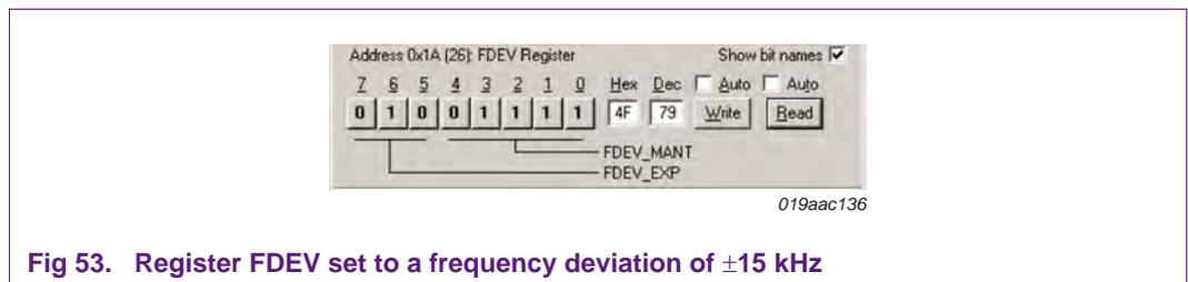
Fig 53. Register FDEV set to a frequency deviation of ±15 kHz
