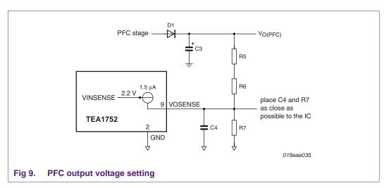
Two resistors of 4.7 M $\Omega$  (1 %) can be used between the bulk elcap and the VOSENSE pin. The dimensioning of the I<sub>bst(dual)</sub> current source (–15  $\mu$ A) has been adapted to the use of these resistor values. With a resistor value of 4.7 M $\Omega$  for R5 and R6 and 60 k $\Omega$  to 62 k $\Omega$  for R7 a universal mains adapter has a PFC output voltage of approximately 380 V to 390 V at high mains and 240 V to 250 V at low mains.
