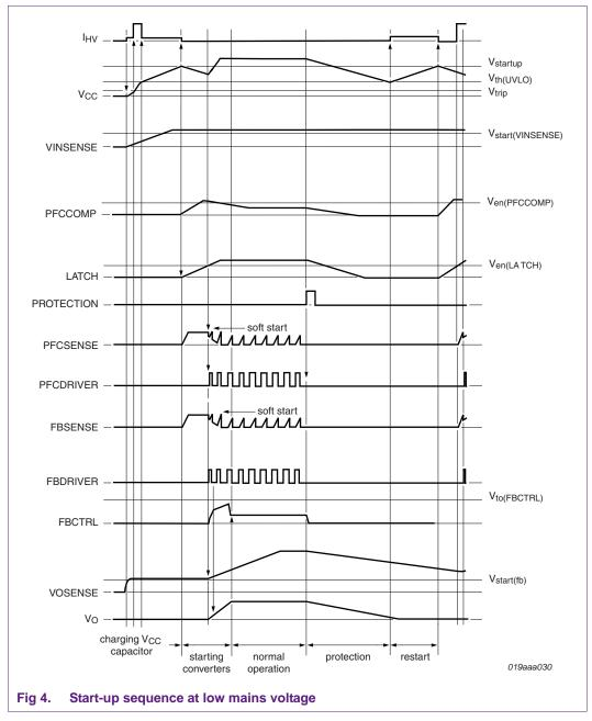
The charge time of the soft start capacitors can be chosen independently for the PFC and the flyback, based on their values.
