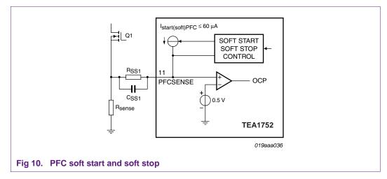
The total soft start or soft stop time is:  $t_{softstart} = 3 \times R_{SSI} \times C_{SSI}$
