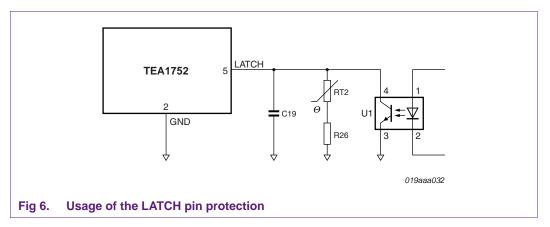
Latching on application overtemperature occurs when the total resistance value of the NTC and its series resistor drops below the following:
