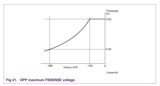
The total OPP resistance determining the I<sub>FBAUX</sub> current during the primary stroke of the flyback exists of R23 + R23A (see <u>Figure 20</u>). The OVP resistor R23 has to be calculated before the remaining part of the OPP resistor R23A can be calculated.
