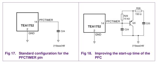
The delay time of the PFC (described in Section 5.2) is no longer determined by the value of C24 in Figure 18, but by C25. The value of capacitor C24 has to be very small, typically 1 nF. The start-up time of the PFC can be neglected. It is recommended to use a transistor with a large DC current gain (=  $h_{FE}$ ).
