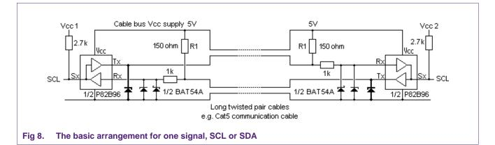
P82B96 is used in its conventional way to split the bidirectional I<sup>2</sup>C-bus signal into two unidirectional components Tx and Rx. Tx is the logic signal to be transmitted over the cable to a remote node and Rx is the logic signal received from that remote node.
