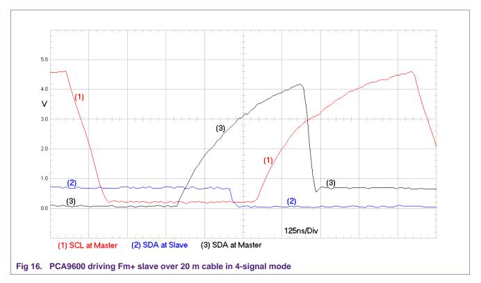
Figure 16 shows a 1 MHz clock (1) as generated at the master. The Acknowledge by a PCA9633 slave (measured at the slave SDA pin) is shown (2) and the SDA waveform as measured at the master SDA pin is shown as (3).
