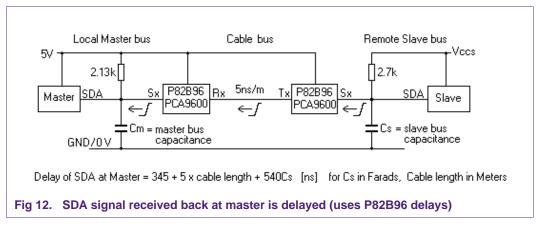
Figure 11 and Figure 12 show those two delays and how they may be approximated when the buffer used is P82B96.
