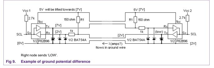
Figure 9 shows one example of the situation that must be handled when the ground potential at each end of the cable is different.
