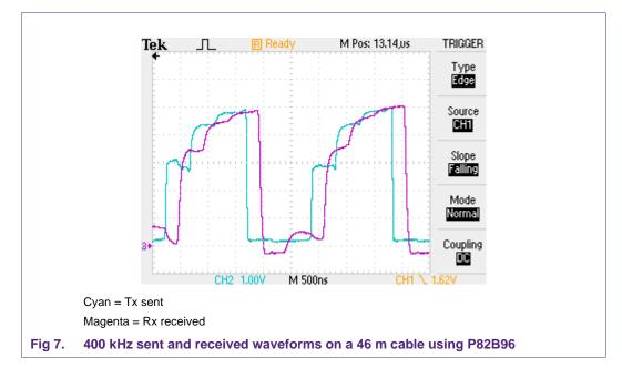
Typical waveforms on a 46 m cable are shown in <u>Figure 7</u>. The cyan trace shows the 'send' signal generated at Tx. It is pulled LOW to approximately 0.2 V by the strong sink capability of Tx even though the 'dynamic' load is the 100  $\Omega$  cable characteristic impedance.
