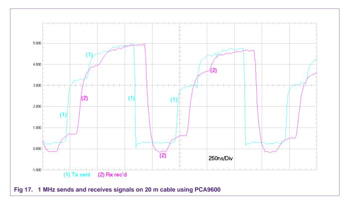
Figure 17 shows the PCA9600 cable waveforms for comparison with P82B96 shown in Figure 7 in Section 3.2.
