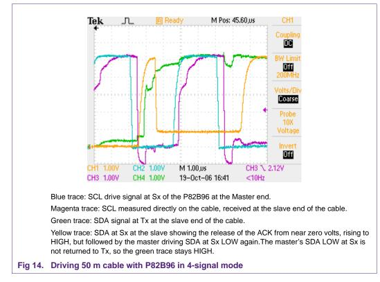
Points to note include the reasonably controlled overshoot of the falling edge of SCL at the far end of the cable to about -1 V which would still exceed the rating of Rx if the series 1 k $\Omega$  and shunt Schottky diode had not been used. The effects of cross-coupling of the 4 signals and the voltage drop on the cable resistance also results in some distortions of
