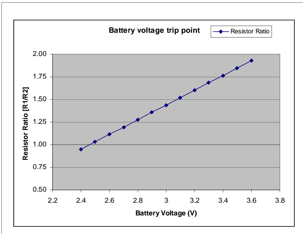
Fig 2. Battery trip points resistor ratio
