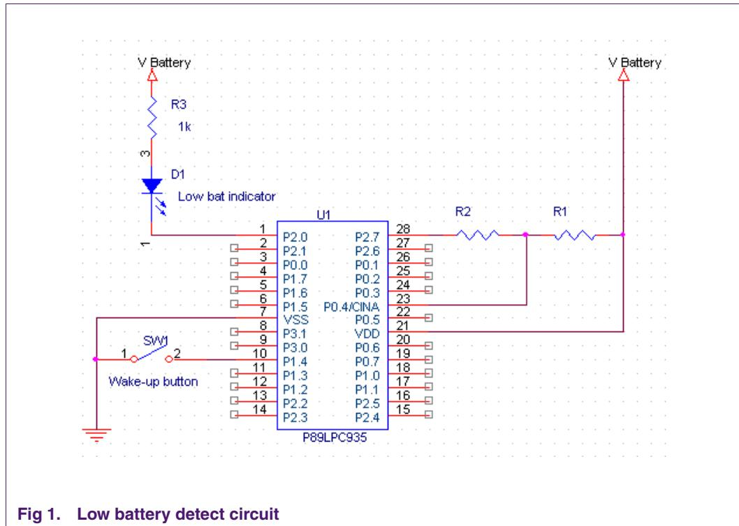
R1 and R2 are a resistor divider that is fed into the comparator input, as the battery voltage drops the voltage into the comparator drops. Since the comparator has a stable internal reference voltage a ratio of R1 and R2 can be chosen to trip the comparator at a specific battery voltage.
