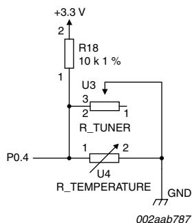
Fig 2. Temperature sensing circuit
