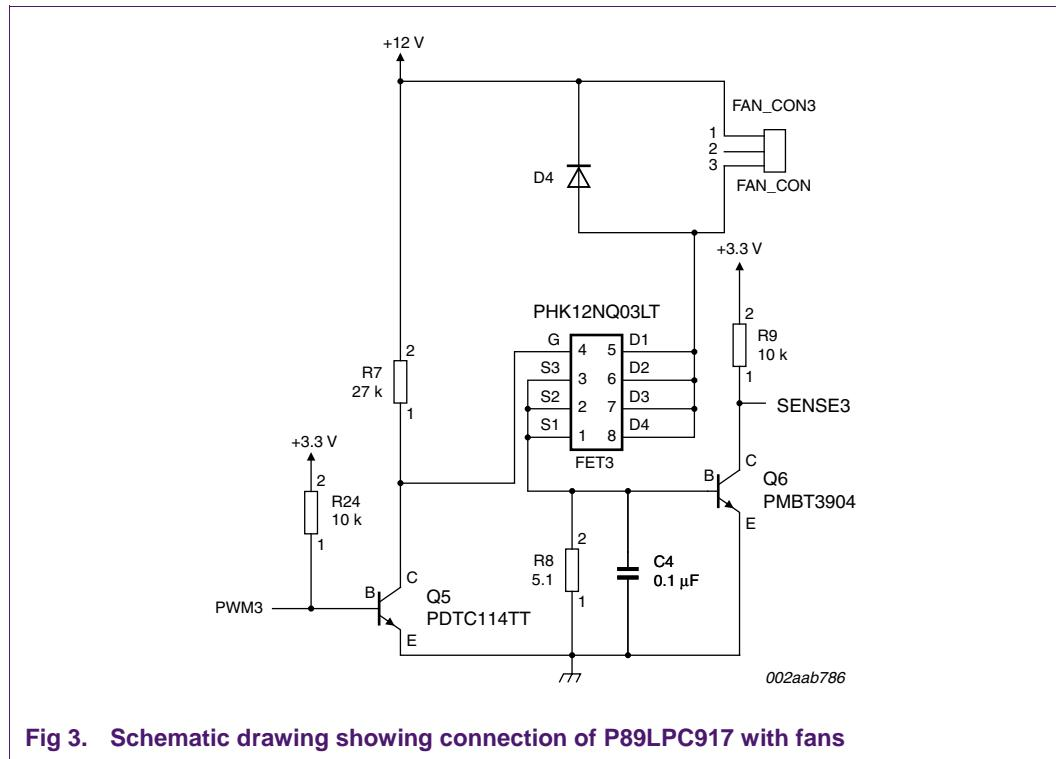
Fig 3. Schematic drawing showing connection of P89LPC917 with fans
