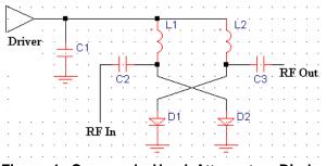
Figure 1. Commonly Used Attenuator. Diodes are BAP50-05.
