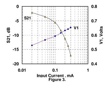
If the diodes are driven from a voltage source (not shown), the speed is very fast, but the attenuation is highly nonlinear and is highly temperature dependent.
