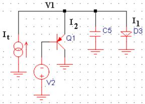
Figure 4. Transistor Shunt. V2 is < 200 mV.
