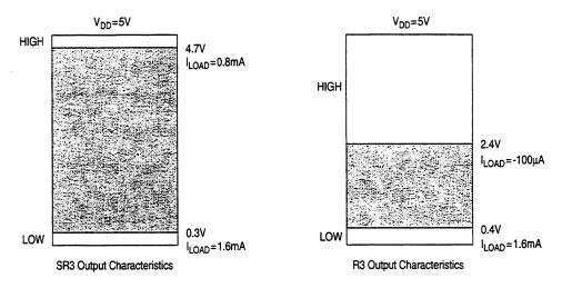
The input level also has better noise margin. However, the input HIGH voltage is 0.7V<sub>DD</sub> and this is 3.5V for a 5V supply. The minimum value of output HIGH for TTL logic is about 2.7V, therefore pull-ups are required for TTL outputs to drive SR3 inputs.
