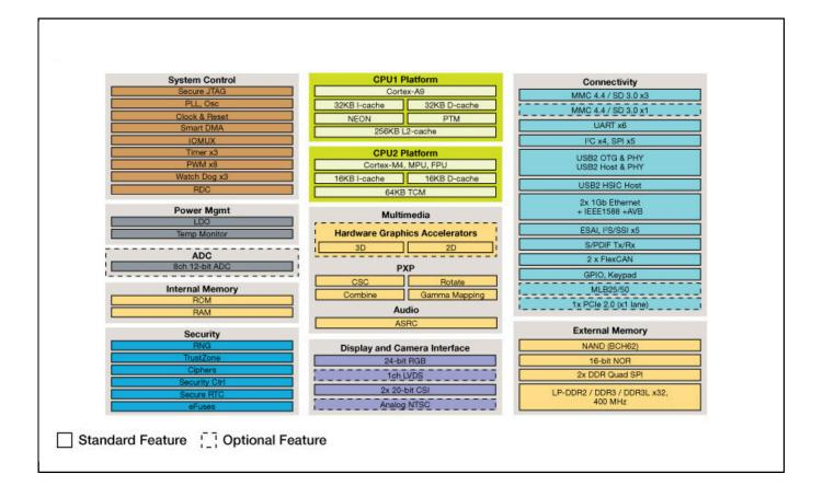
View additional information for i.MX 6SoloX Processors - Heterogeneous Processing with Arm® Cortex®-A9 and Cortex-M4 Cores.
