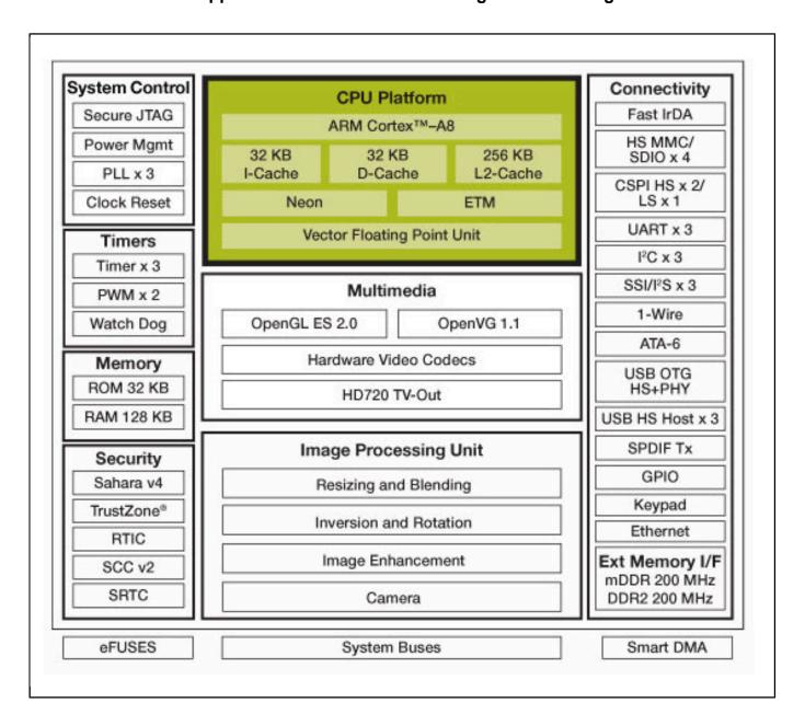
View additional information for Applications Processors - Advanced HMI, High-Performance, Low-Power, Arm® Cortex®-A8 Core.
